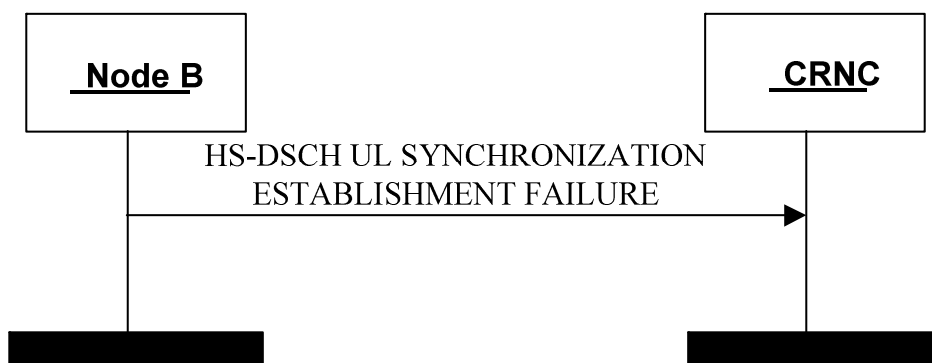
Figure 12D: HS-DSCH UL Synchronization Establishment Failure procedure
