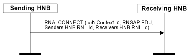
Figure 7.3.2.2.1-1: Signalling Connection Establishment – Direct Iurh-connectivity.
