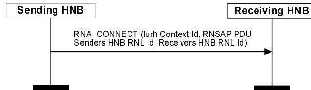
Figure 7.3.2.2.1-1: Signalling Connection Establishment – Direct Iurh-connectivity.
