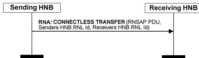
Figure 7.3.2.5.1-1: Connectionless data transfer – Direct Iurh-connectivity.
