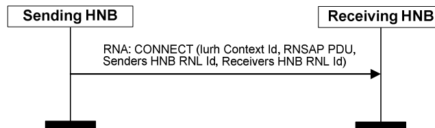
Figure 7.3.2.2.1-1: Signalling Connection Establishment – Direct Iurh-connectivity.
