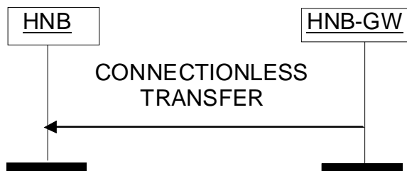
Figure 6: Connectionless Transfer to HNB
