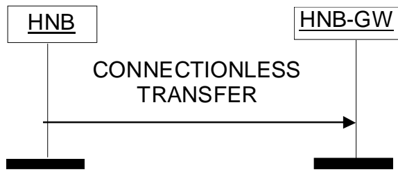
Figure 7: Connectionless Transfer to HNB-GW
