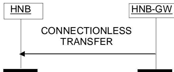
Figure 6: Connectionless Transfer to HNB
