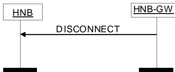
Figure 5: Disconnect to HNB
