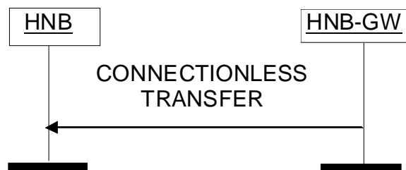
Figure 6: Connectionless Transfer to HNB
