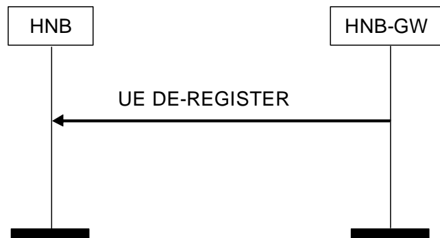
Figure 8 UE De-Register Procedure: HNB-GW Originated Successful Operation
