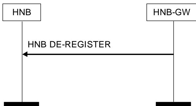
Figure 4: HNB De-register Procedure: Successful Operation
