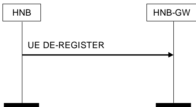
Figure 7 UE De-Register Procedure: HNB Originated Successful Operation
