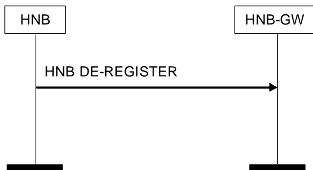
Figure 3: HNB De-register Procedure: Successful Operation
