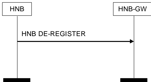
Figure 3: HNB De-register Procedure: Successful Operation
