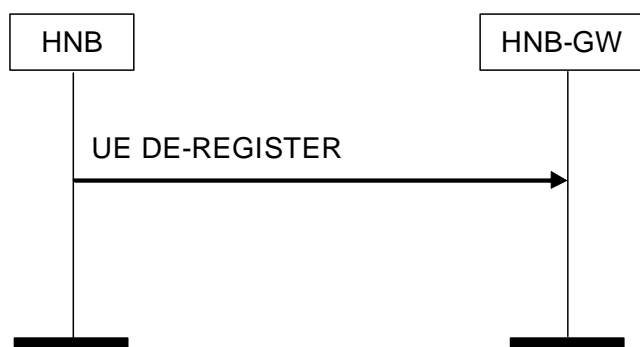
Figure 7 UE De-Register Procedure: HNB Originated Successful Operation
