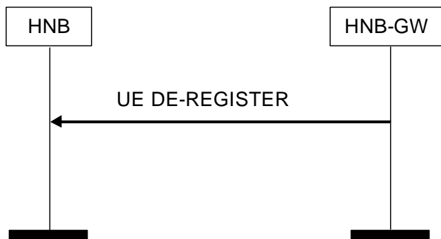
Figure 8 UE De-Register Procedure: HNB-GW Originated Successful Operation
