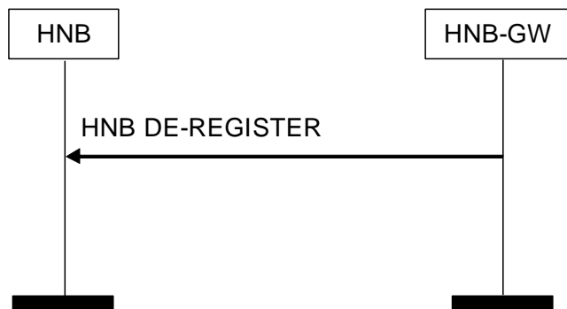
Figure 4: HNB De-register Procedure: Successful Operation
