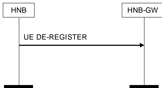
Figure 7 UE De-Register Procedure: HNB Originated Successful Operation
