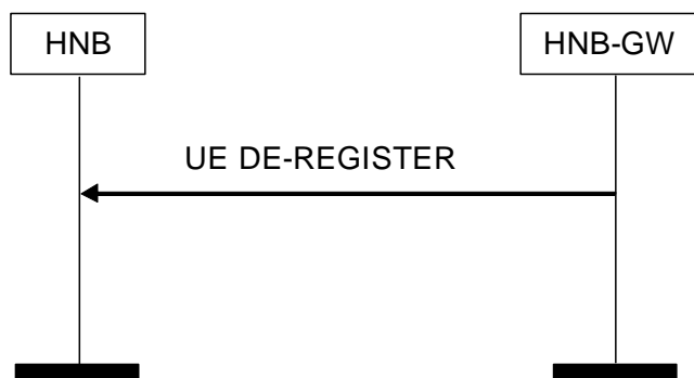
Figure 8 UE De-Register Procedure: HNB-GW Originated Successful Operation
