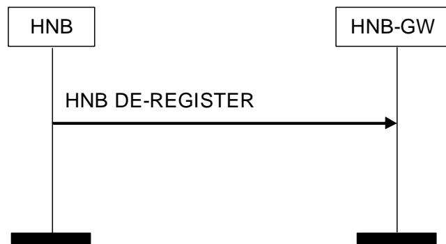
Figure 3: HNB De-register Procedure: Successful Operation
