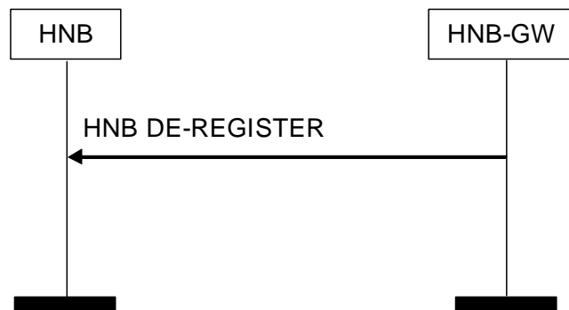
Figure 4: HNB De-register Procedure: Successful Operation
