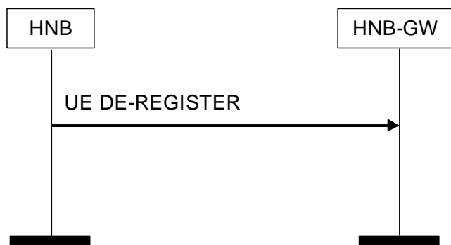
Figure 7 UE De-Register Procedure: HNB Originated Successful Operation
