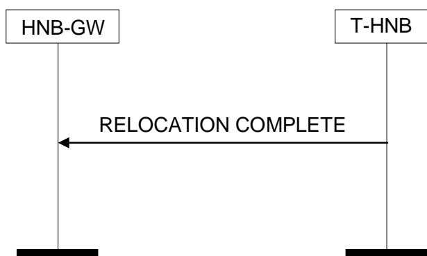
Figure 17: Relocation Complete procedure. Successful operation.
