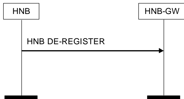
Figure 3: HNB De-register Procedure: Successful Operation
