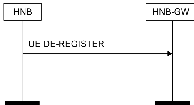
Figure 8.5.2-1: UE De-Register Procedure: HNB Originated Successful Operation
