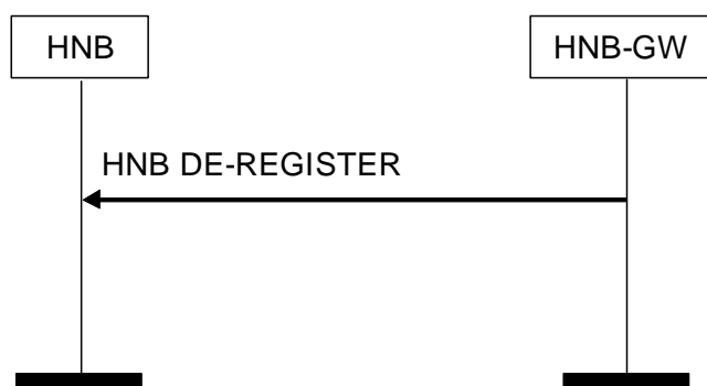
Figure 8.3.2-1: HNB De-register Procedure: Successful Operation
