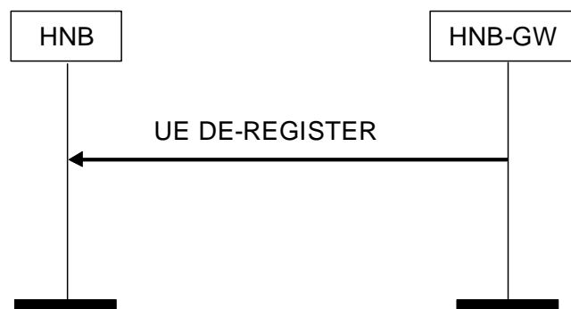
Figure 8.5.3-1: UE De-Register Procedure: HNB-GW Originated Successful Operation
