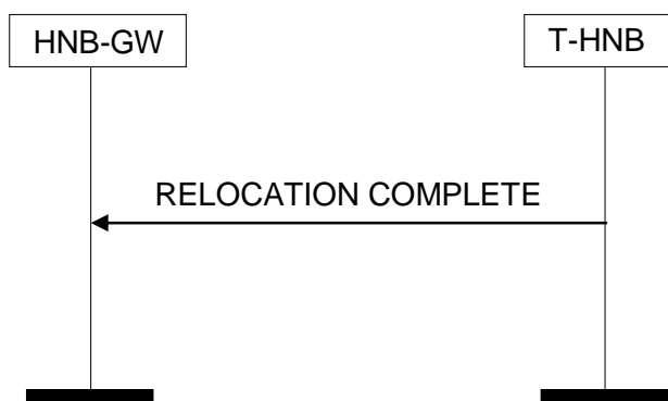
Figure 8.11.2-1: Relocation Complete procedure. Successful operation.
