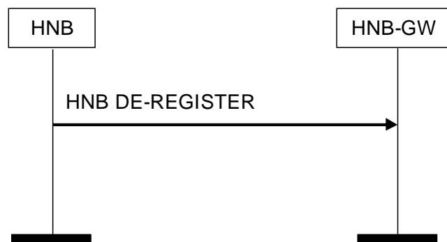
Figure 8.3.1-1: HNB De-register Procedure: Successful Operation
