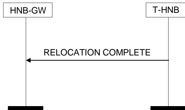
Figure 8.11.2-1: Relocation Complete procedure. Successful operation.
