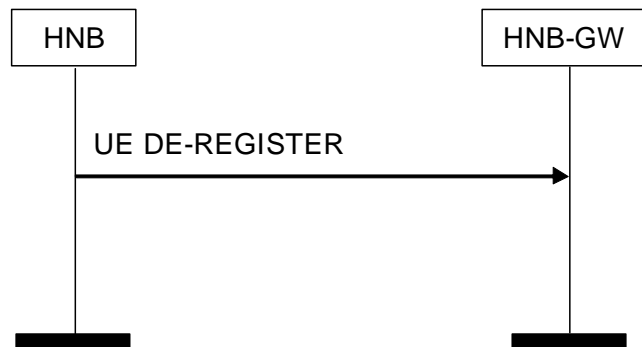
Figure 8.5.2-1: UE De-Register Procedure: HNB Originated Successful Operation
