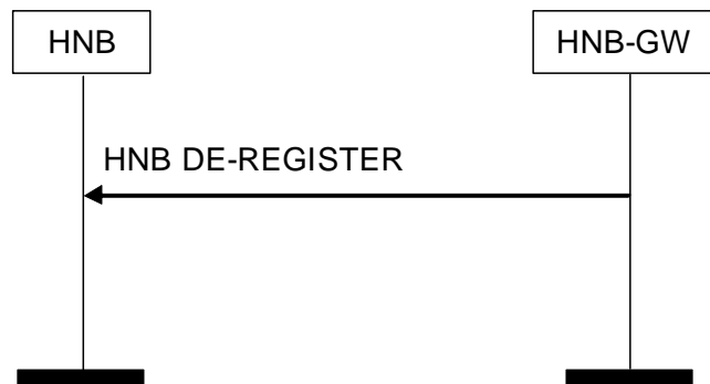
Figure 8.3.2-1: HNB De-register Procedure: Successful Operation
