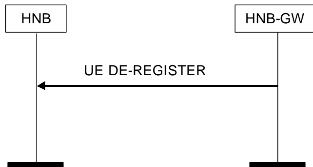
Figure 8.5.3-1: UE De-Register Procedure: HNB-GW Originated Successful Operation
