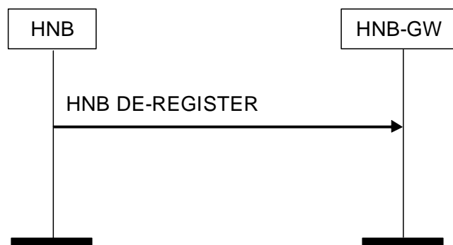
Figure 8.3.1-1: HNB De-register Procedure: Successful Operation
