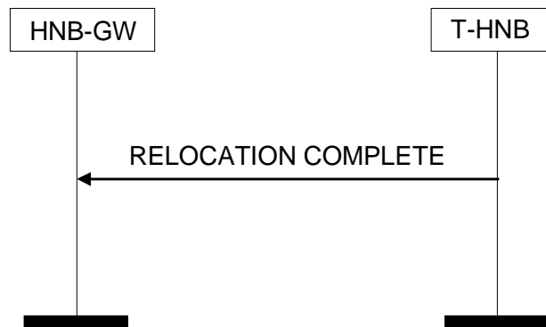
Figure 8.11.2-1: Relocation Complete procedure. Successful operation.
