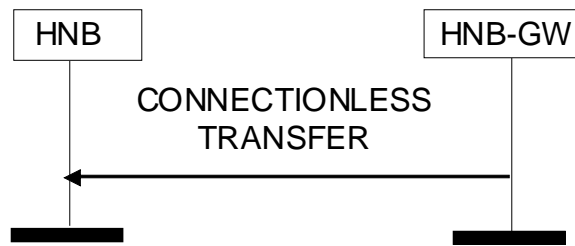
Figure 8.5.2-1: Connectionless Transfer procedure to HNB
