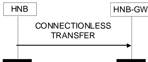
Figure 8.5.3-1: Connectionless Transfer procedure to HNB-GW
