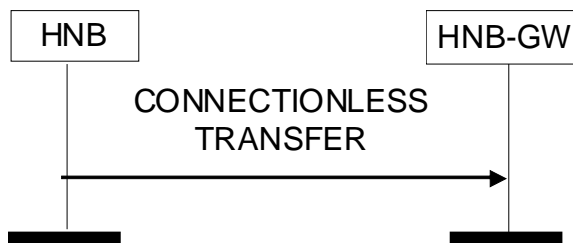
Figure 8.5.3-1: Connectionless Transfer procedure to HNB-GW
