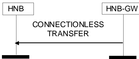
Figure 8.5.2-1: Connectionless Transfer procedure to HNB
