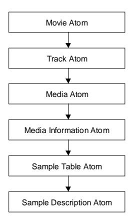
Figure D.1: MP4 Atom Structure Hierarchy
