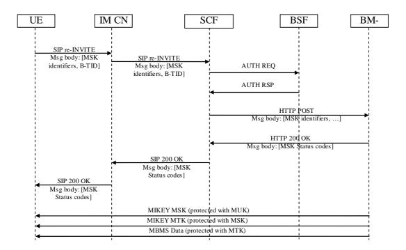
Figure 25: SIP based MBMS MSK request
