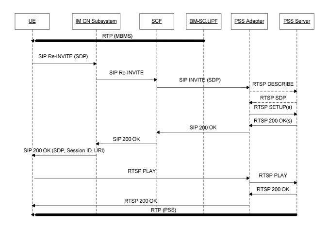
Figure 18: IMS Hybrid PSS-MBMS-to-PSS content switching
