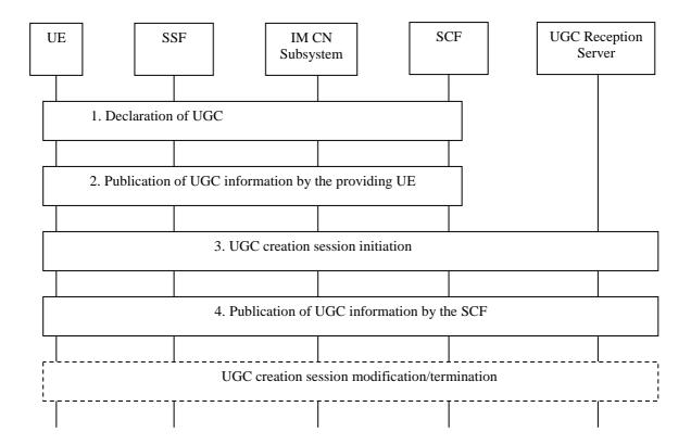
Figure 30: IMS Based UGC Provision Procedures
