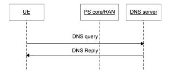
Figure 5: Service Provider Discovery with DNS
