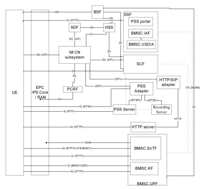
Figure 2: IMS based PSS and MBMS functional architecture
