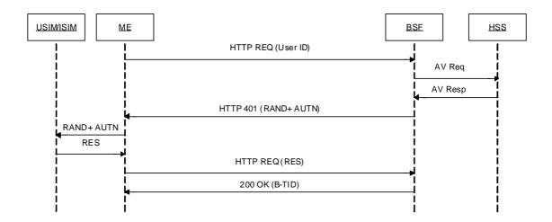
Figure 21: GBA/GAA Bootstrapping procedure
