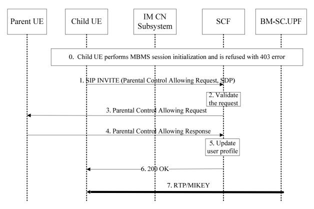
Figure 38: Interactive Parental Control Service—Allowing a MBMS user service
