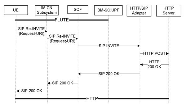
Figure 32b: IMS-based Switching from MBMS Download to PSS download
