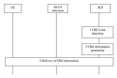
Figure 47: Procedure for CRS provided by SCF
