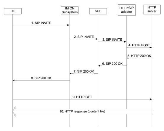
Figure 33: IMS based session set-up for progressive download
