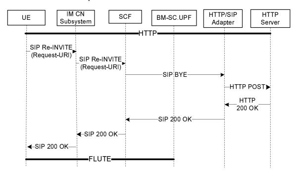
Figure 33d: IMS-based Switching from PSS Download to MBMS download
