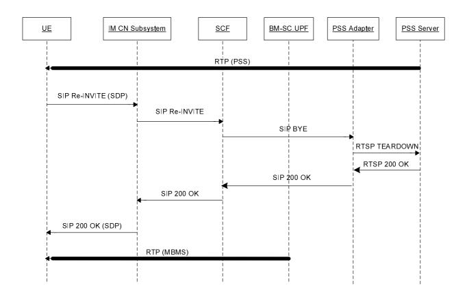
Figure 19: IMS PSS-to-MBMS content switching
