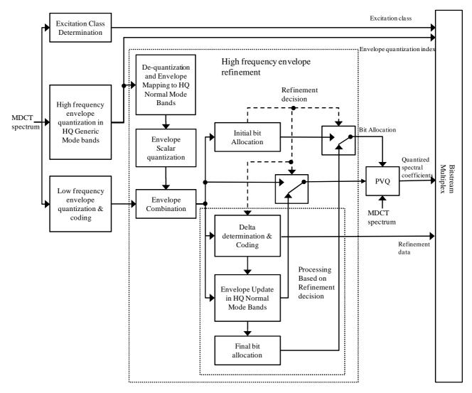
Figure 82: Generic mode Encoder Block Diagram
