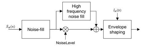
Figure 101: Spectrum filling block diagram
