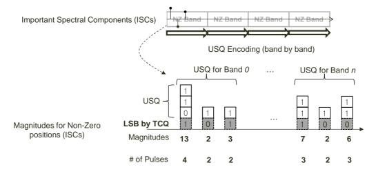
Figure 72: Concept of LSB coding
