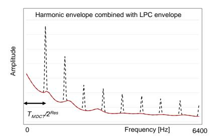
Figure 64: Example of harmonic envelope combined with LPC envelope used in envelope based arithmetic coding.
