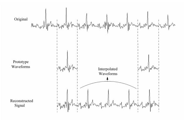
Figure 41: Illustration of principles of PPP coding [20]
