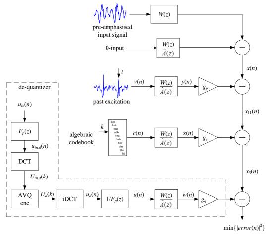
Figure 30: Schematic diagram of the ACELP encoder using a combined algebraic codebook in IC mode at high bit-rates
