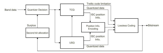
Figure 70: Block diagram of TCQ and USQ encoding with second bit allocation
