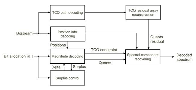
Figure 97: Block diagram for LSB TCQ decoding
