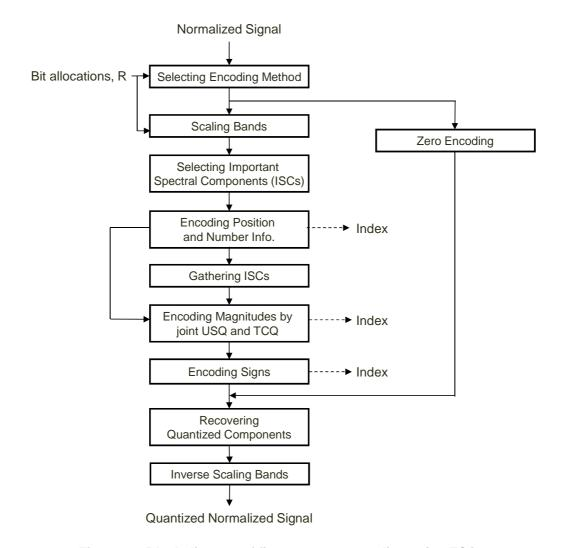
Figure 68: Block diagram of fine structure encoding using TCQ
