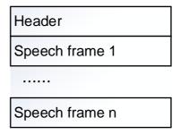
Figure A.7. Storage format for EVS
