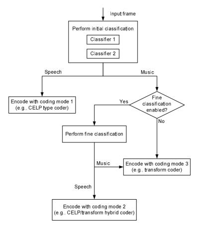
Figure 18: Multiple coding mode signal classification
