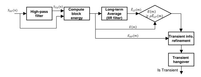
Figure 56: Transient detection algorithm for NB
