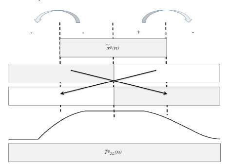
Figure 109: Unfolding and windowing with ALDO window.
