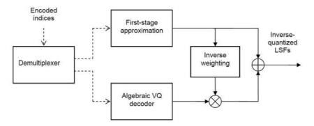
Figure 93: Overview high-rate LPC decoding
