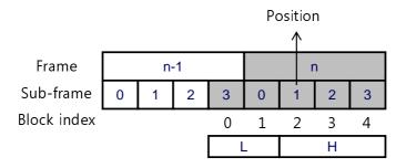
Figure 57: Transient information refinement for NB
