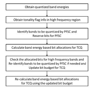
Figure 67: A flowchart of bit allocation processing for LR-HQ Normal mode.
