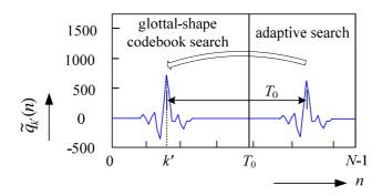
Figure 37: Glottal-shape codevector with two impulses construction
