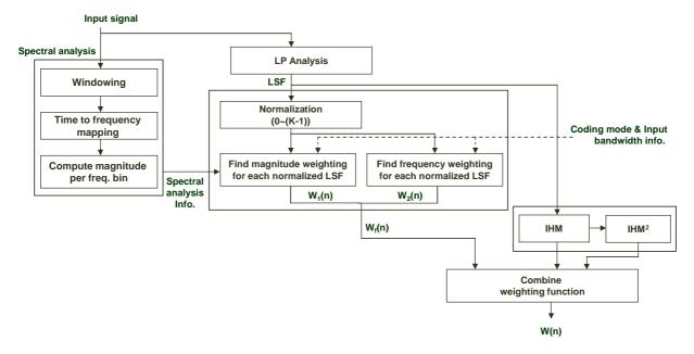
Figure 20: Block diagram of LSF weighting computation
