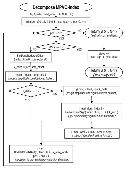
Figure 108: Detailed MPVQ-de-indexing
