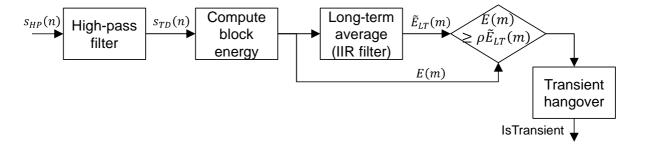
Figure 55: Transient detection algorithm
