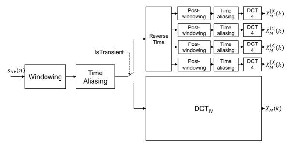
Figure 58: Adaptive time-frequency transform
