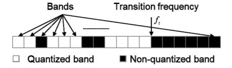
Figure 80: Estimation of transition frequency
