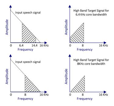
Figure 45: Generation of high band target signal for SWB TBE
