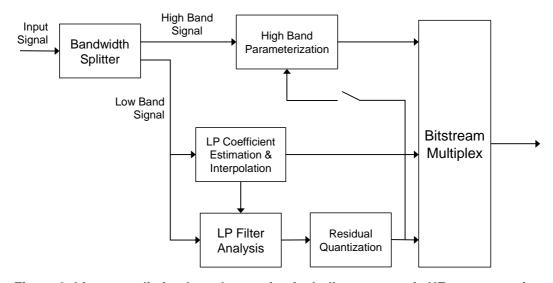
Figure 2: Linear prediction based operation including parametric HF representation
