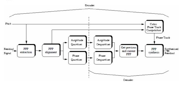
Figure 42: Block diagram of PPP coding scheme [20]
