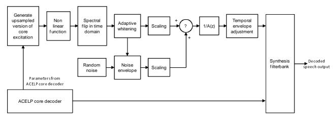
Figure 92: Time domain bandwidth extension decoder
