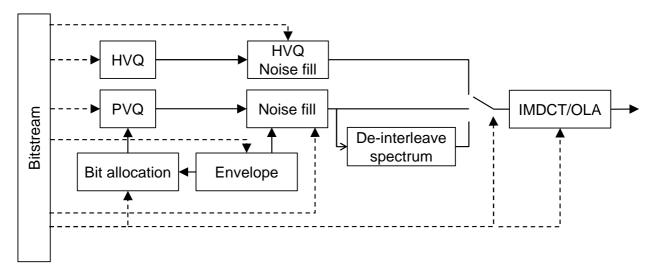
Figure 100: High level structure of the high-rate HQ decoder
