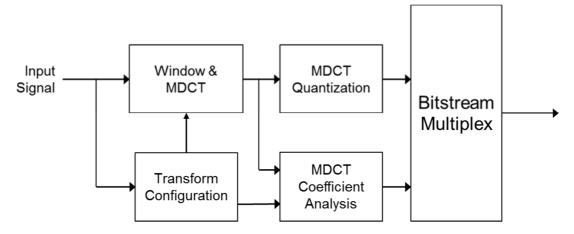
Figure 3: Frequency domain encoder
