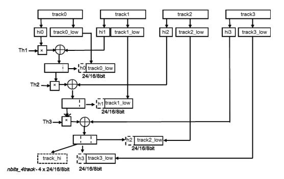
Figure 28: Schematic diagram of 4-track joint coding
