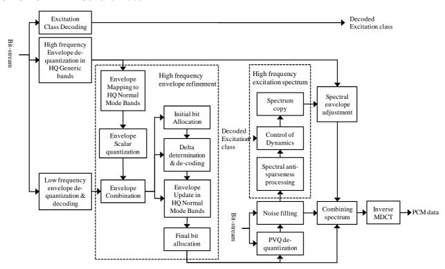
Figure 107: Generic mode Decoder Block Diagram
