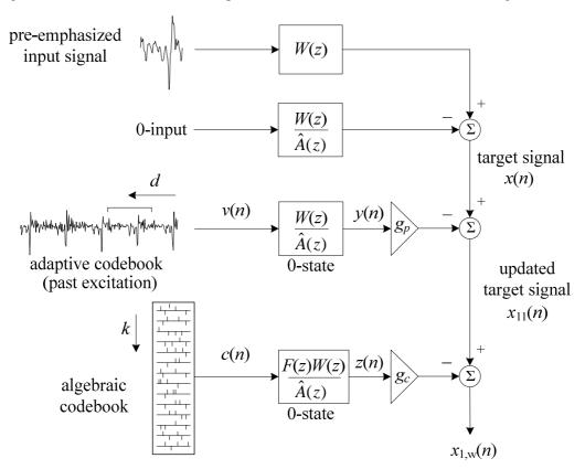
Figure 25: Schematic diagram of the excitation coding in GC and VC mode
