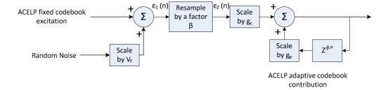
Figure 49: Generating the upsampled version of the lowband excitation
