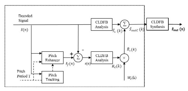
Figure 91: Block diagram of bass post-filter
