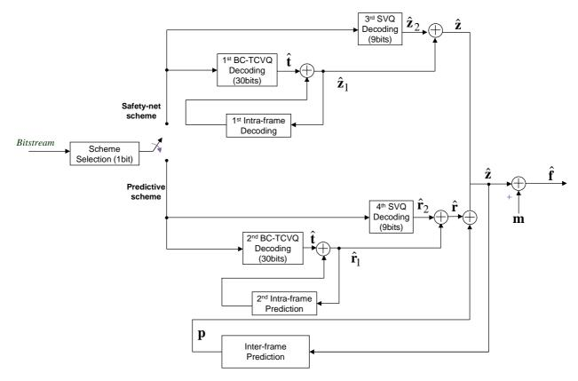
Figure 89: Block diagram of the decoder for the predictive BC-TCVQ/SVQ with safety-net for an encoding rate of 40 bits per frame
