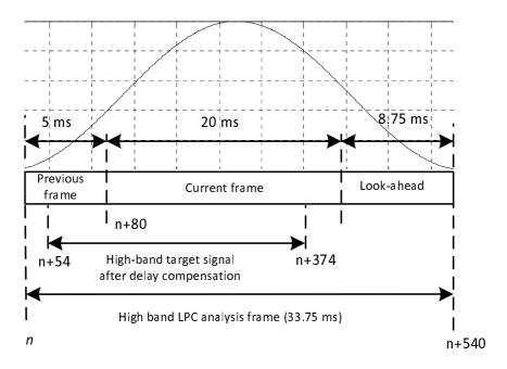
Figure 47: SWB Highband target signal buffers
