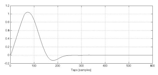
Figure 4: Impulse response of CLDFB prototype filter with 600 taps for 48 kHz sample rate
