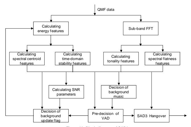
Figure 12: Block diagram of SAD3
