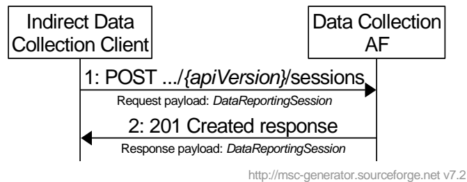
Figure 4.2.4.2-1: Initial configuration of Indirect Data Collection Client
