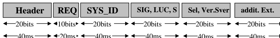
Figure 7.4-5: Construction of a TFO_REQ Message with Selector, TFO_Version.Subversion and one additional Extension_Block
