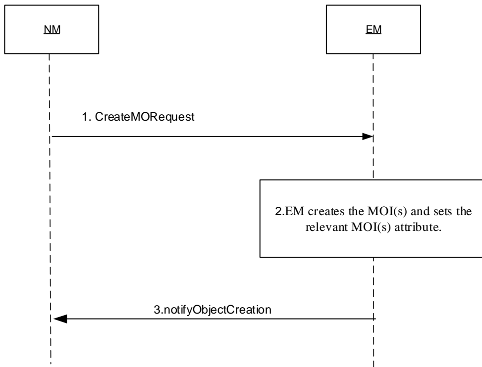
Figure 4.4.2-1: Creating MO with VNF instance identifier specified
