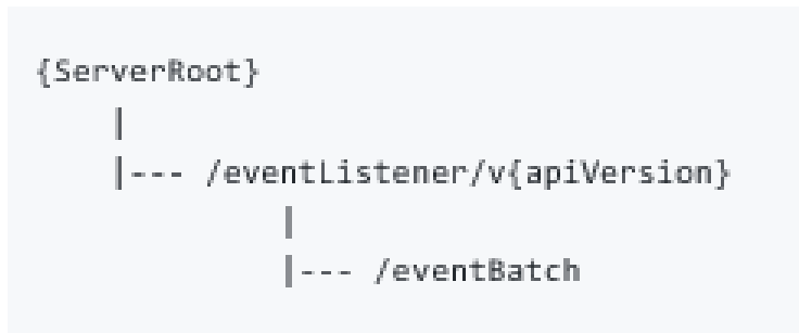
Figure 12.1.2.3.1-1: Resource URI structure of the provisioning MnS for integration with ONAP VES Event Listener 7.1.1 (Resource structure section) [45]
