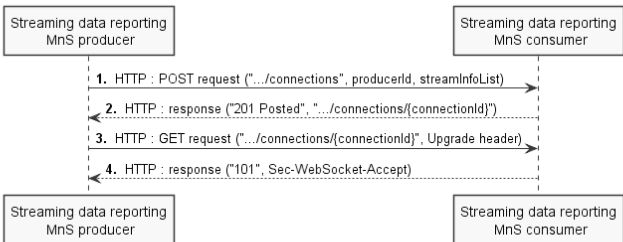
Figure 12.5.1.1.2-1: Message flow for establishing a streaming connection
