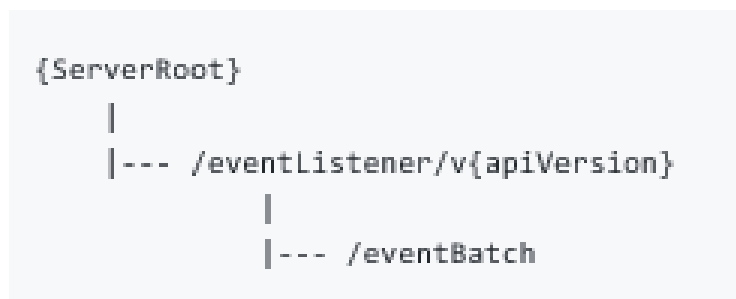
Figure 12.1.2.3.1-1: Resource URI structure of the provisioning MnS for integration with ONAP VES Event Listener 7.1.1 (Resource structure section) [45]
