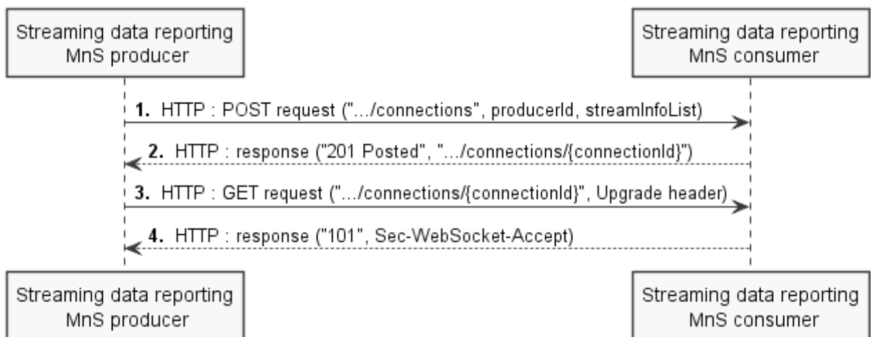
Figure 12.5.1.1.2-1: Message flow for establishing a streaming connection
