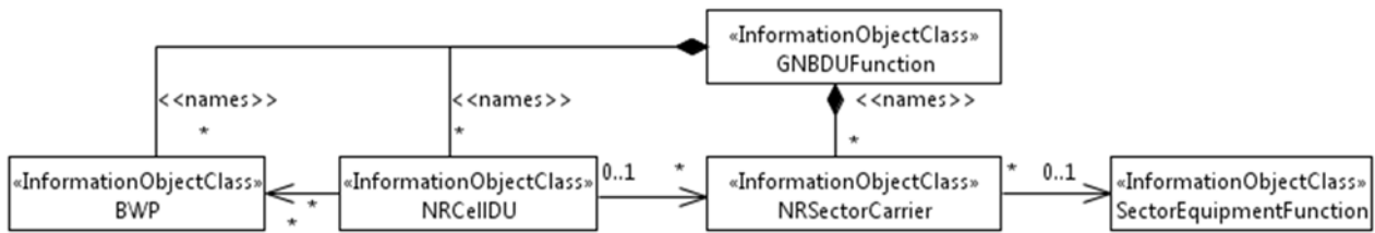
Figure 4.2.1.1-3: NRM for <<IOC>>NRSectorCarrier and <<IOC>>BWP for all deployment scenarios
