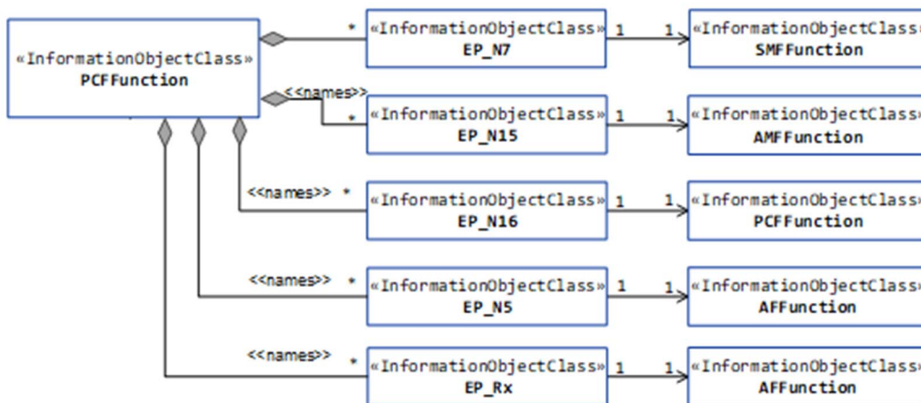
Figure 5.2.1.1-6: Transport view of PCF NRM
