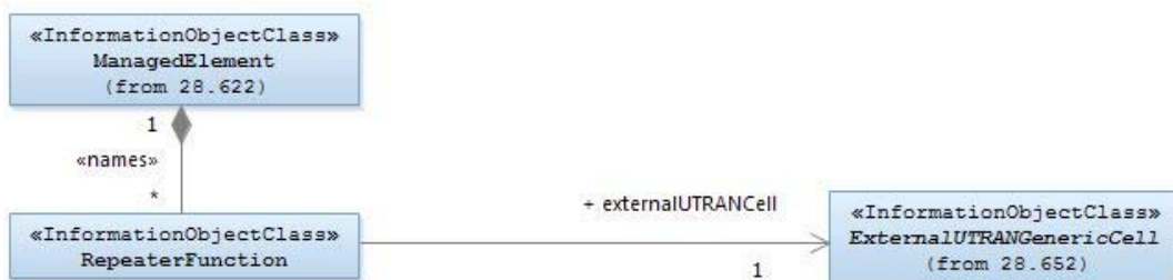
Figure 4.2.1.4: Repeater object Containment/Naming and Association diagram
