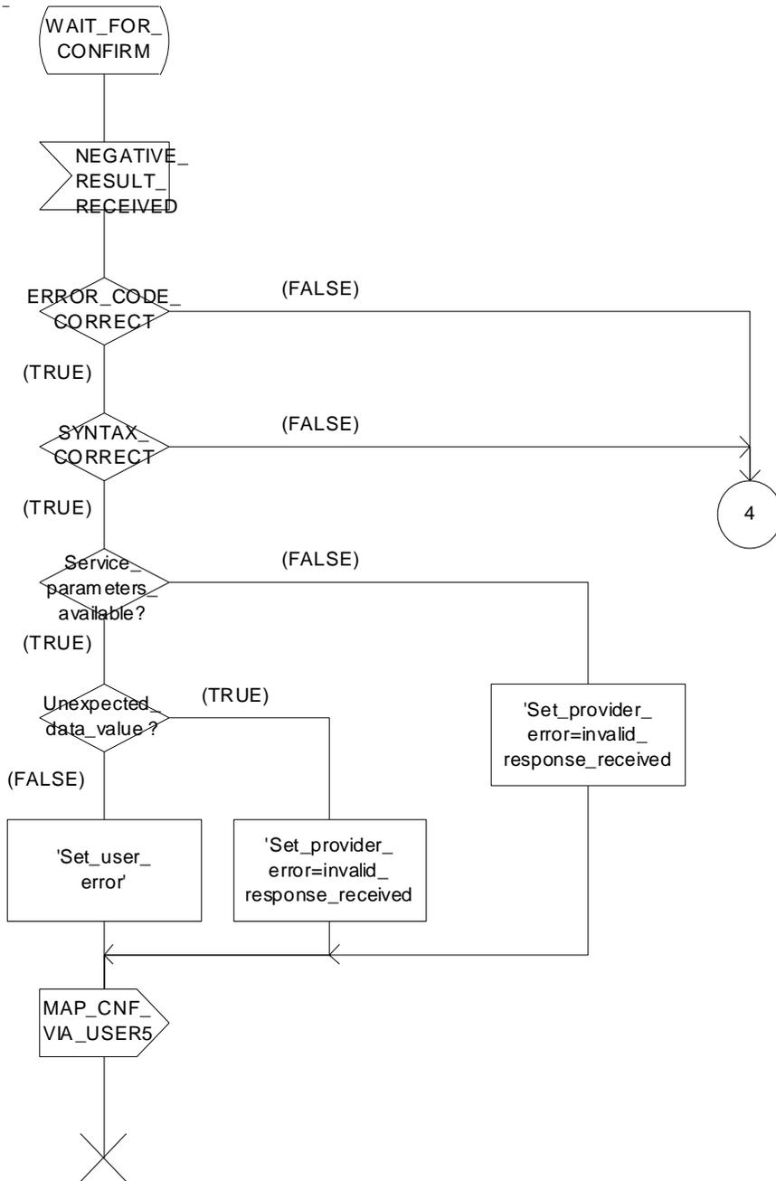
Figure 16.2/7 (sheet 3 of 4): Process REQUESTING\_MAP\_SSM
