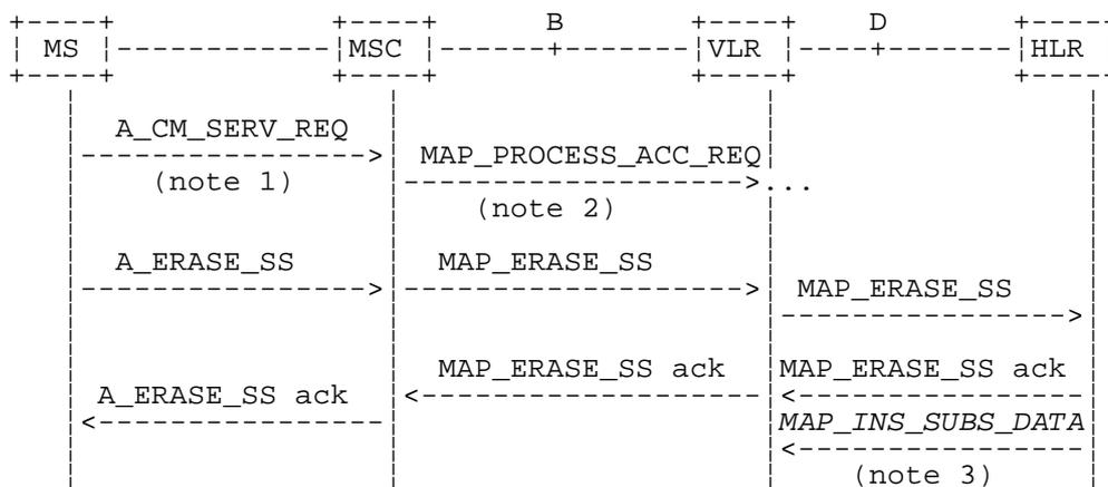
**Figure 22.3.1/1: Interfaces and services for supplementary service erasure**
