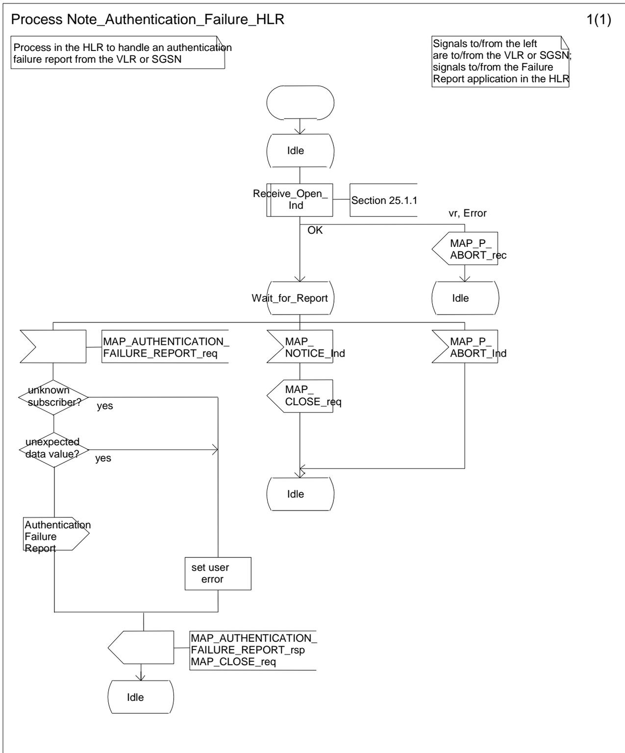
Figure 25.6/10: Process Note\_Authentication\_Failure\_HLR
