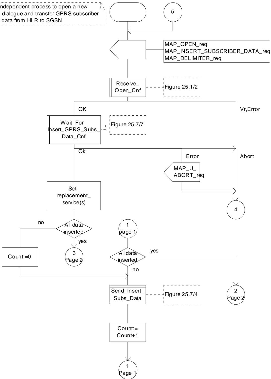
Figure 25.7/5 (sheet 1 of 2): Process Insert\_GPRS\_Subscriber\_Data\_Stand\_Alone\_HLR
