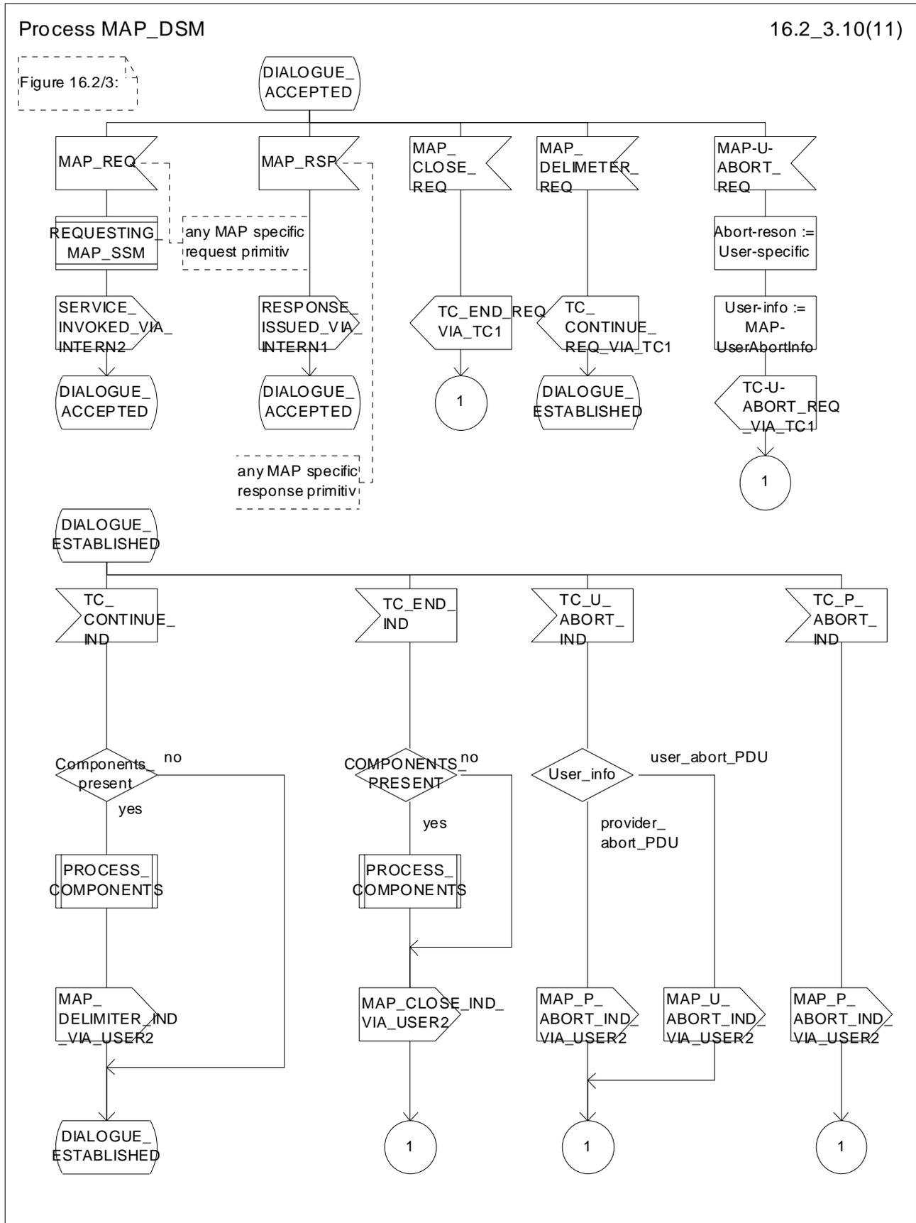
Figure 16.2/3 (sheet 10 of 11): Process MAP\_DSM
