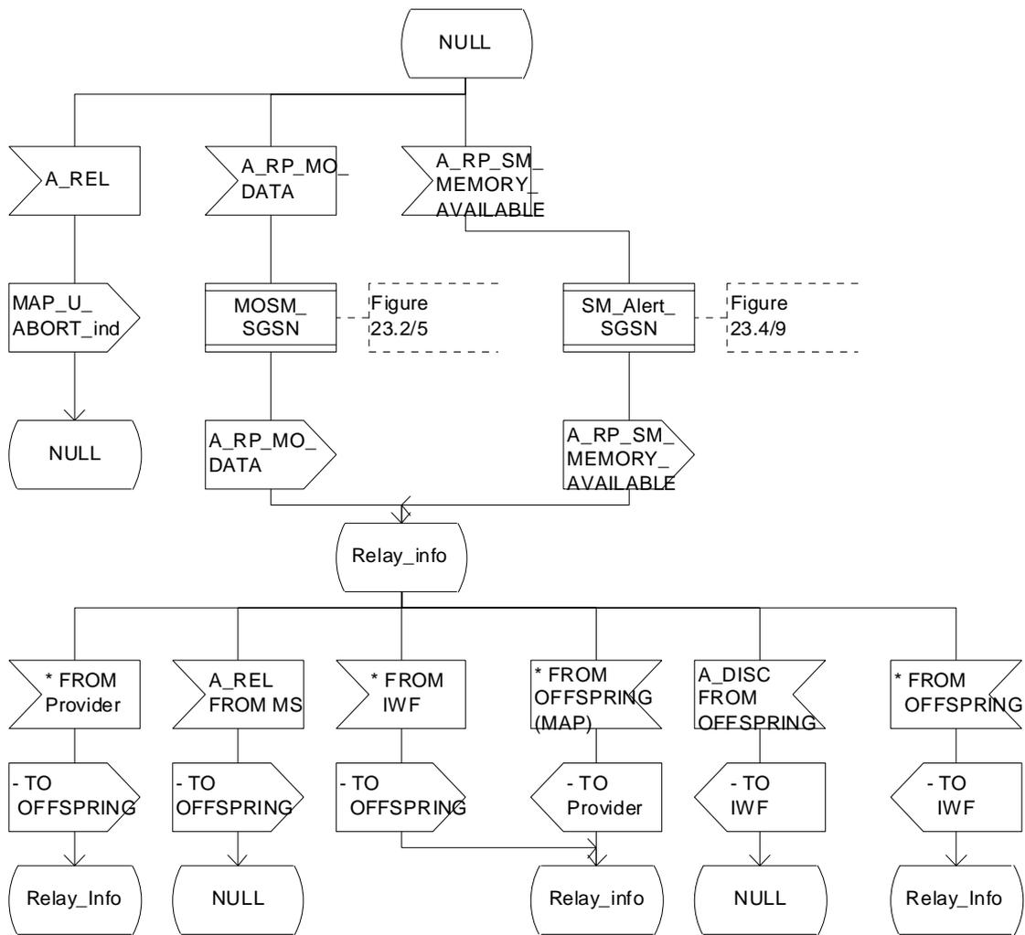
Figure 23.1/3: Process Co\_SMS\_SGSN
