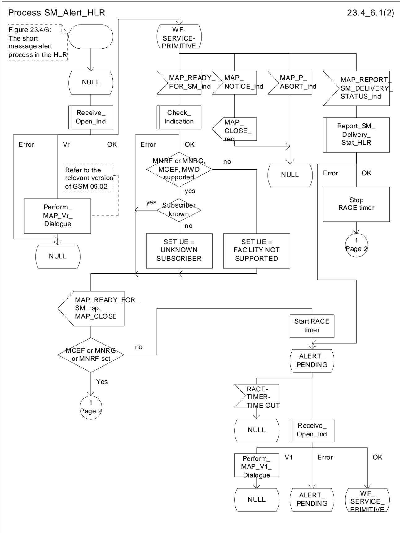
Figure 23.4/6 (sheet 1 of 2): Process SM\_Alert\_HLR
