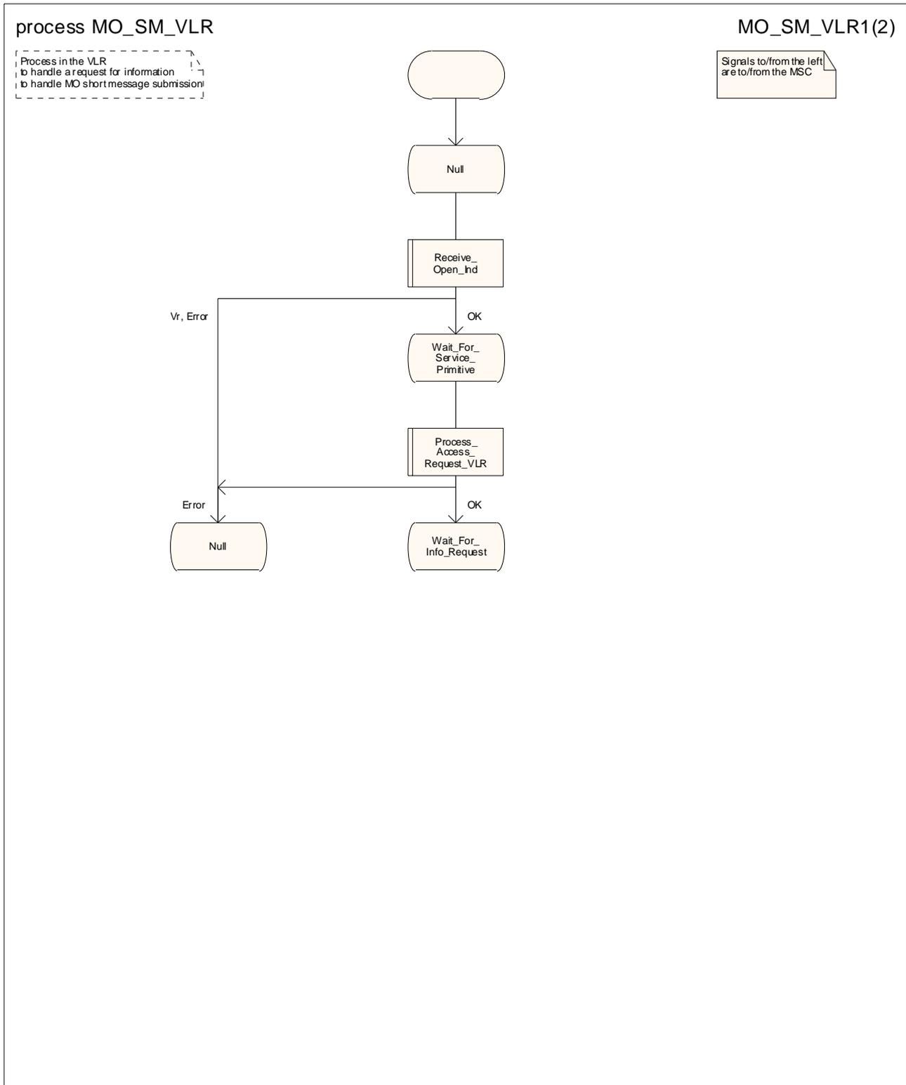
Figure 23.2/3(sheet 1 of 2): Process MOSM\_VLR
