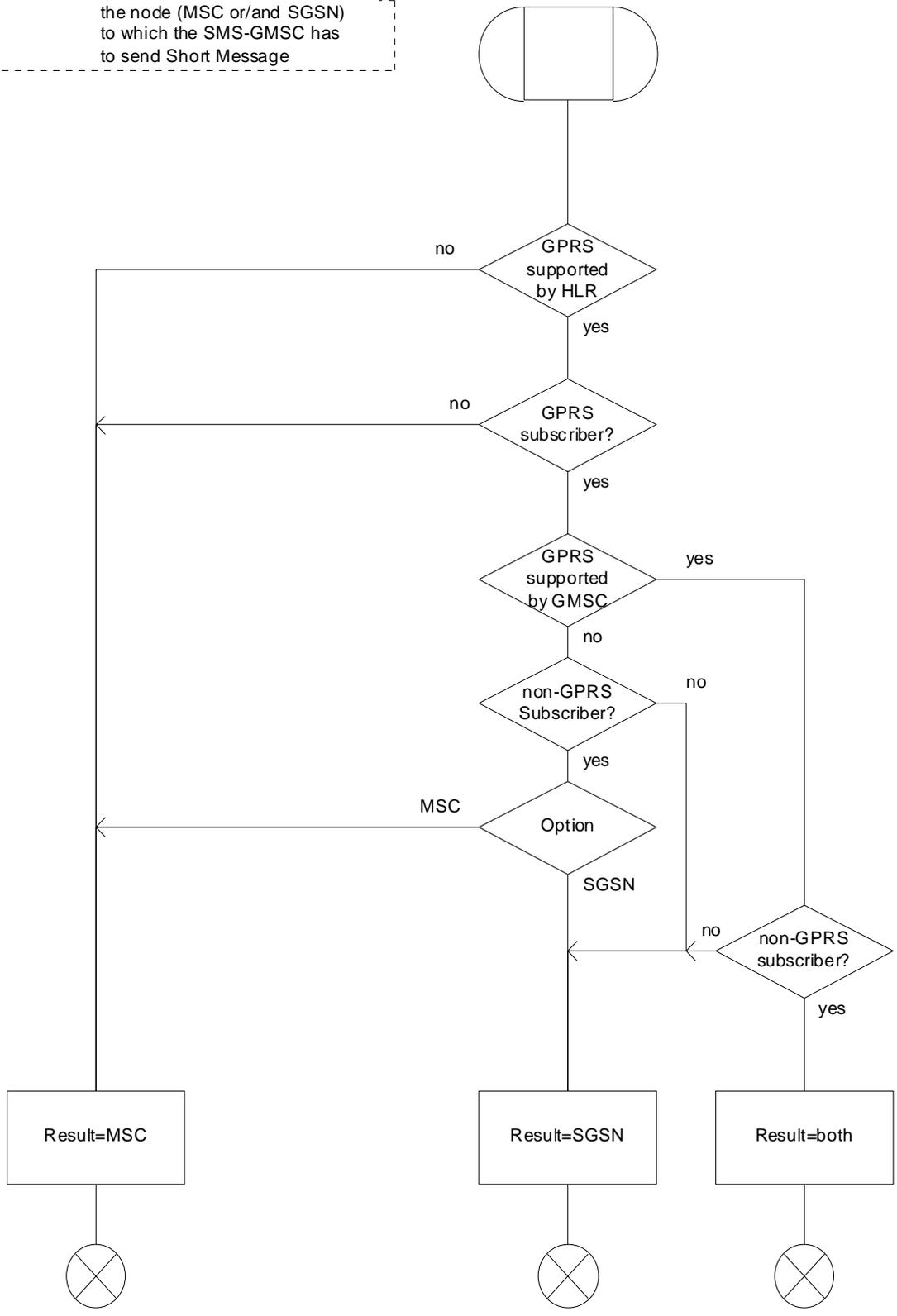
Figure 23.3/11: Procedure Select\_Transfer\_Nodes
