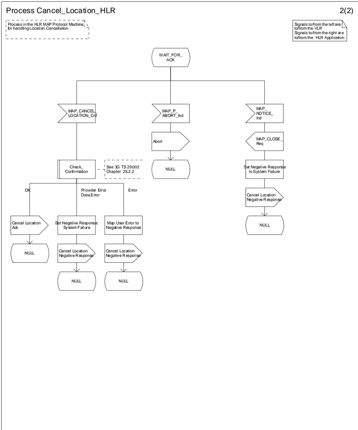
Figure 19.1.2/2 (Sheet 2 of 2): Process Cancel\_Location\_HLR
