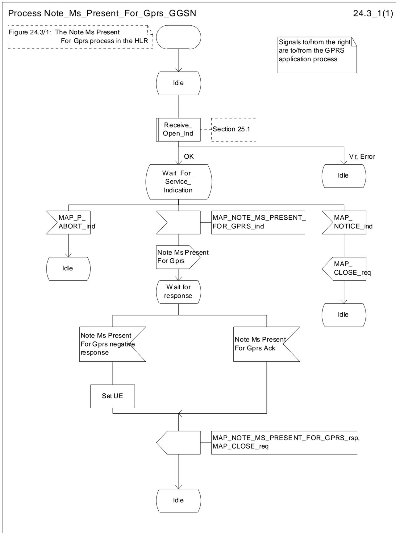
Figure 24.3/1: Process Note\_Ms\_Present\_For\_Gprs\_GGSN
