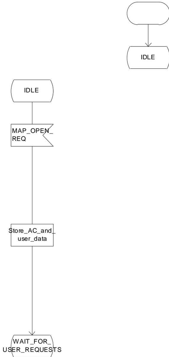
Figure 16.2/3 (sheet 1 of 11): Process MAP\_DSM
