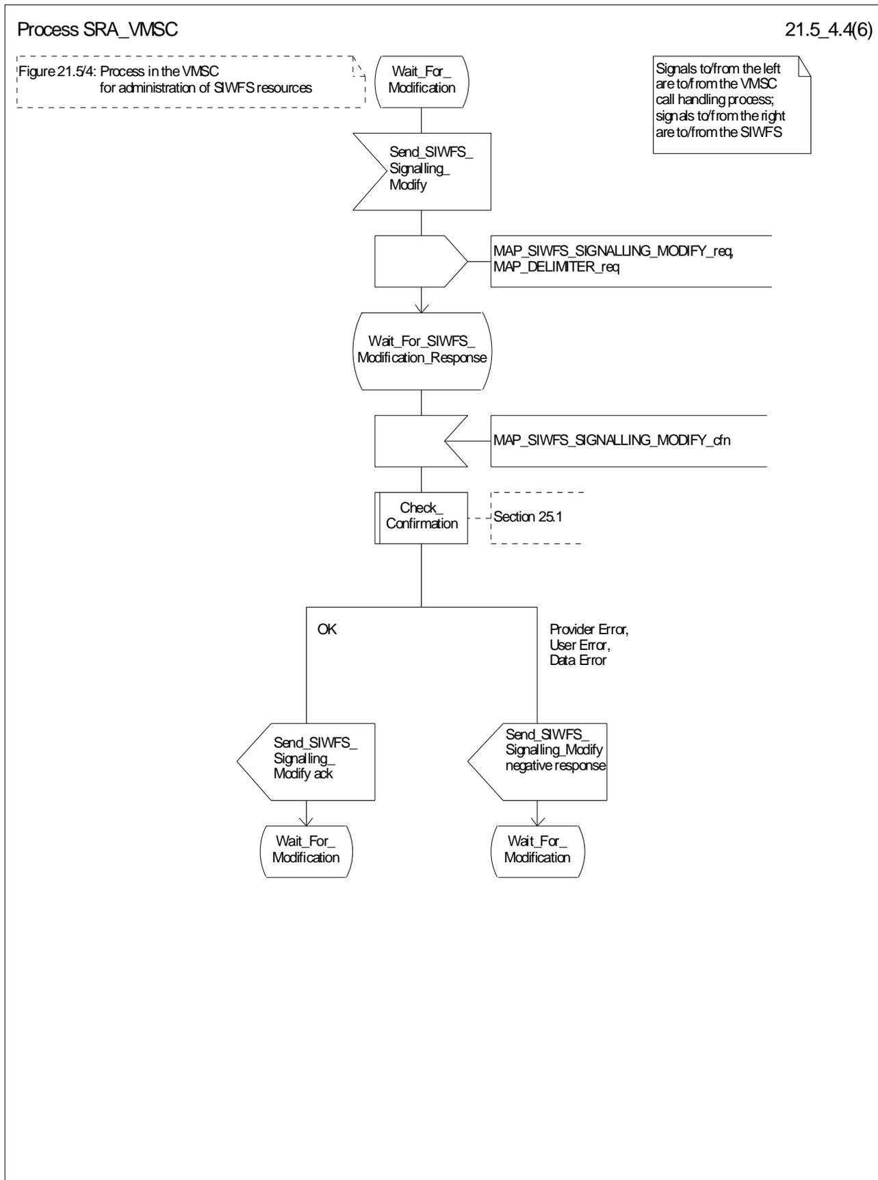
Figure 21.5/4 (sheet 4 of 6): Process SRA\_VMSC
