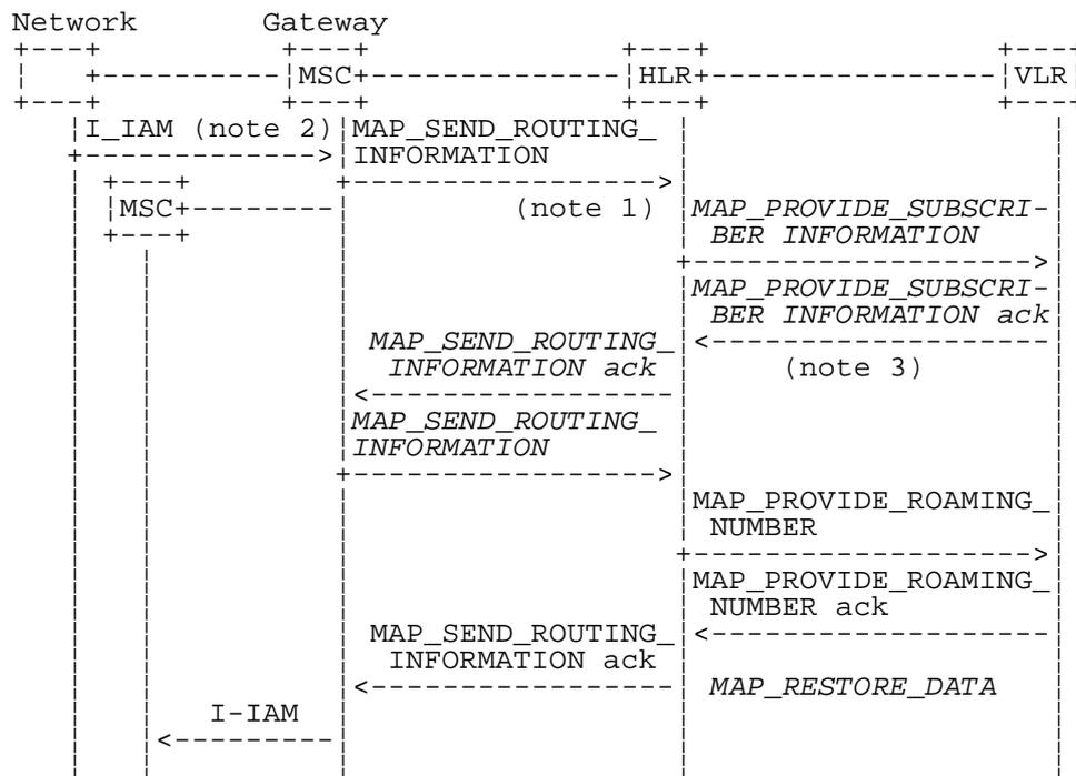
**Figure 21.2/1: Message flow for retrieval of routing information (non-optimally routed call)**
