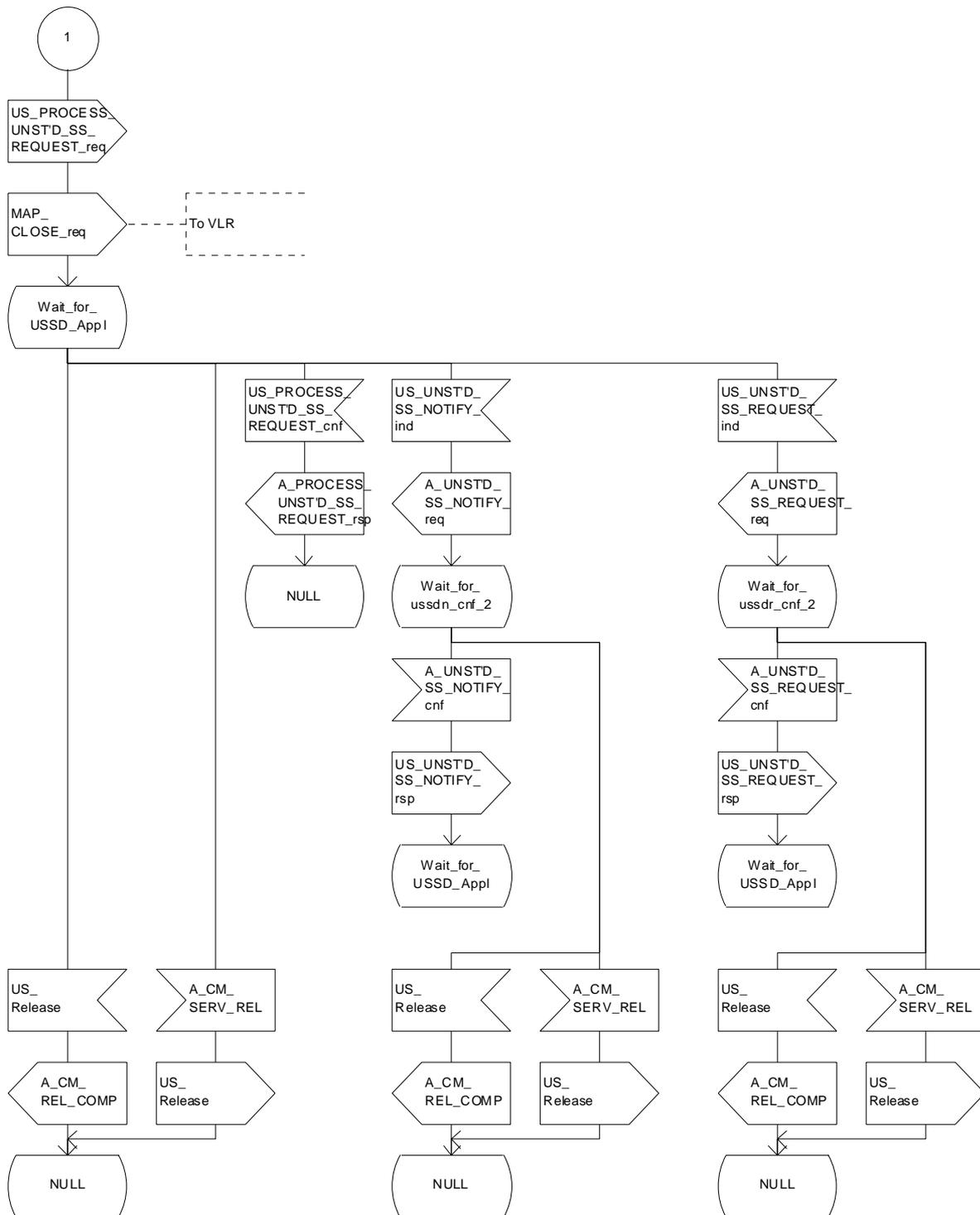
Figure 22.9.2/1 (sheet 2 of 2): Procedure MI\_USSD\_MSC
