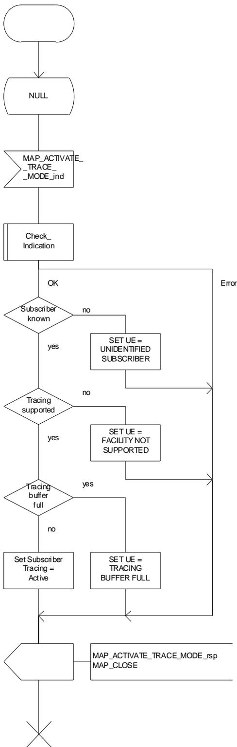
Figure 20.2/9: Process ATM\_VLR\_Standalone
