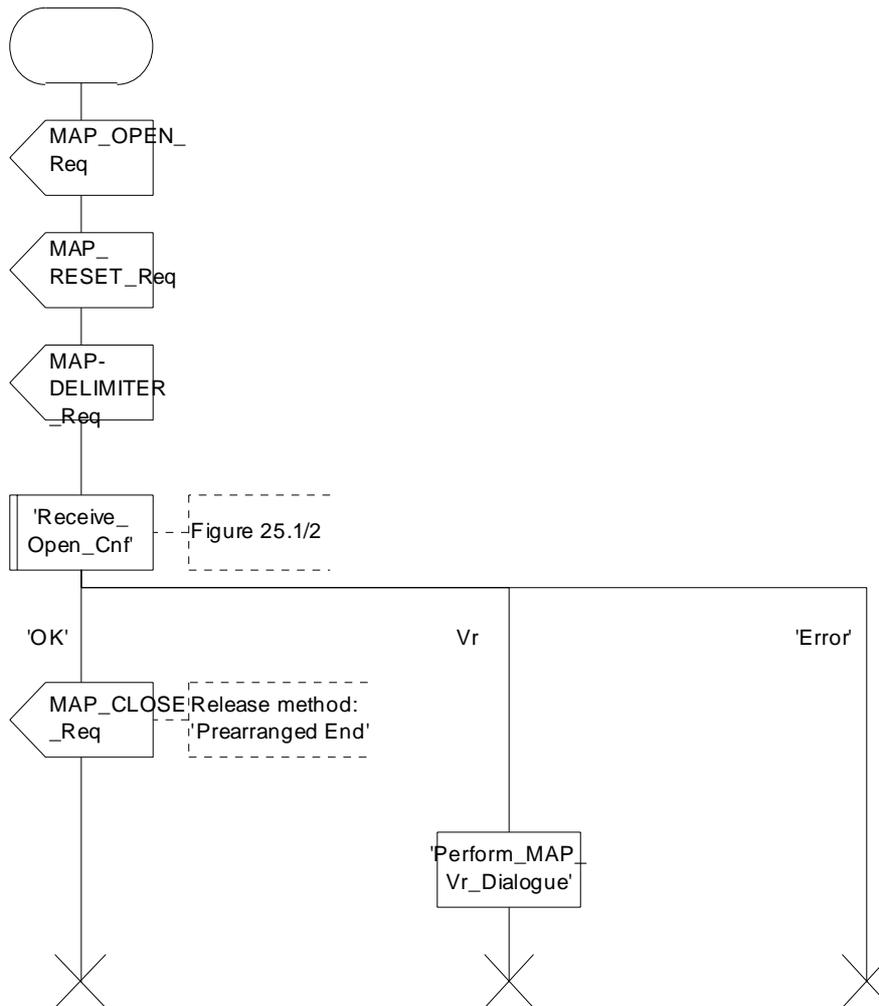
Figure 19.3/7: Process SEND\_RESET\_TO\_SGSN
