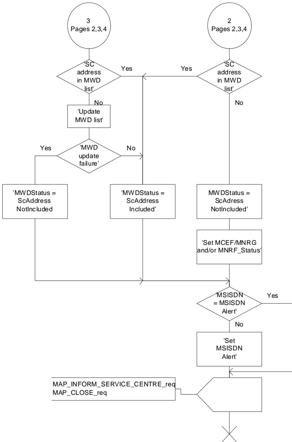
Figure 23.3/6 (sheet 5 of 5): Process Mobile\_terminated\_SM\_HLR
