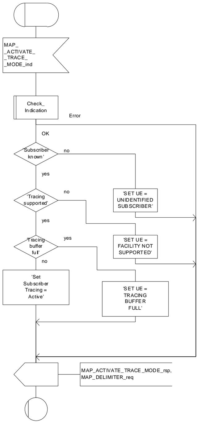
Figure 25.9/3: Macro Activate\_Tracing\_VLR
