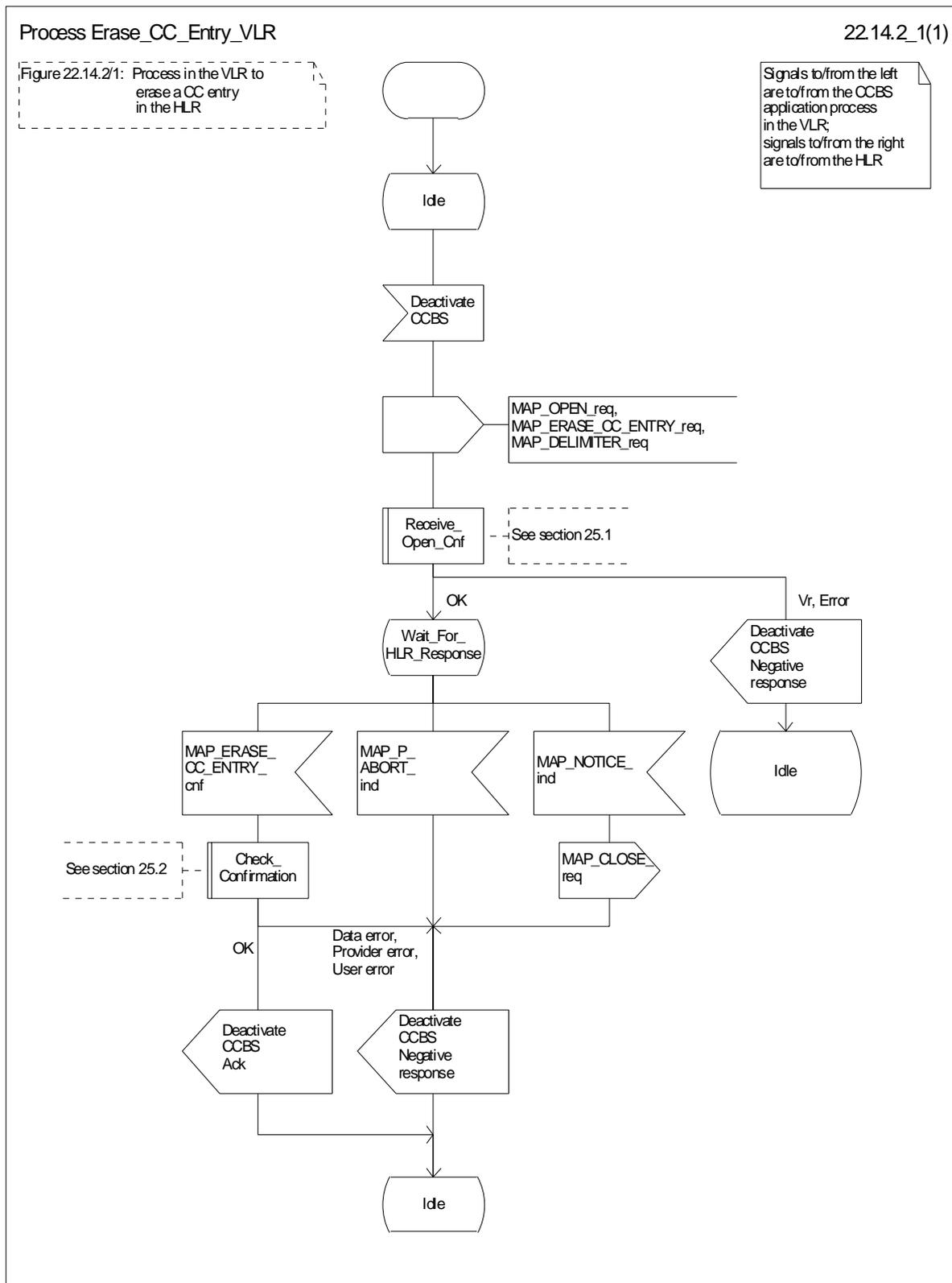
Figure 22.14.2/1: Process Erase\_CC\_Entry\_VLR
