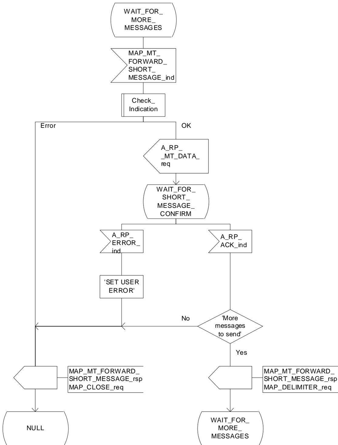
Figure 23.3/9 (sheet 2 of 3): Procedure MT\_SM\_Transfer\_SGSN
