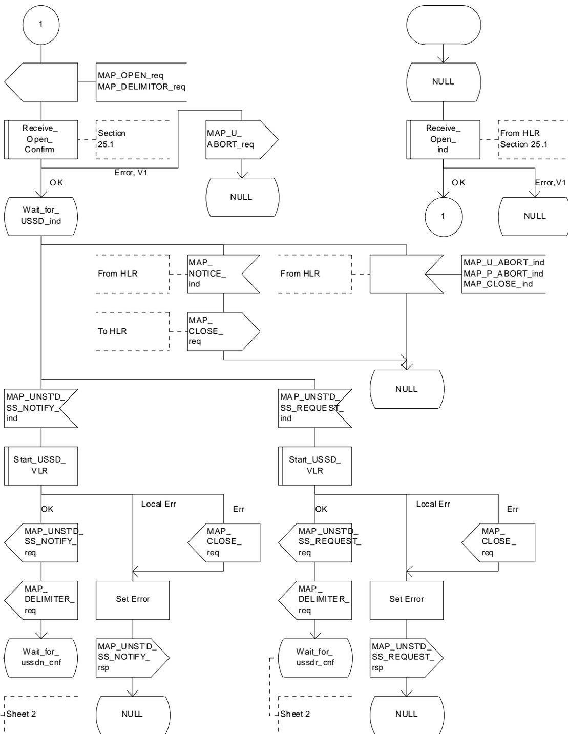
Figure 22.10.3/1 (sheet 1 of 4): Procedure NI\_USSD\_VLR
