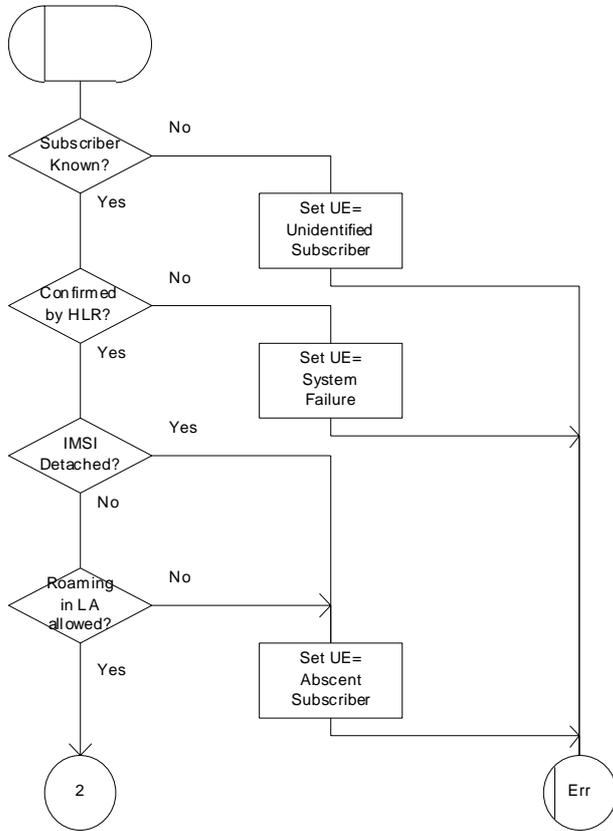
Figure 22.10.3/2 (sheet 1 of 2): Macro Start\_USSD\_VLR
