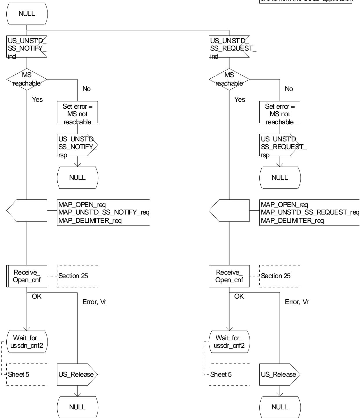
Figure 22.10.4/1 (sheet 4 of 5): Procedure NI\_USSD\_HLR
