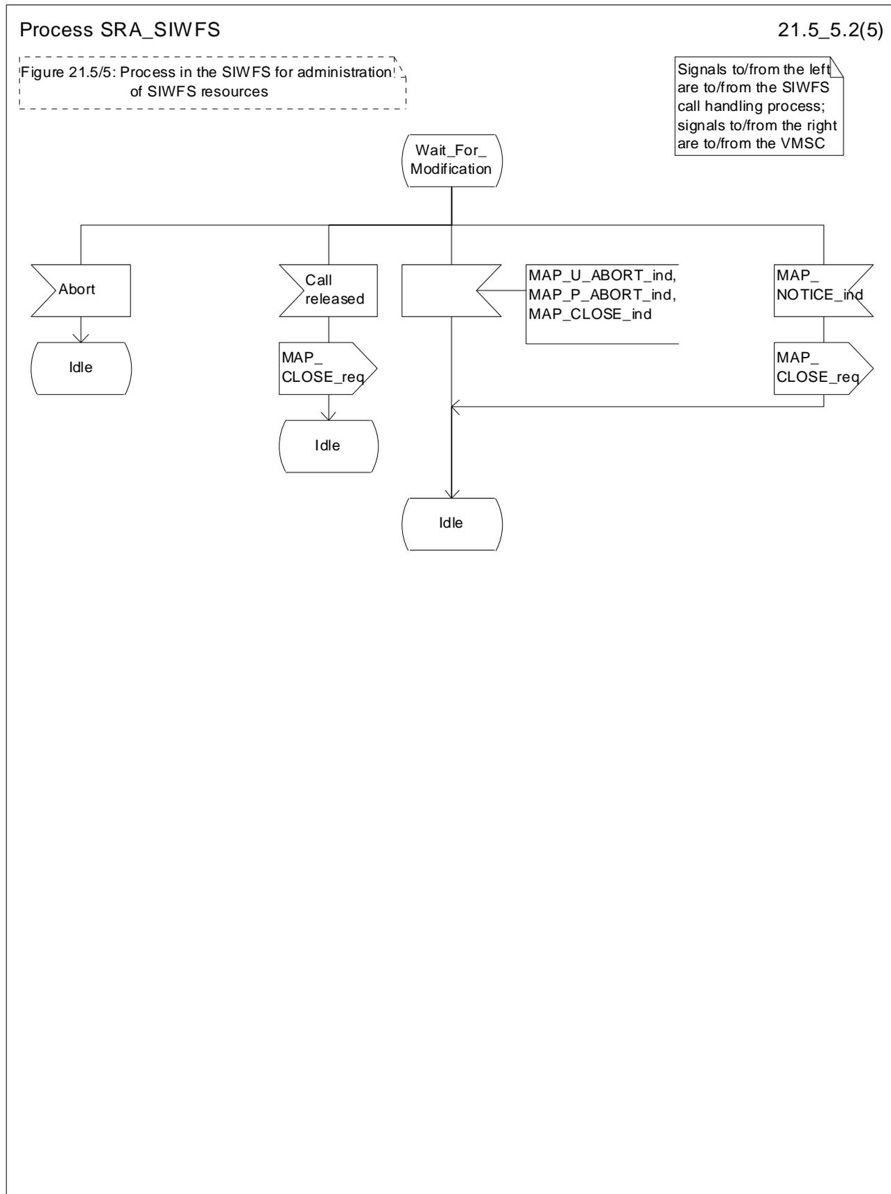
Figure 21.5/5 (sheet 2 of 5): Process SRA\_SIWFS
