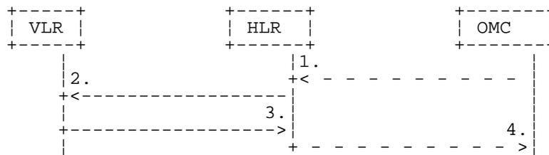
**Figure 20.3/1: Subscriber deletion procedure**
