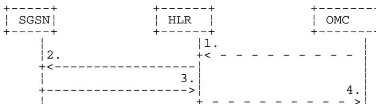
**Figure 20.3/9: Subscriber data modification procedure for GPRS**
