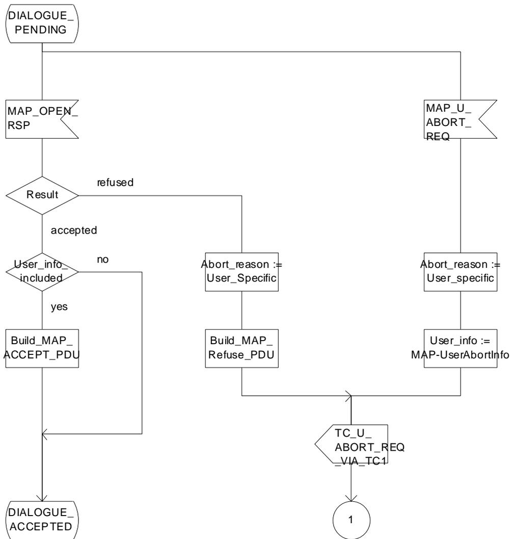
Figure 16.2/3 (sheet 9 of 11): Process MAP\_DSM
