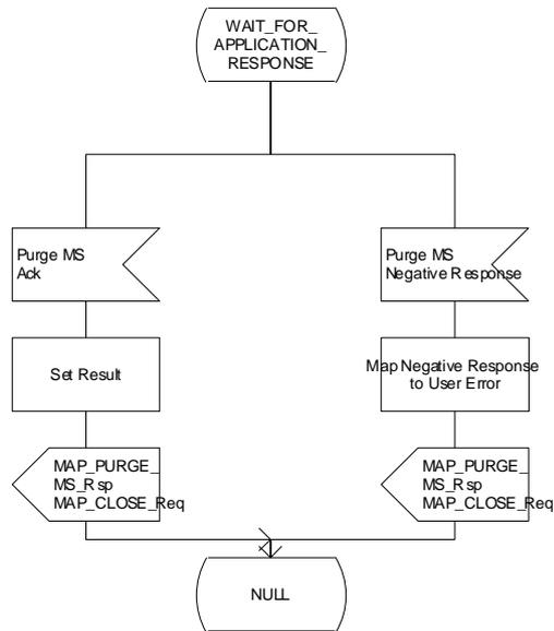
Figure 19.1.4/3 (Sheet 2 of 2): Process Purge\_MS\_HLR
