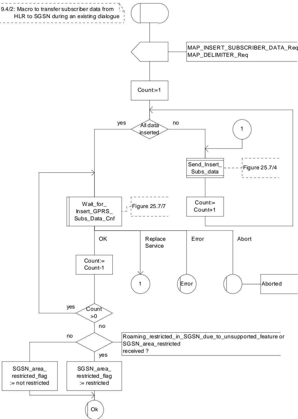
Figure 19.4/2: Macro Insert\_Subs\_Data\_In\_SGSN\_Framed\_HLR
