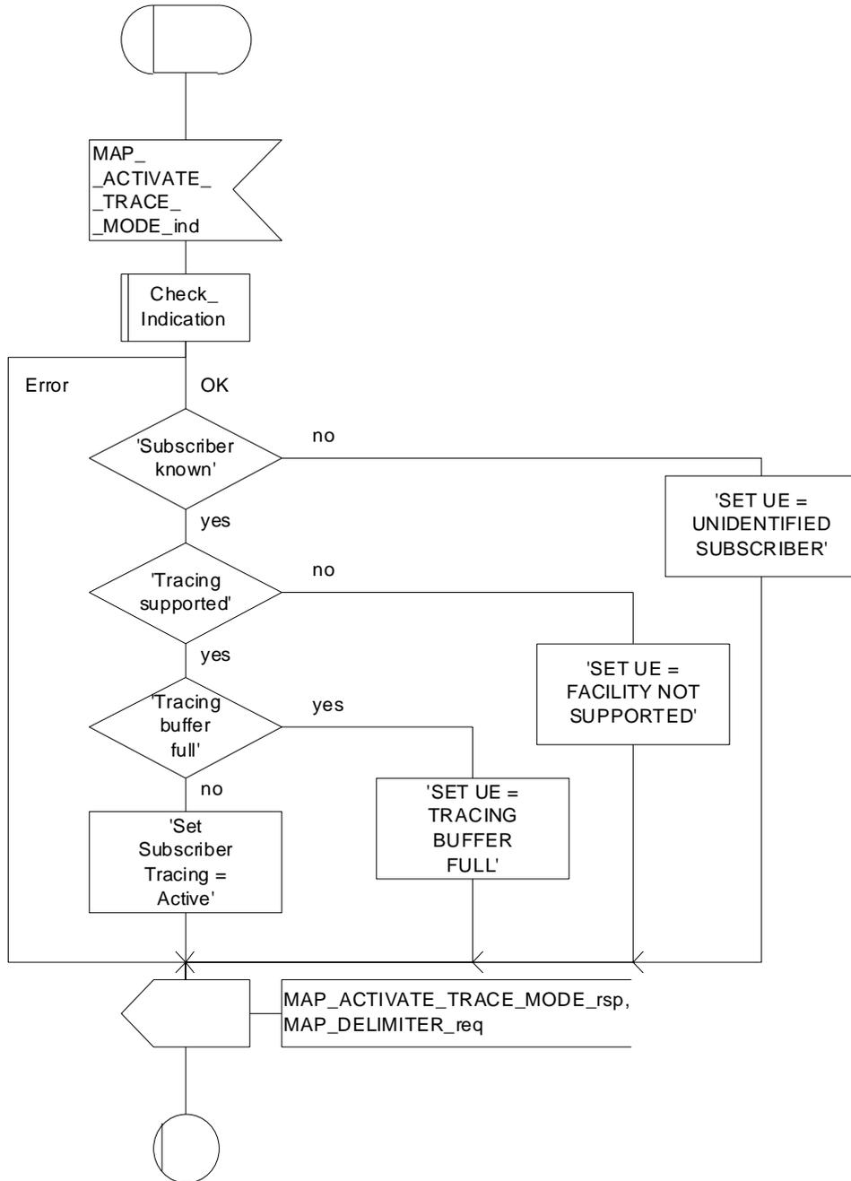
Figure 25.9/7: Macro Activate\_Tracing\_SGSN
