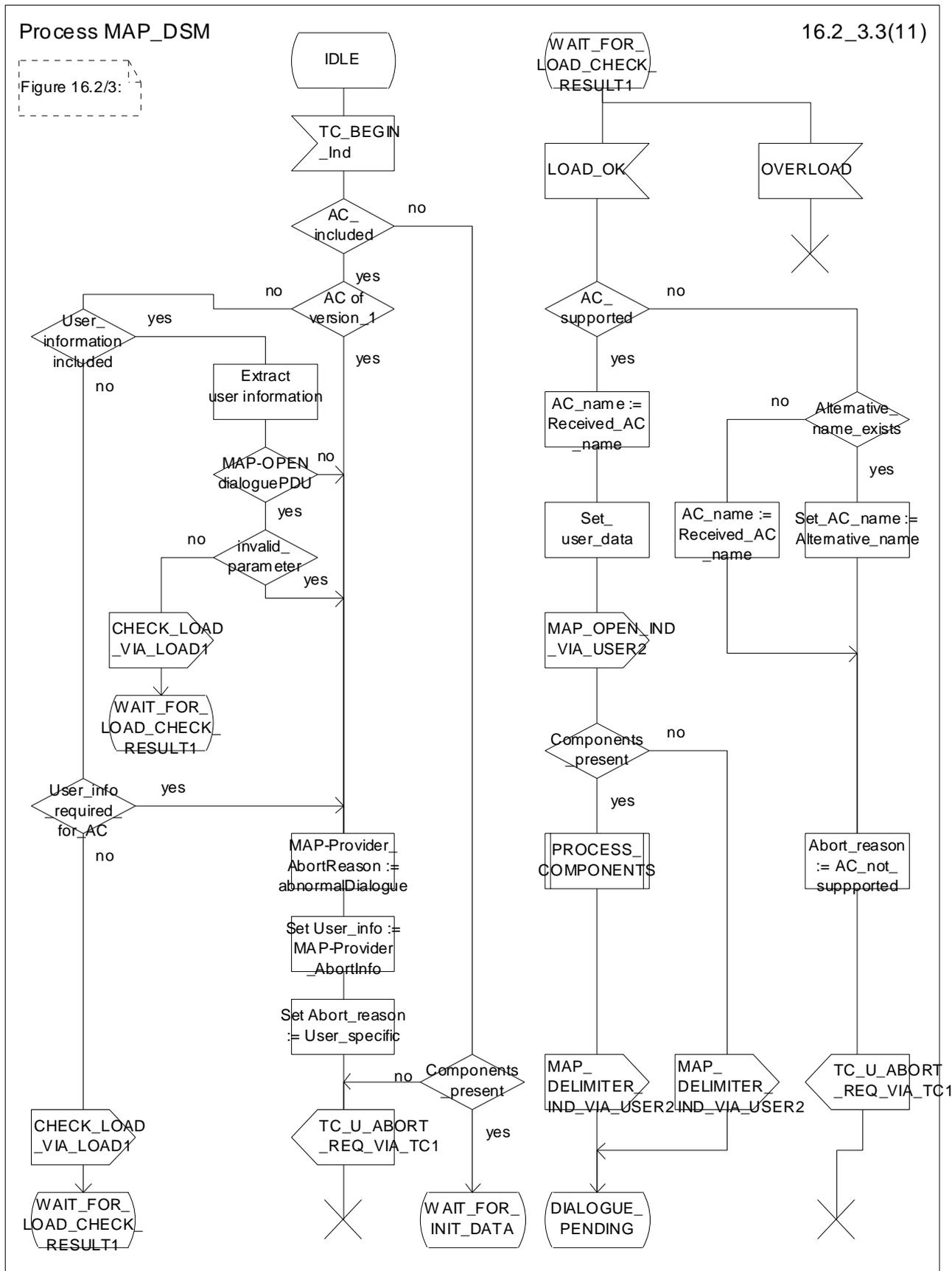
Figure 16.2/3 (sheet 3 of 11): Process MAP\_DSM
