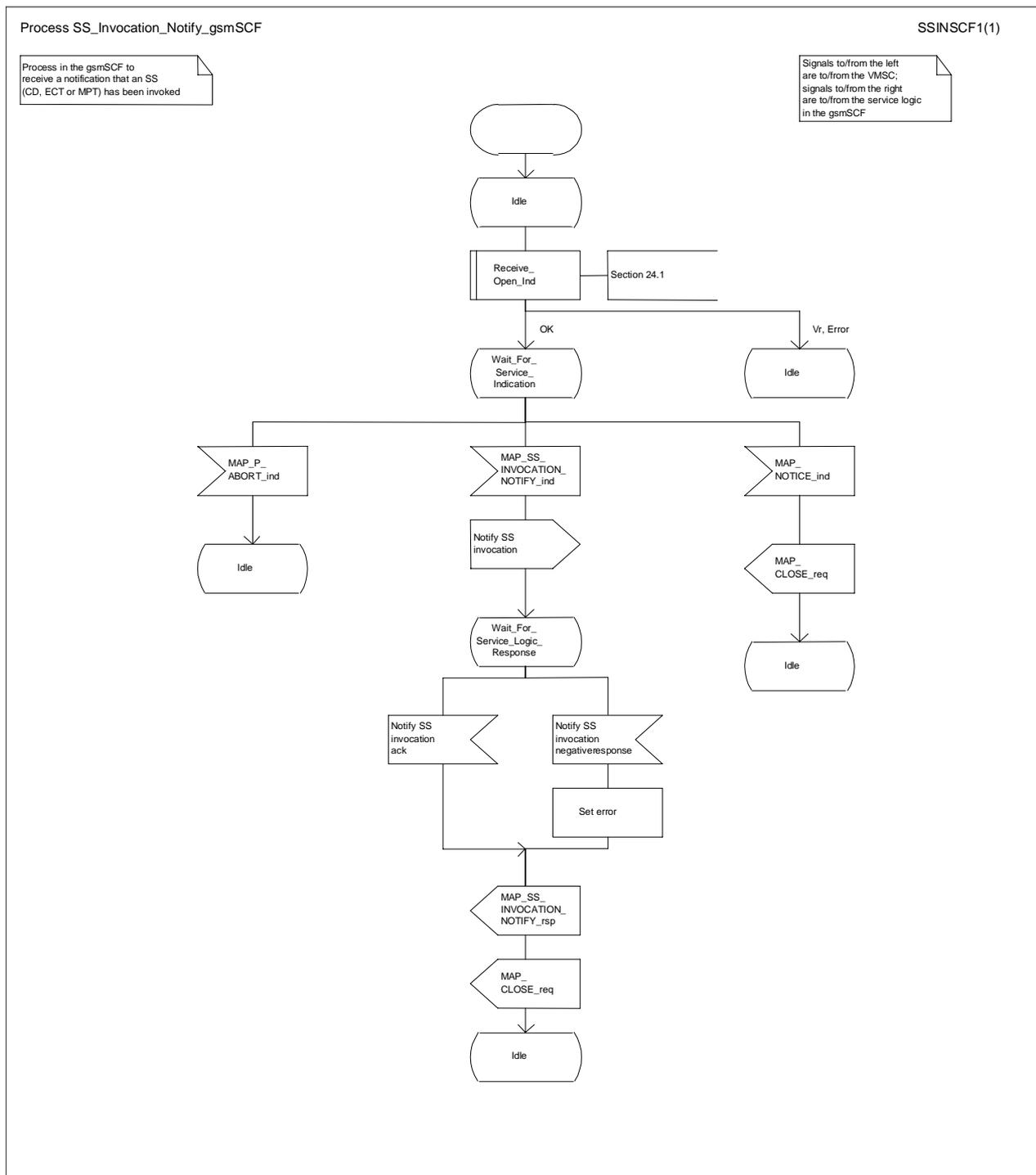
Figure 22.12.3/1: Process SS\_Invocation\_Notify\_gsmSCF (sheet 1 of 1)
