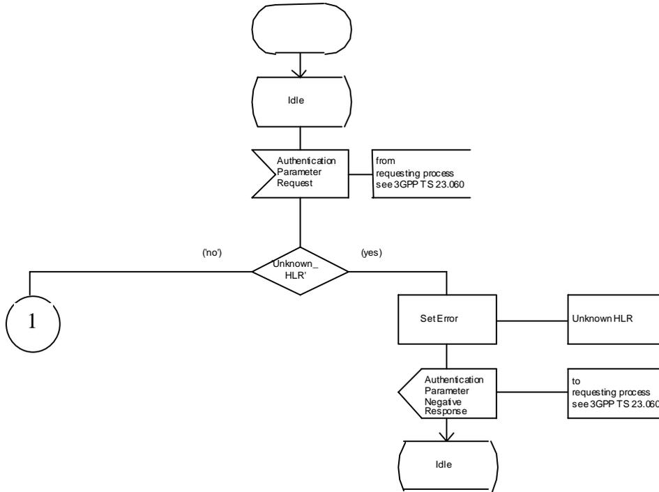
Figure 25.5/6 (sheet 1 of 3): Process Obtain\_Authen\_Para\_SGSN
