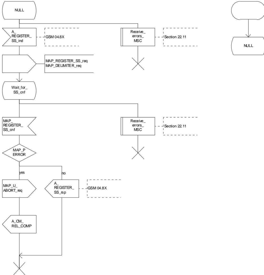
Figure 22.2.2/1: Procedure SS\_Register\_MSC
