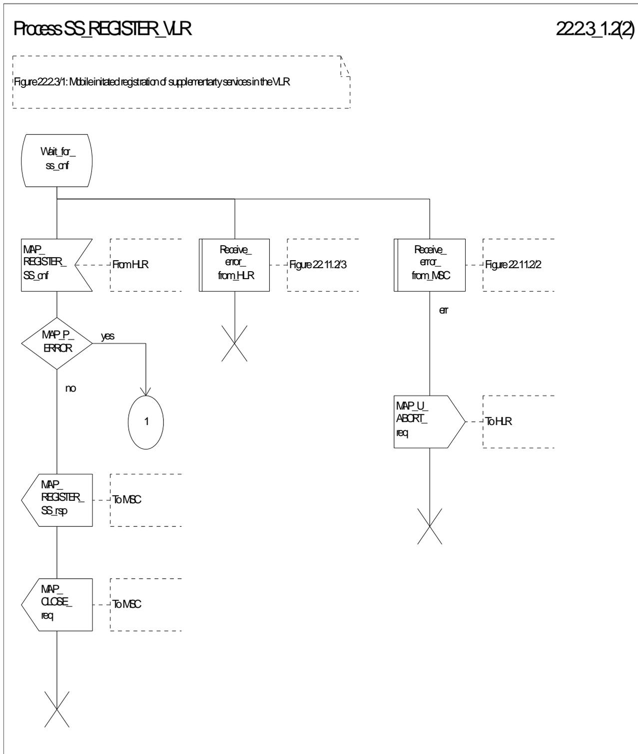
Figure 22.2.3/1 (sheet 2 of 2): Procedure SS\_Register\_VLR
