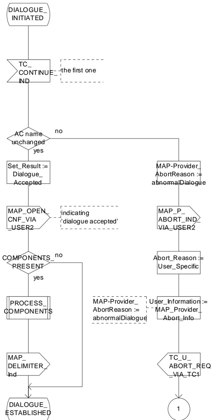
Figure 16.2/3 (sheet 6 of 11): Process MAP\_DSM
