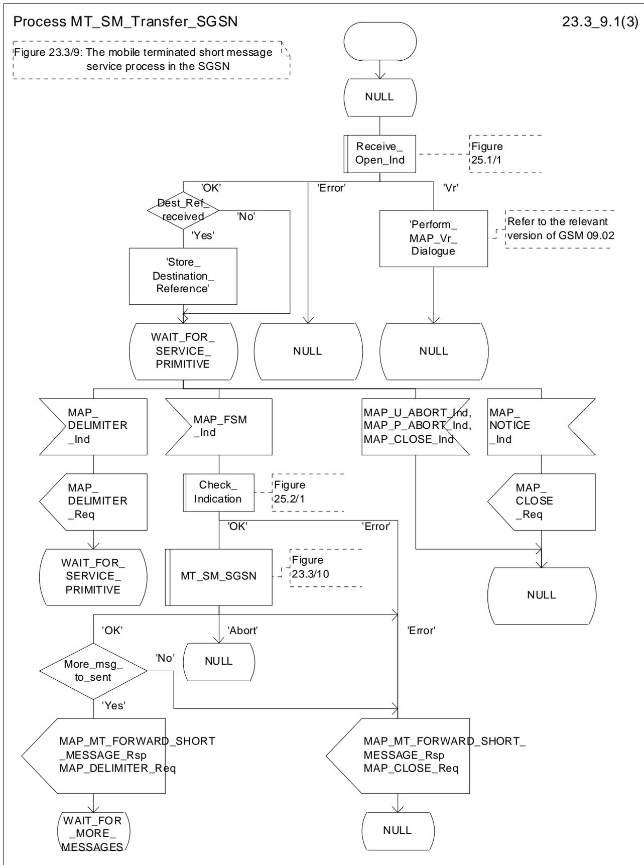
Figure 23.3/9 (sheet 1 of 3): Procedure MT\_SM\_Transfer\_SGSN
