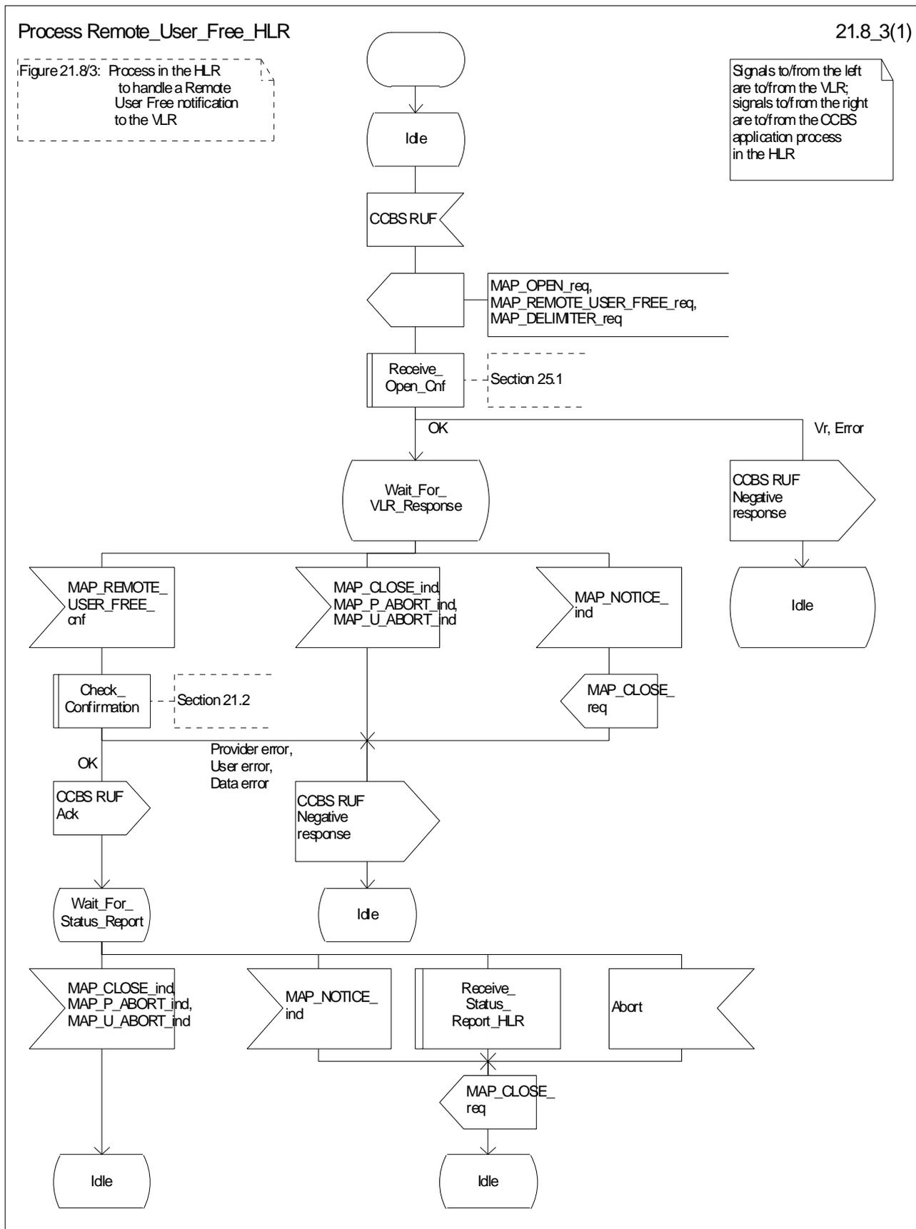
Figure 21.8/3: Process Remote\_User\_Free\_HLR
