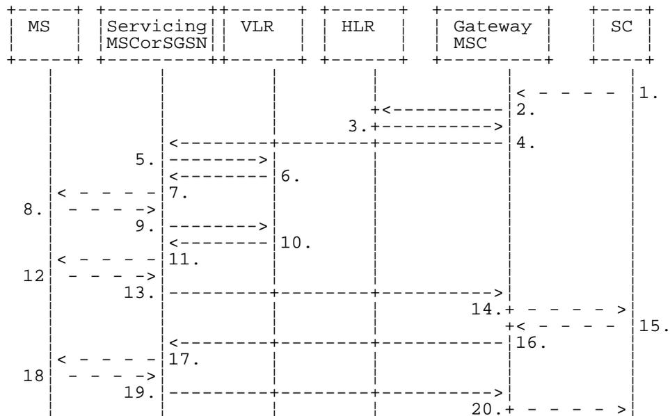
**Figure 23.3/2: Mobile terminated short message procedure for multiple short message transfer**
