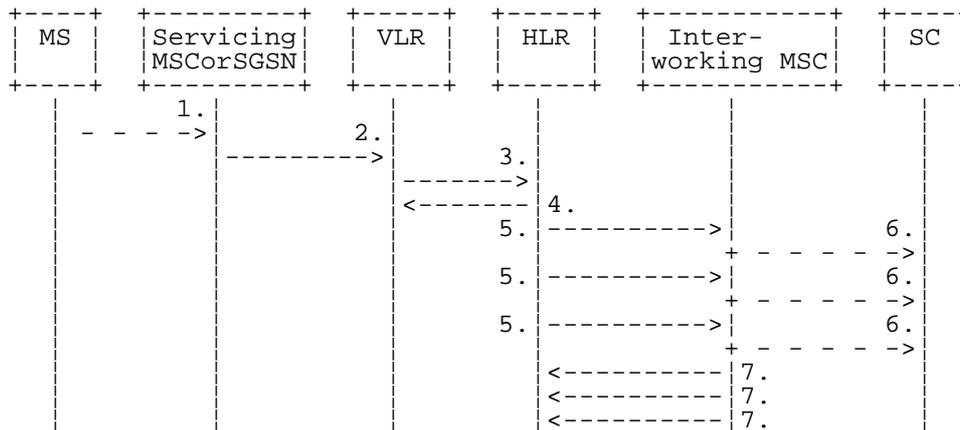
**Figure 23.4/1: Short message alert procedure (Mobile is present)**
