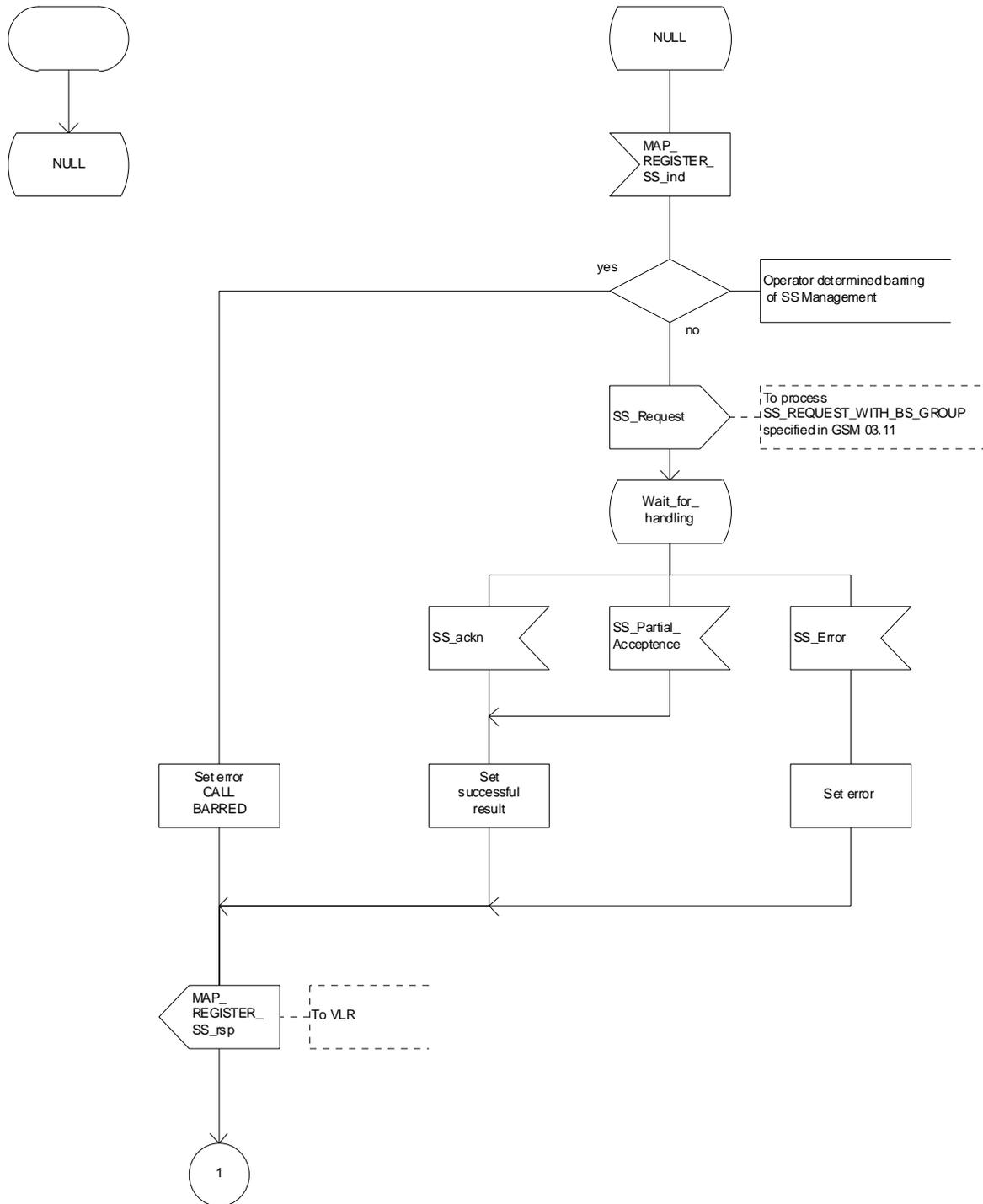
Figure 22.2.4/1 (sheet 1 of 2): Procedure SS\_Register\_HLR
