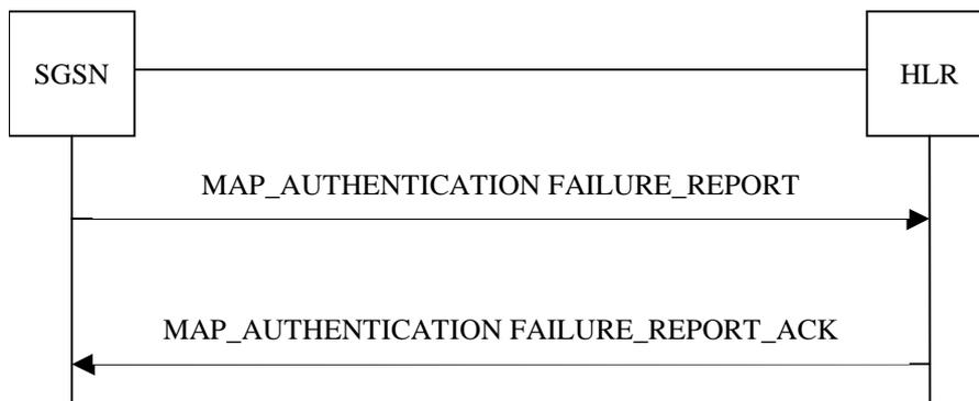
**Figure 25.6/7: Message Flows to Authentication Failure Report**
