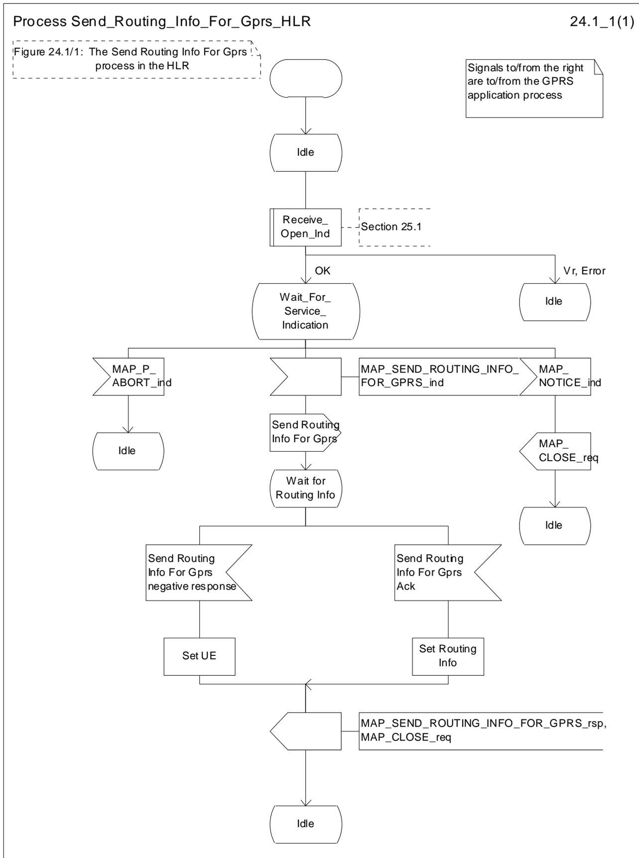
Figure 24.1/1: Process Send Routing Info For Gprs\_HLR
