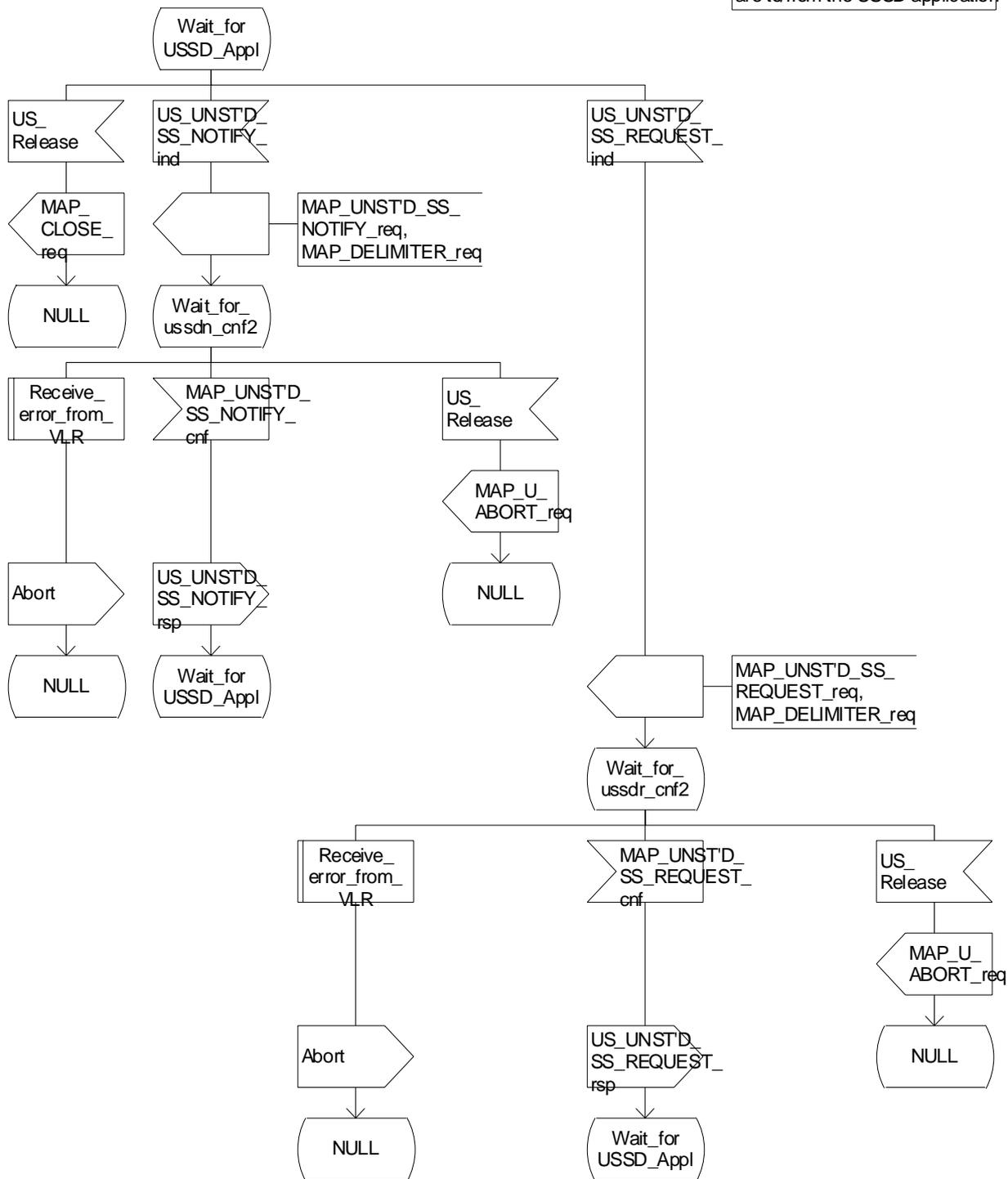
Figure 22.10.4/1 (sheet 5 of 5): Procedure NI\_USSD\_HLR
