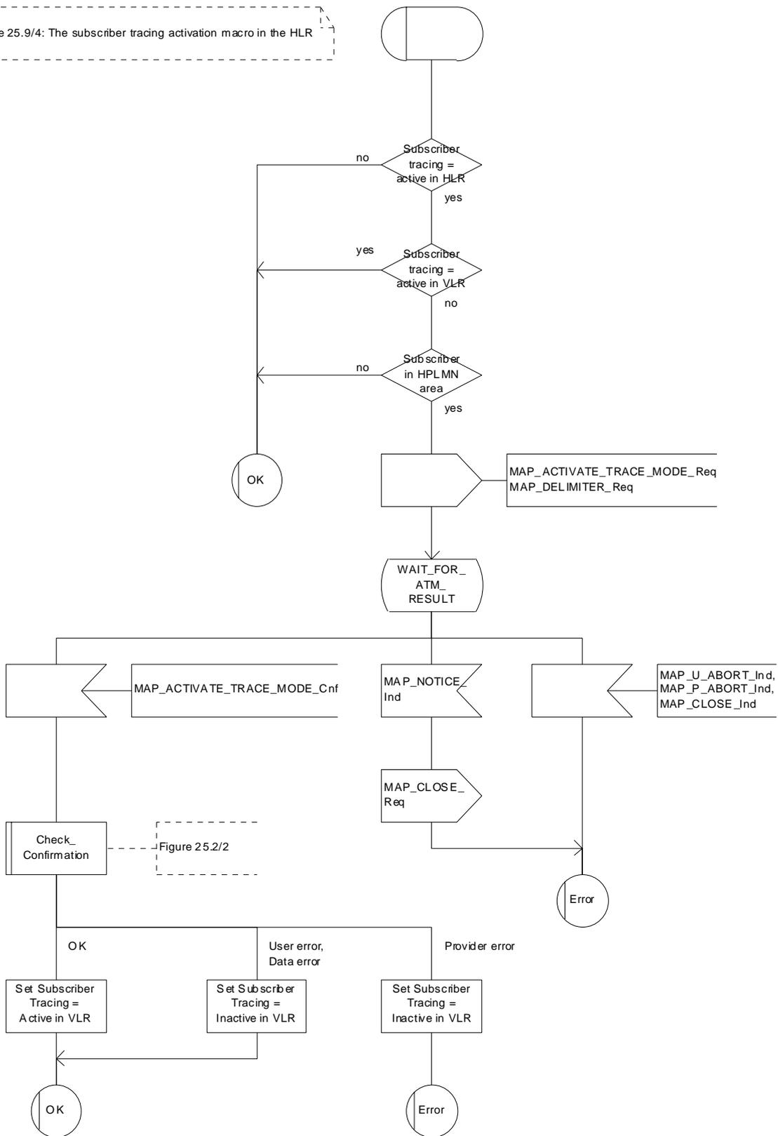
Figure 25.9/4: Macro Control\_Tracing\_HLR
