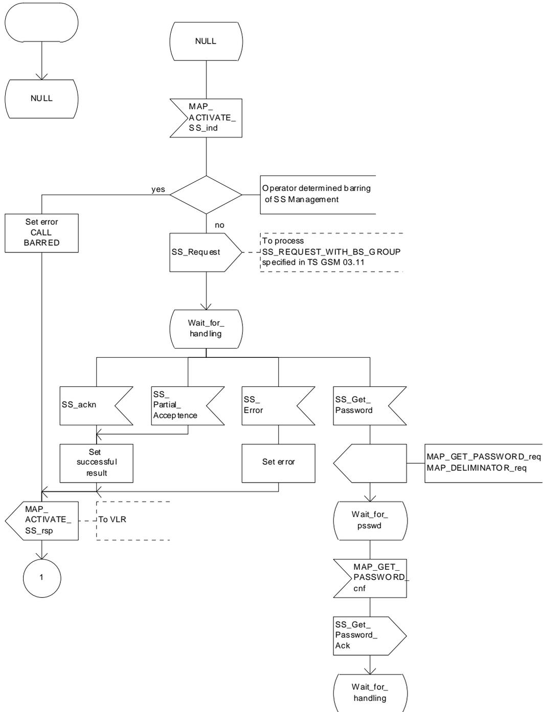
Figure 22.4.4/1 (sheet 1 of 2): Procedure Activate\_SS\_HLR
