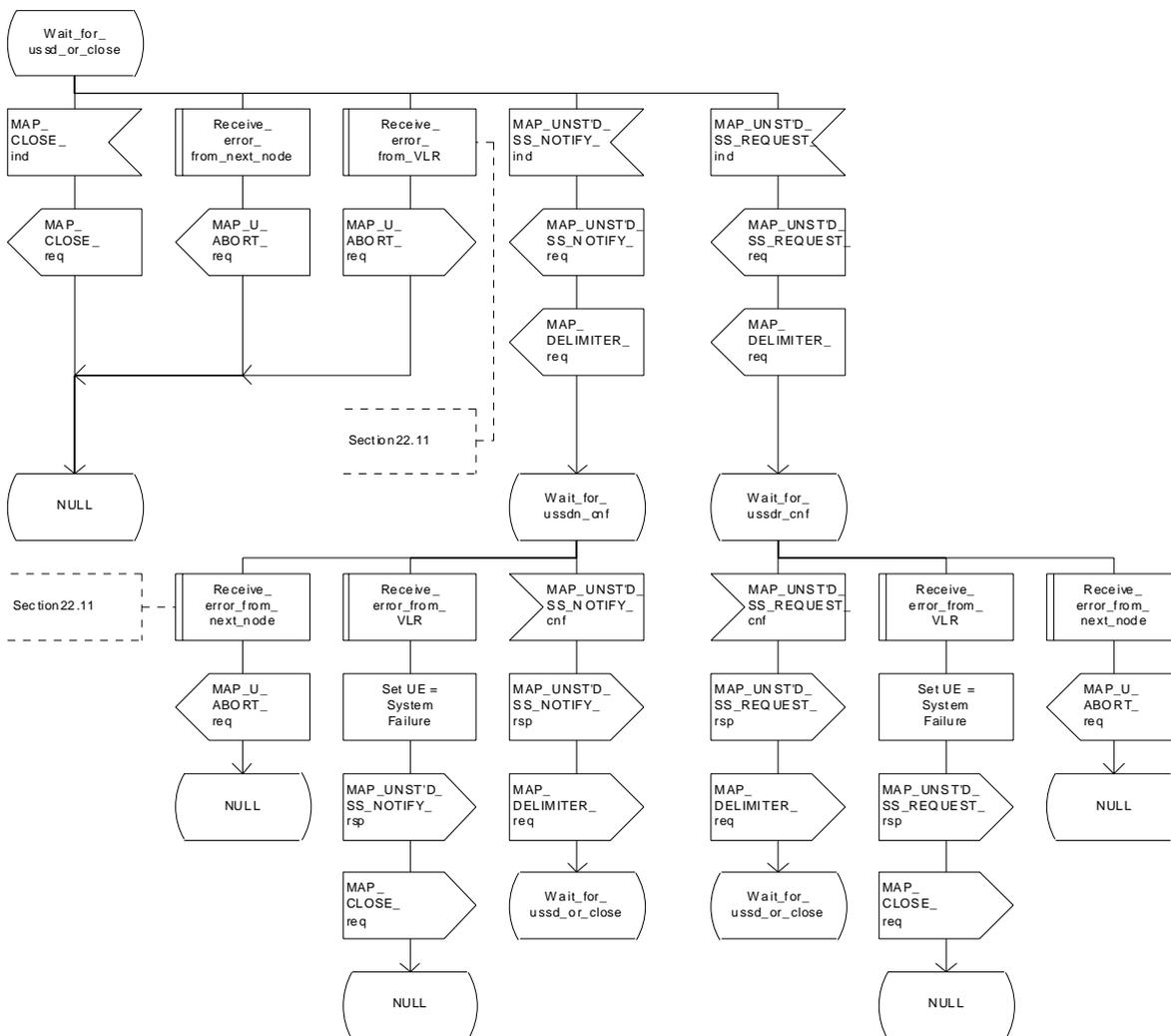
Figure 22.10.4/1 (sheet 3 of 5): Procedure NI\_USSD\_HLR
