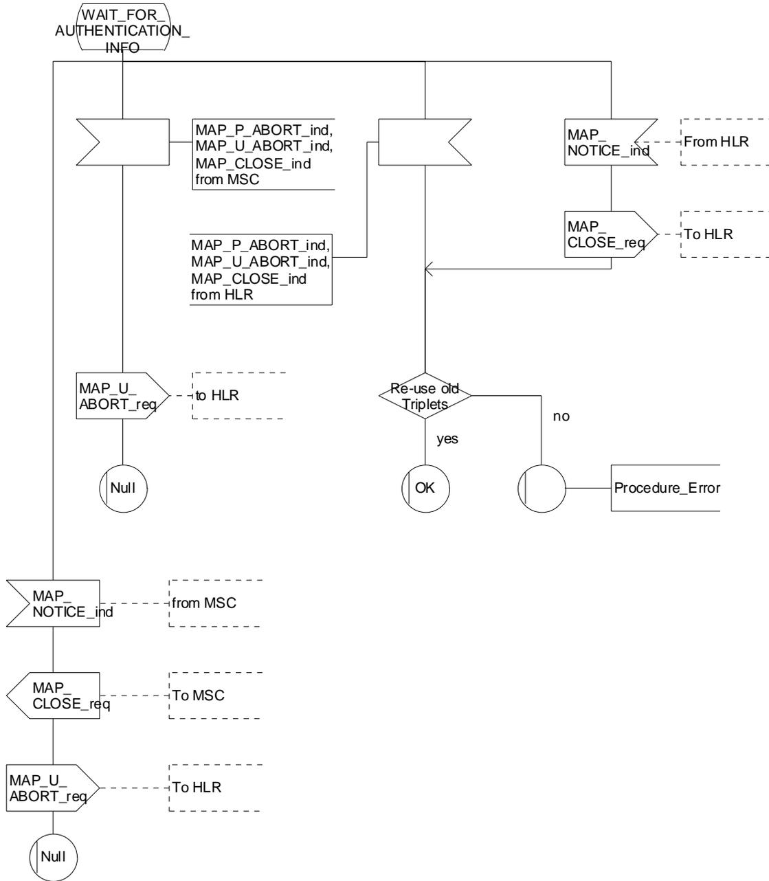
Figure 25.5/4 (sheet 3 of 3): Macro Obtain\_Authent\_Para\_VLR
