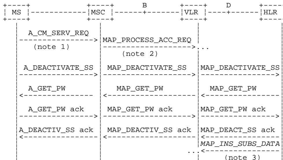
Figure 22.5.1/1: Interfaces and services for supplementary service deactivation
