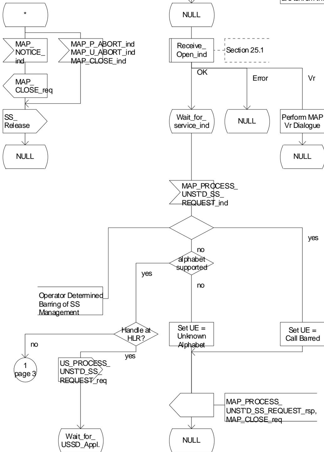
Figure 22.9.4/1 (sheet 1 of 4): Procedure MI\_USSD\_HLR
