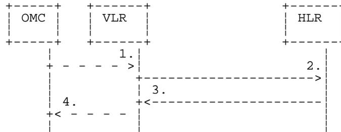
**Figure 20.4/1: The subscriber identity procedure**
