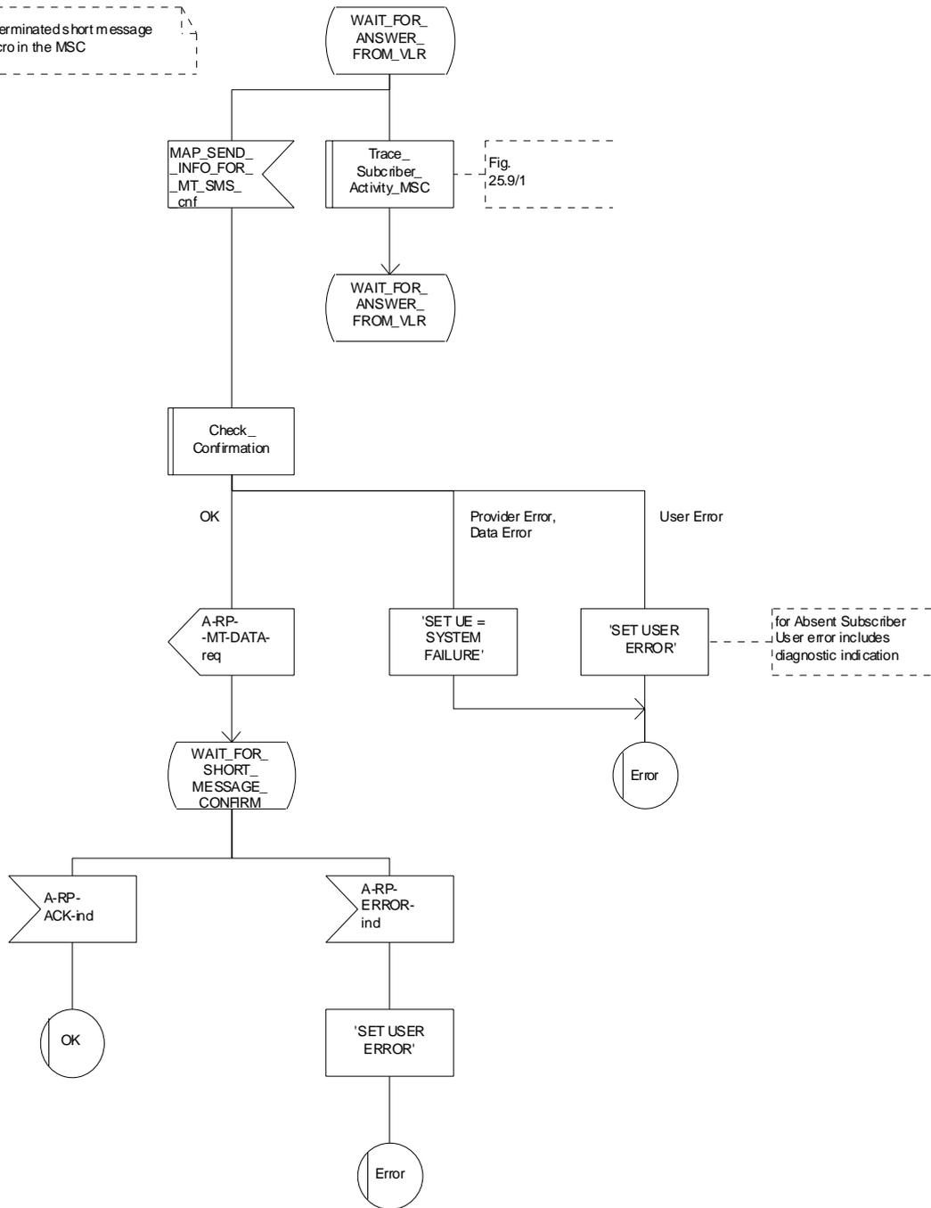
Figure 23.3/4 (sheet 2 of 3): Macro MT\_SM\_Transfer\_MSC
