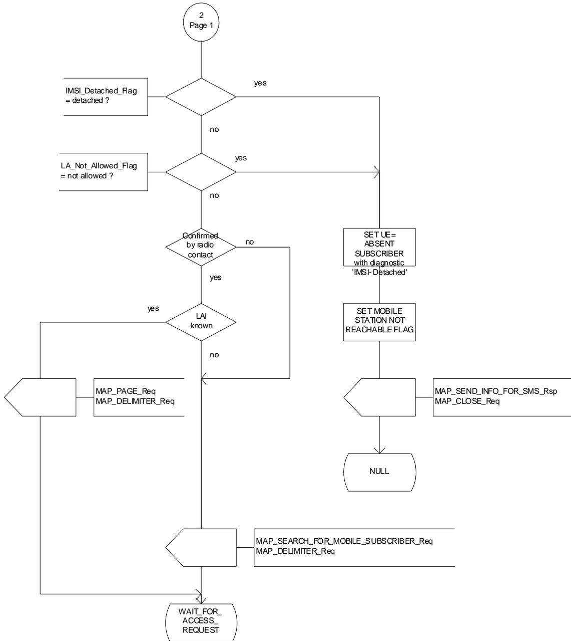
Figure 23.3/5 (sheet 2 of 3): Process MT\_SM\_VLR
