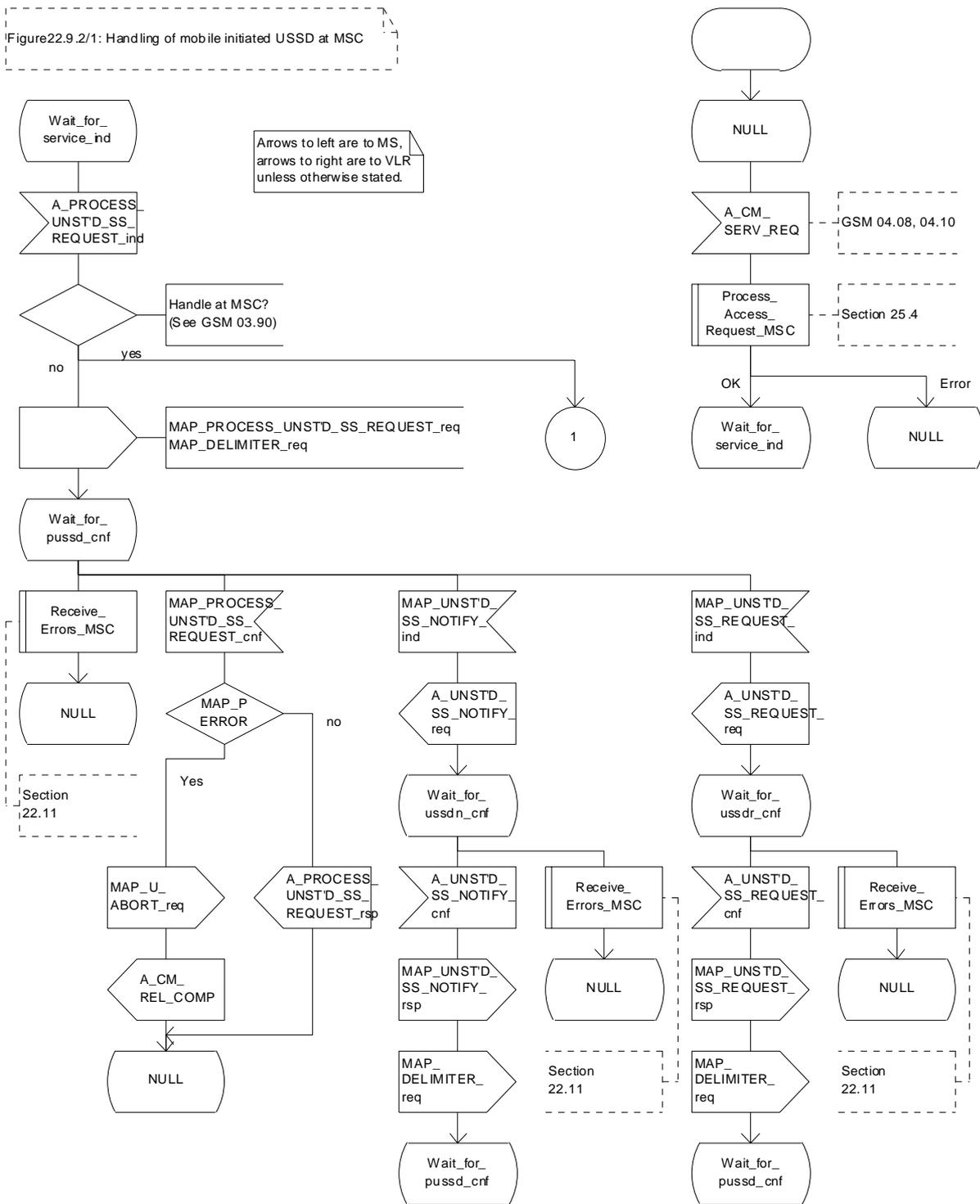
Figure 22.9.2/1 (sheet 1 of 2): Procedure MI\_USSD\_MSC
