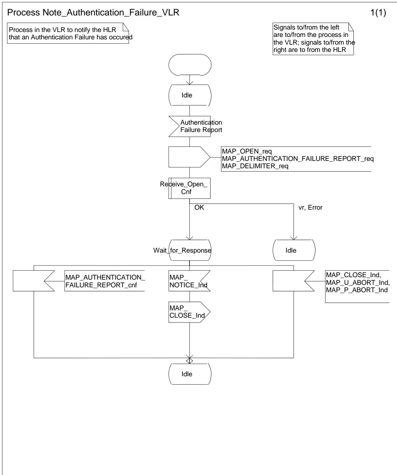
Figure 25.6/8: Process Note\_Authentication\_Failure\_VLR
