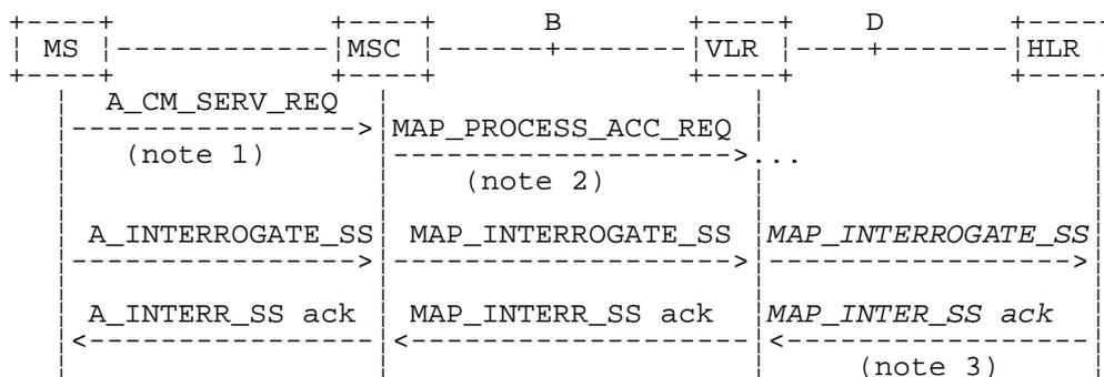
**Figure 22.6.1/1: Interfaces and services for supplementary service interrogation**
