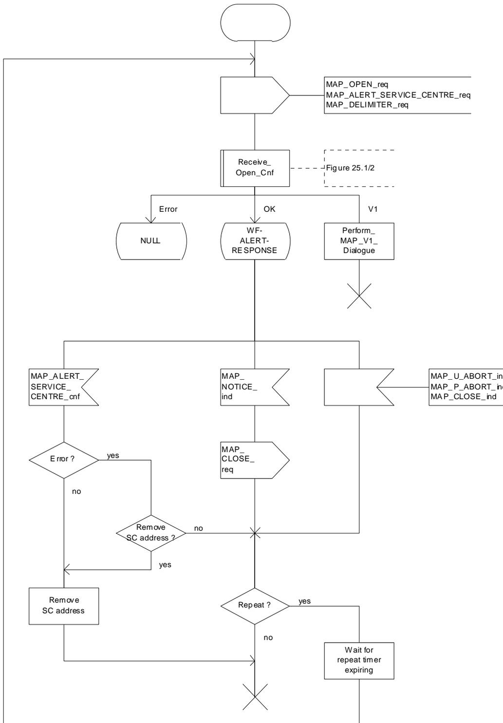
Figure 25.10/3: Process Alert\_Service\_Centre\_HLR
