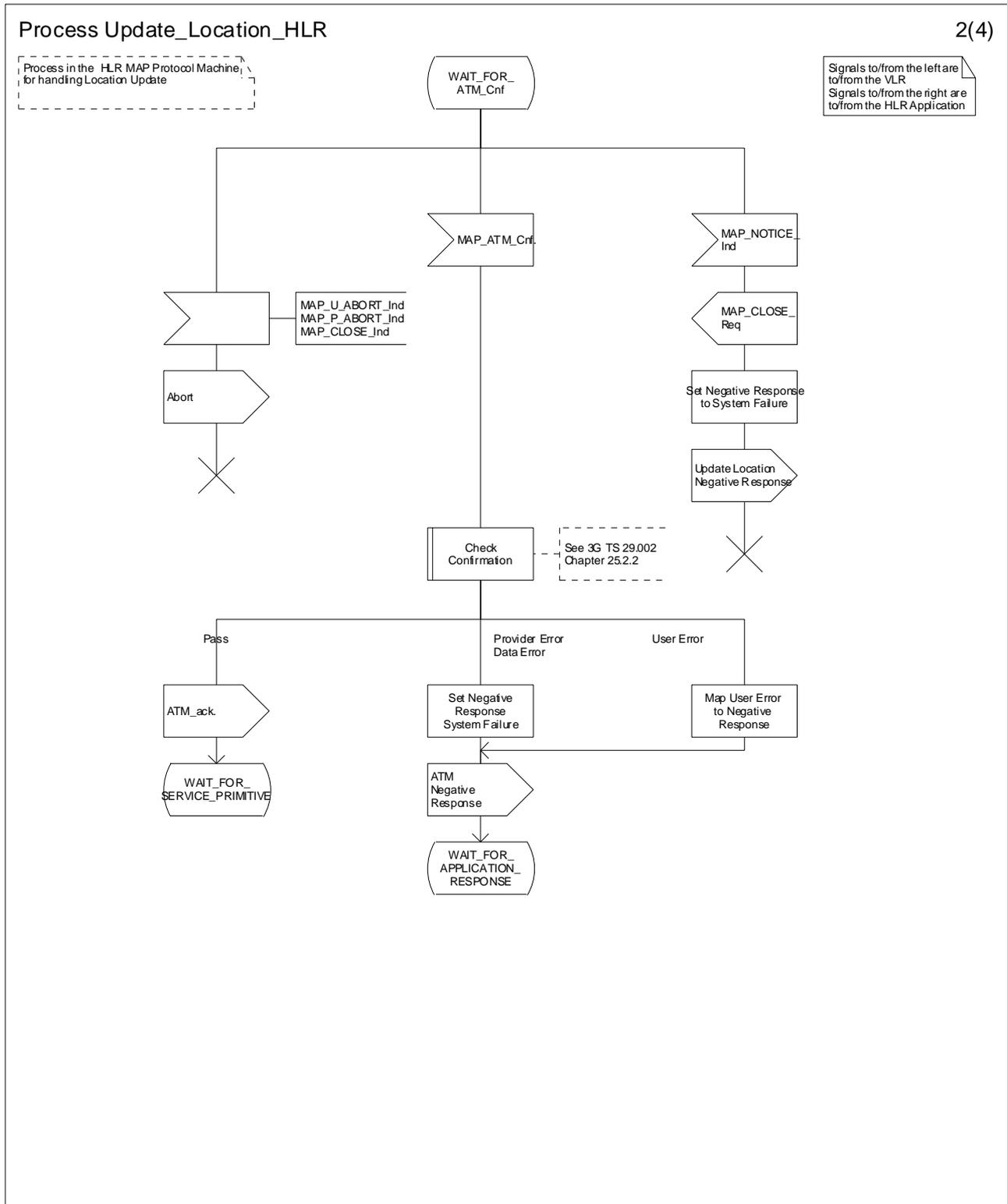
Figure 19.1.1/9 (sheet 2 of 4): Process Update\_Location\_HLR
