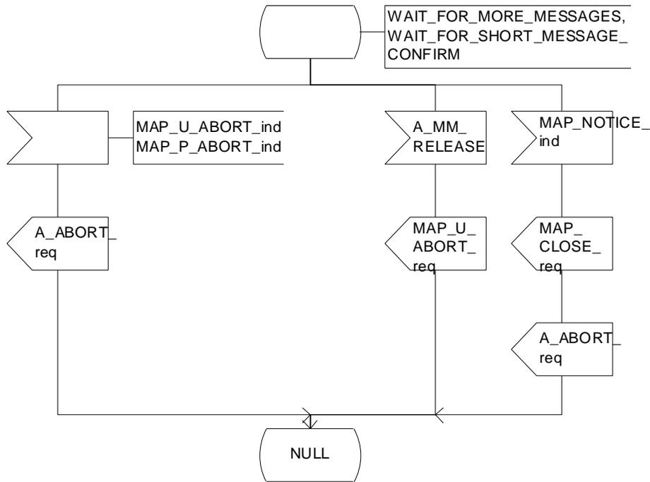
Figure 23.3/3 (sheet 3 of 3): Procedure MTSM\_VMSC
