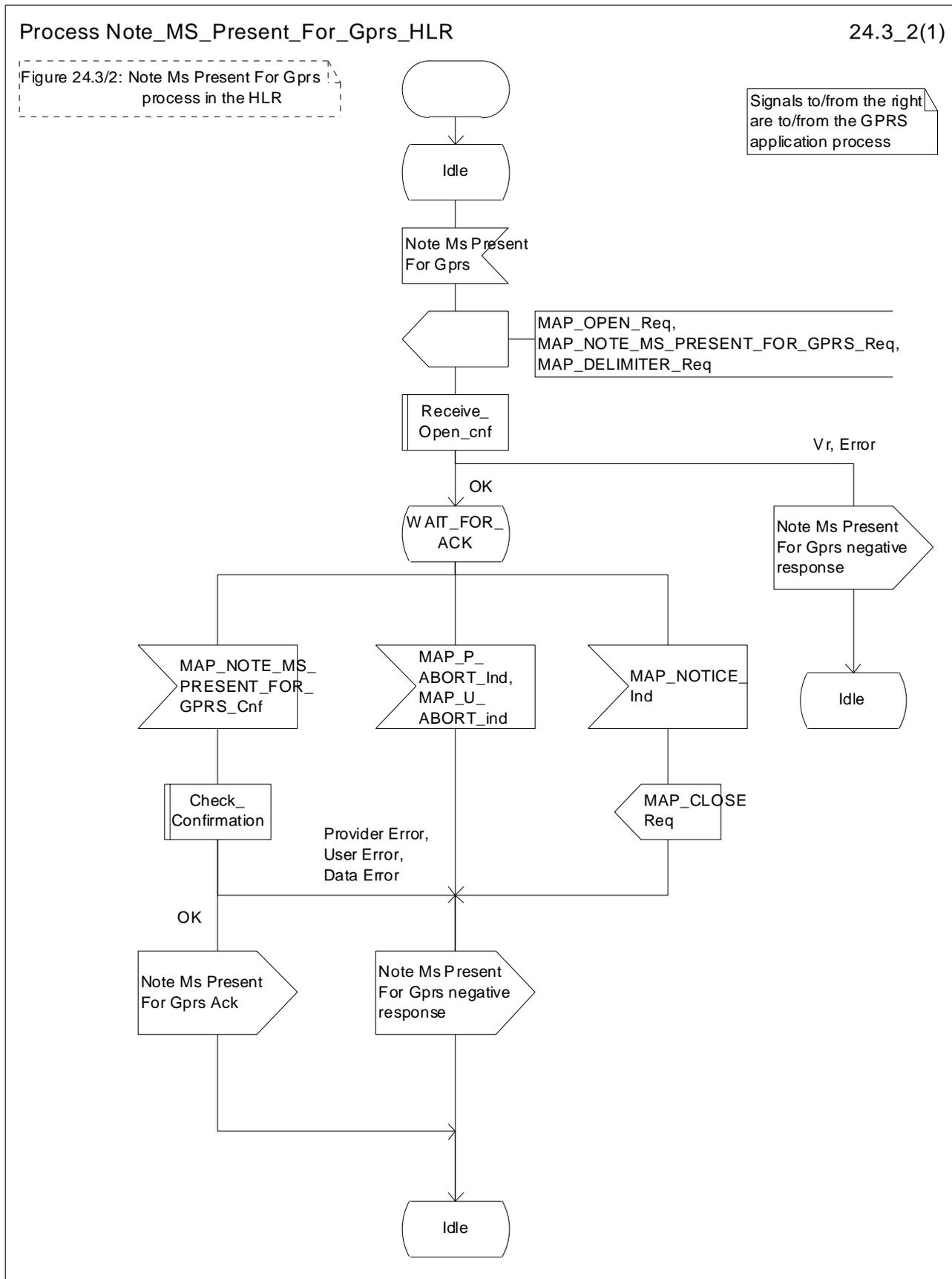
Figure 24.3/2: Process Note\_Ms\_Present\_For\_Gprs\_HLR
