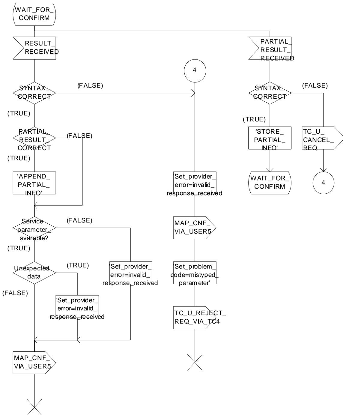
Figure 16.2/7 (sheet 2 of 4): Process REQUESTING\_MAP\_SSM
