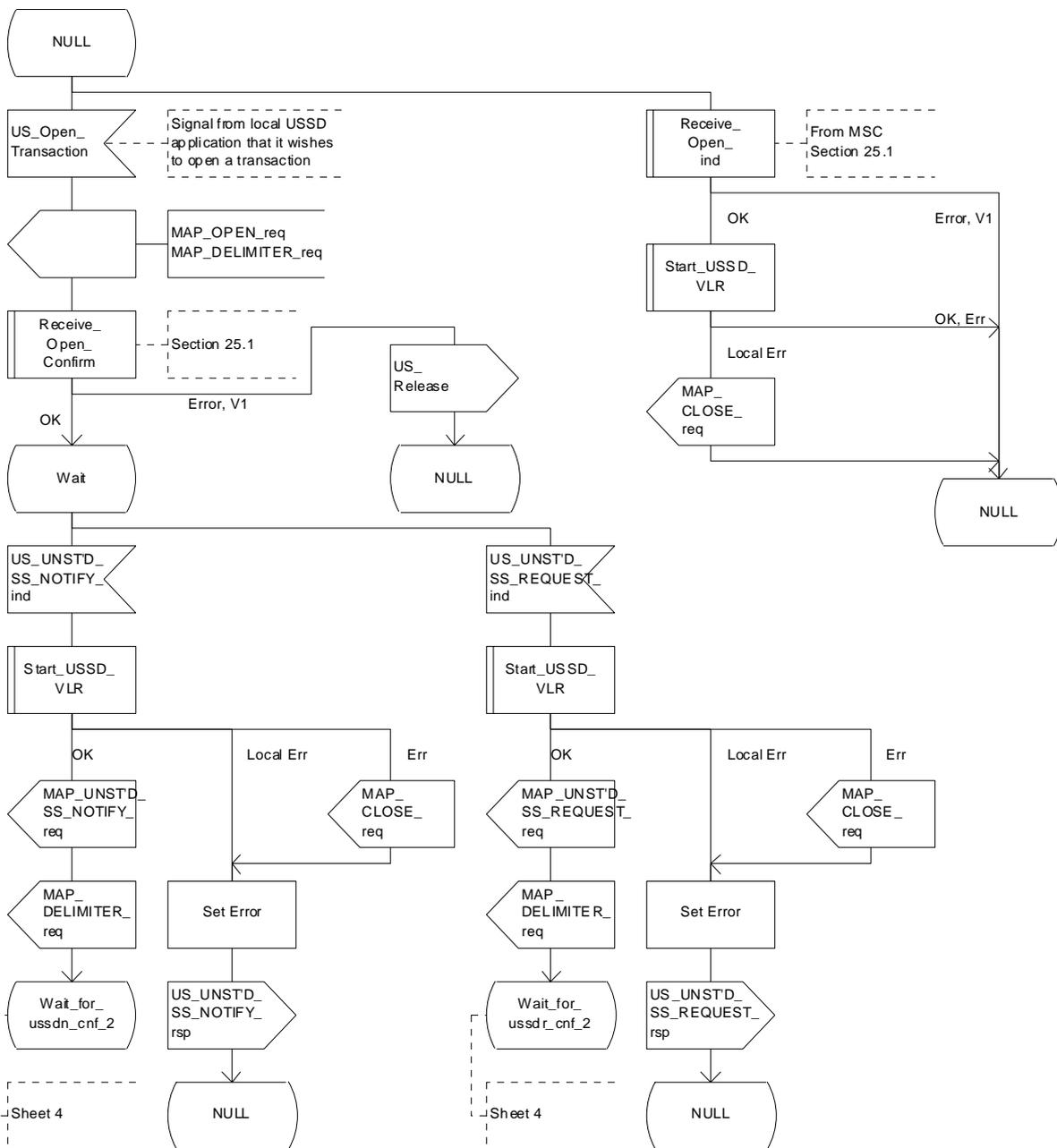
Figure 22.10.3/1 (sheet 3 of 4): Procedure NI\_USSD\_VLR
