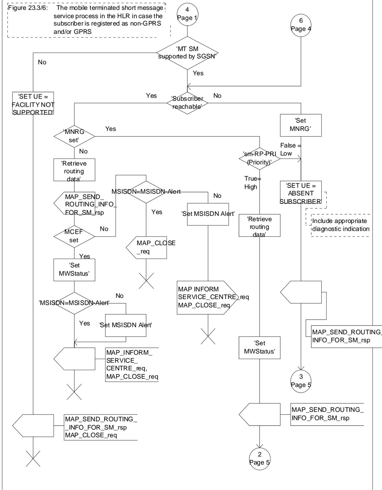
Figure 23.3/6 (sheet 3 of 5): Process Mobile\_terminated\_SM\_HLR
