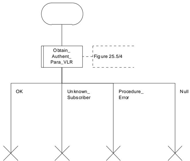
Figure 25.5/3: Process Obtain\_Authentication\_Sets\_VLR
