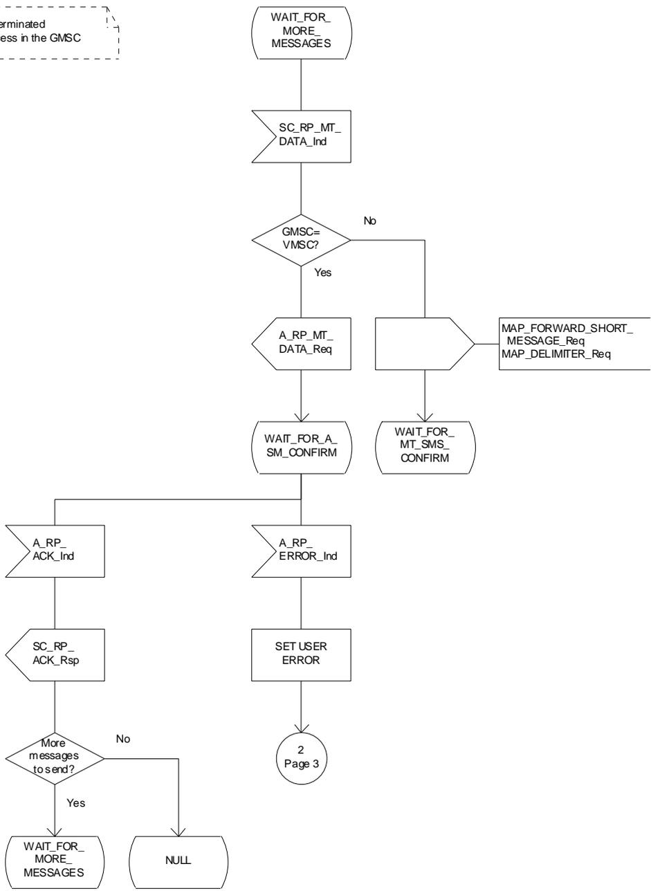
Figure 23.3/7 (sheet 4 of 6): Procedure\_MT\_SM\_GMSC
