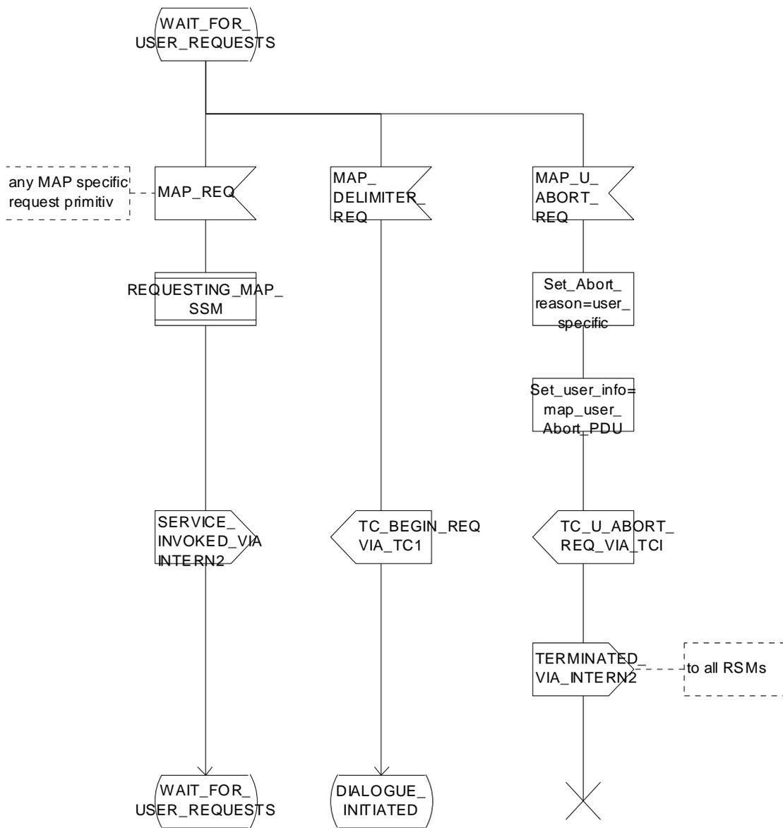
Figure 16.2/3 (sheet 4 of 11): Process MAP\_DSM
