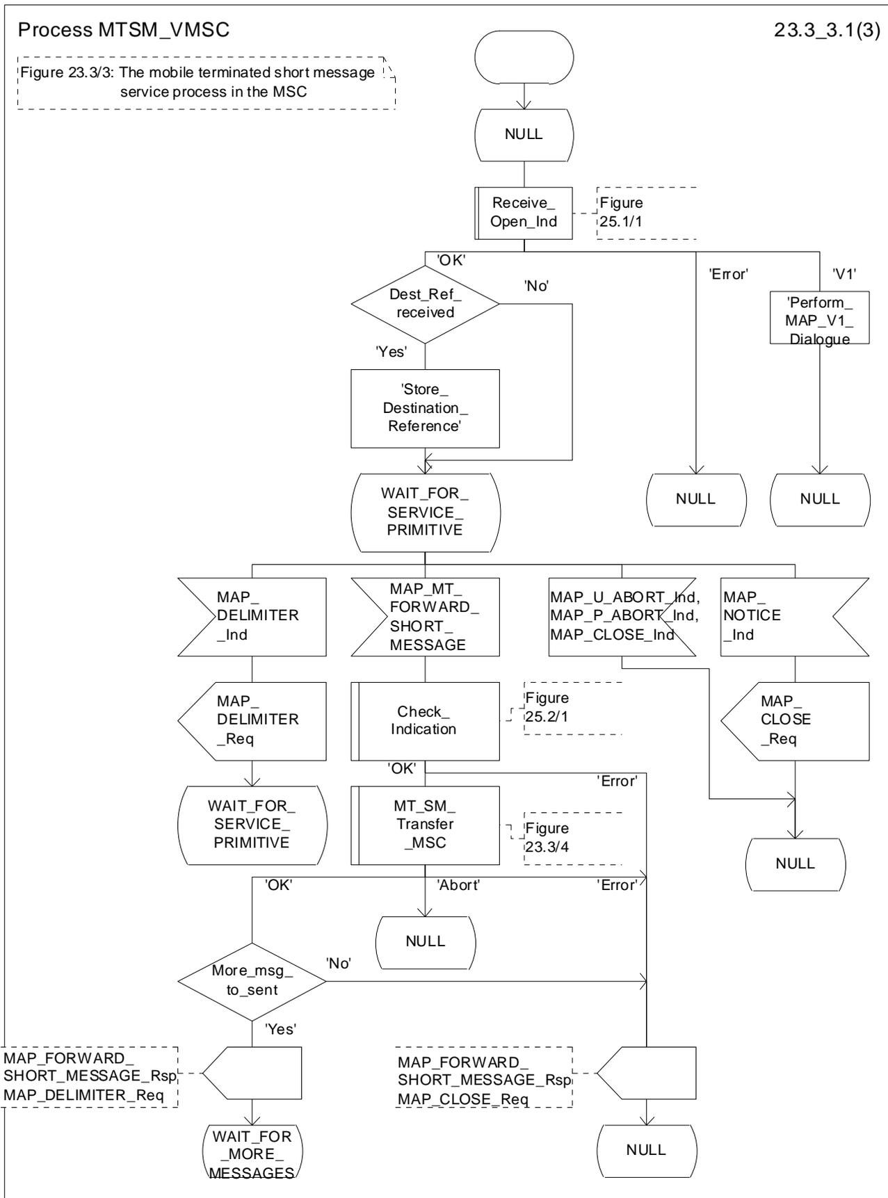
Figure 23.3/3 (sheet 1 of 3): Procedure MTSM\_VMSC
