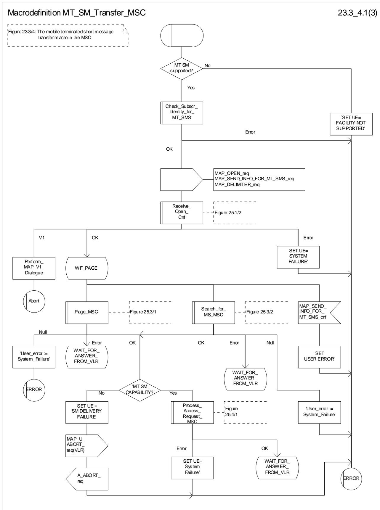
Figure 23.3/4 (sheet 1 of 3): Macro MT\_SM\_Transfer\_MSC
