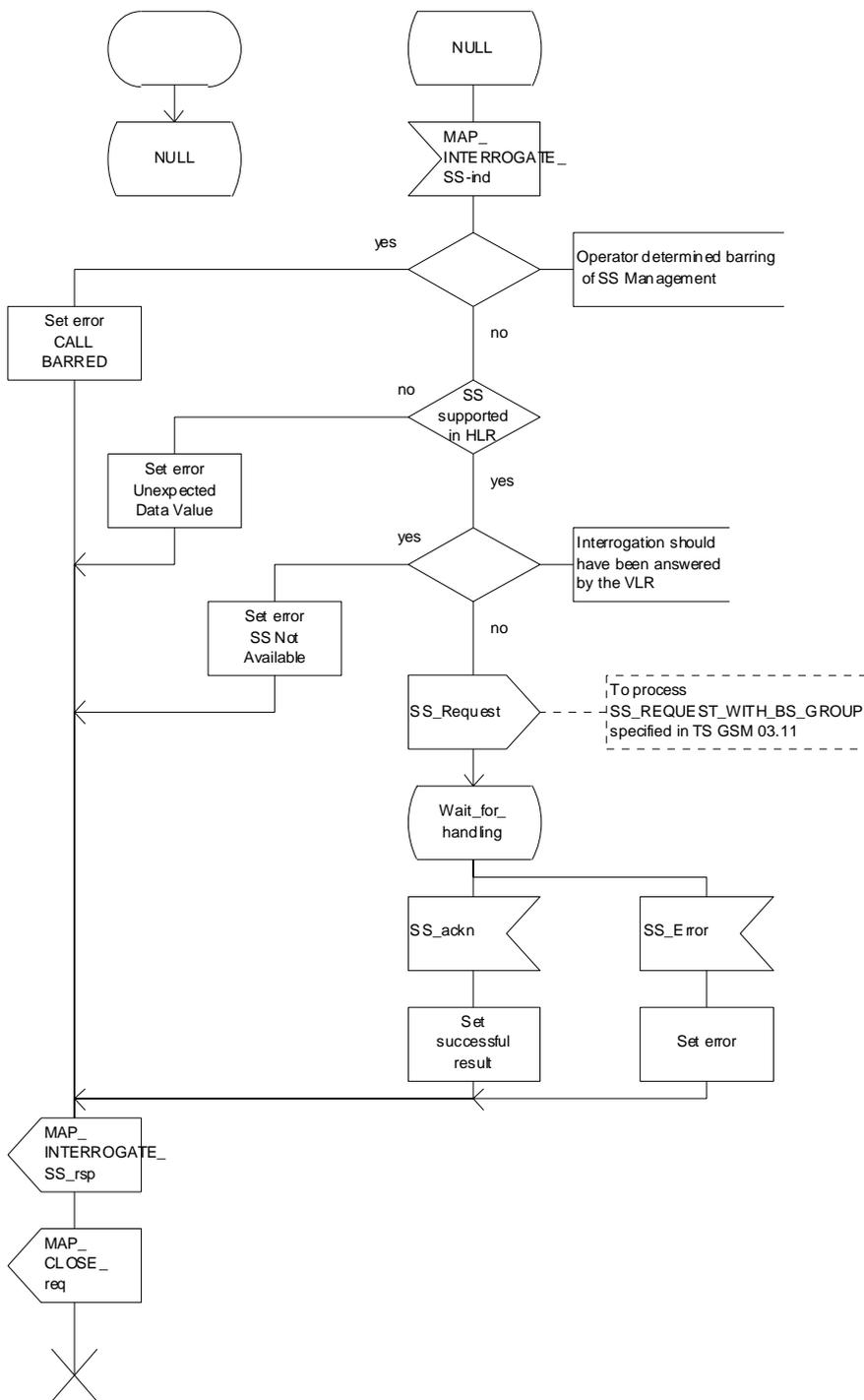
Figure 22.6.4/1: Procedure Interrogate\_SS\_HLR
