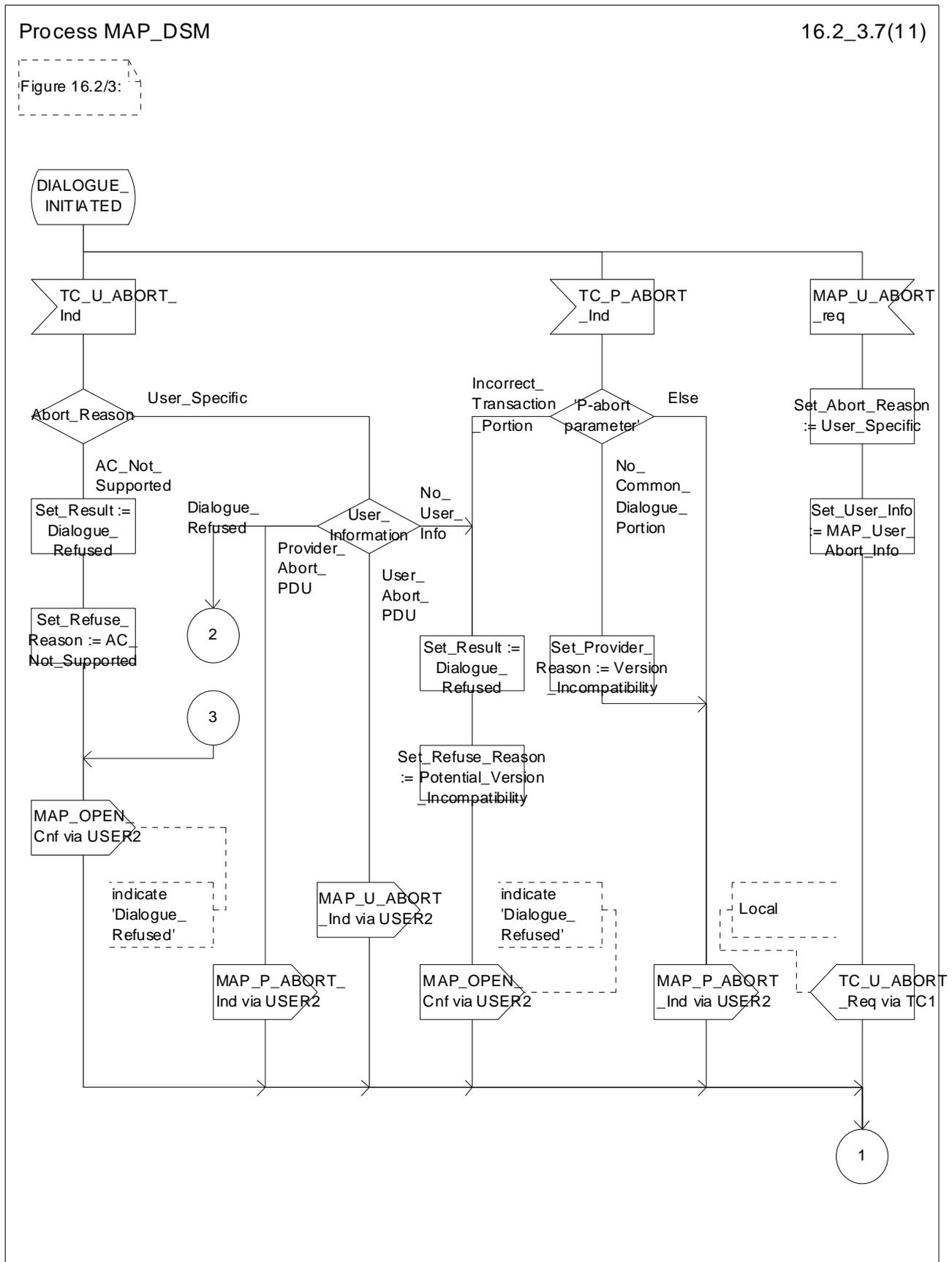
Figure 16.2/3 (sheet 7 of 11): Process MAP\_DSM
