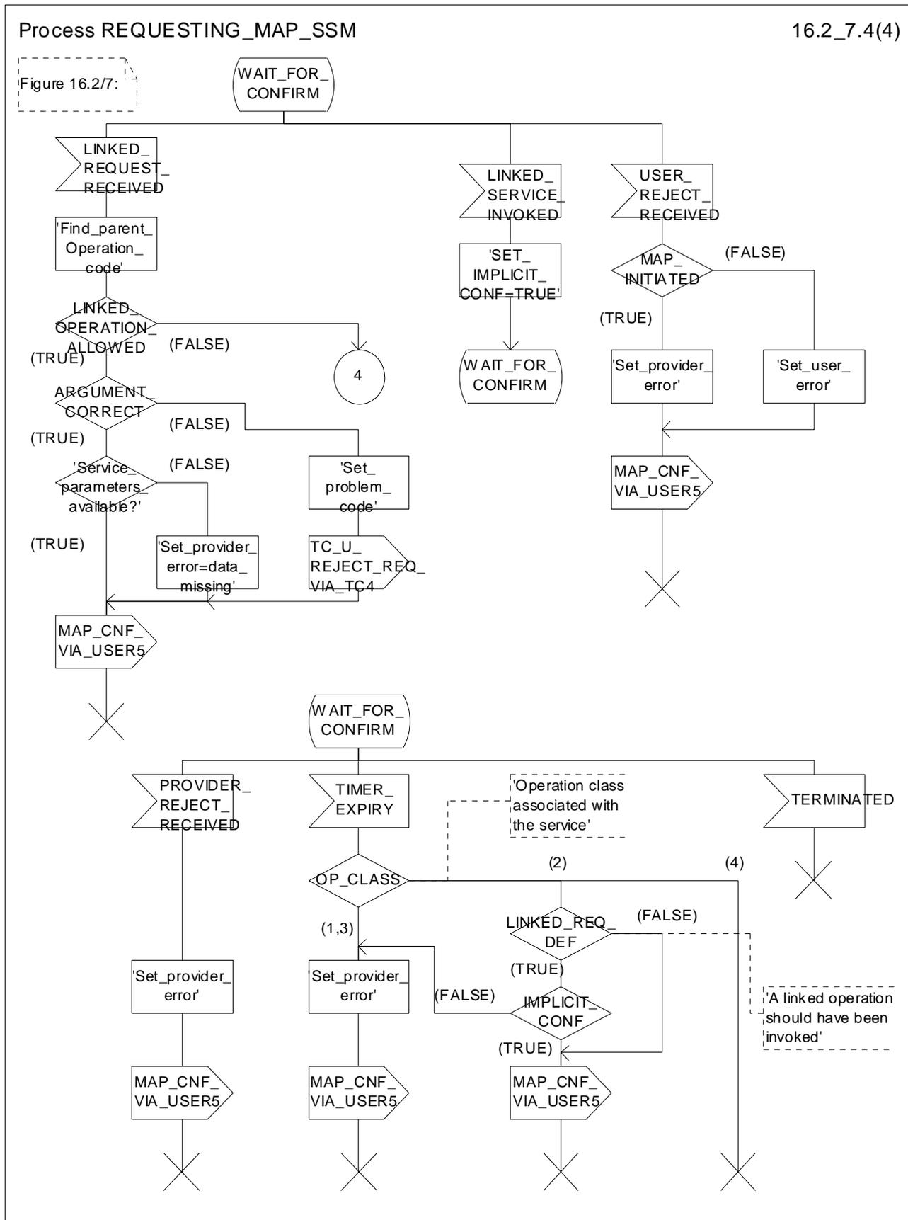
Figure 16.2/7 (sheet 4 of 4): Process REQUESTING\_MAP\_SSM
