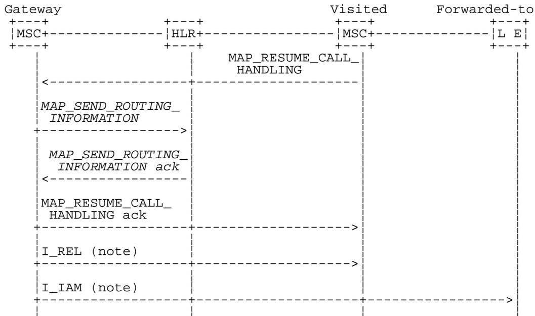
Figure 21.3/1: Message flow for transfer of call handling
