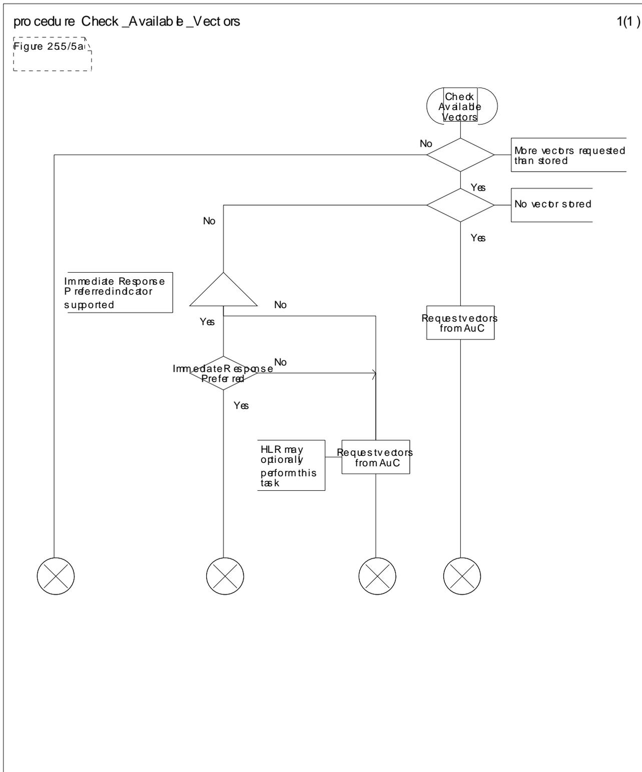
Figure 25.5/6: Procedure Check\_Available\_Vectors
