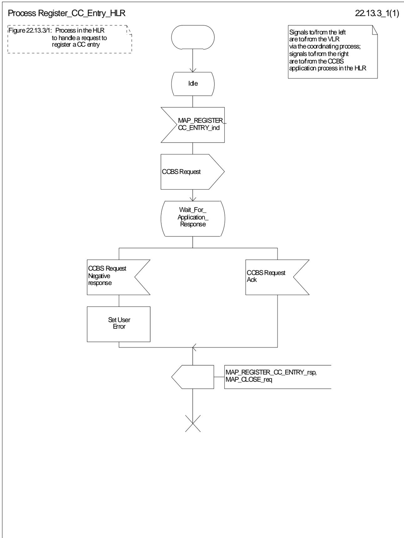
Figure 22.13.3/1: Process Register\_CC\_Entry\_HLR
