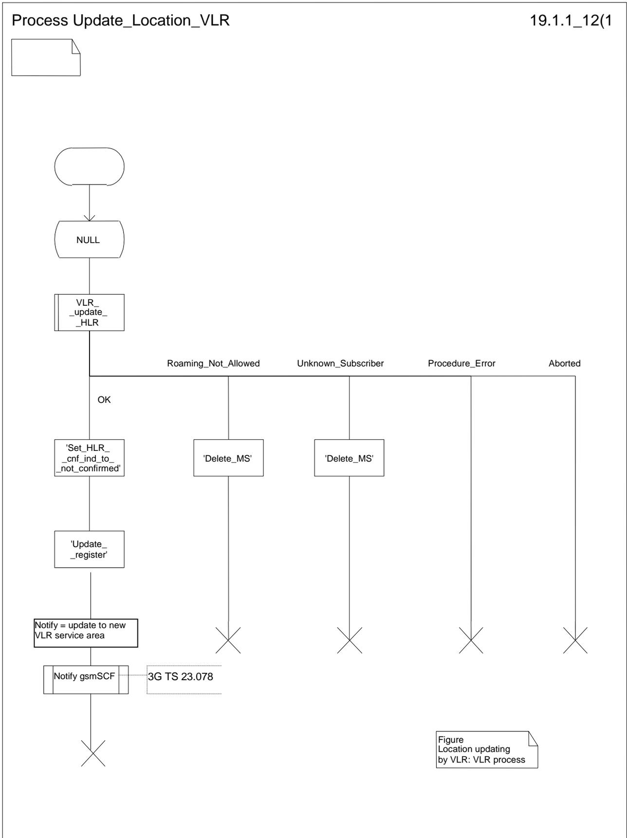
Figure Location updating by VLR: VLR process
