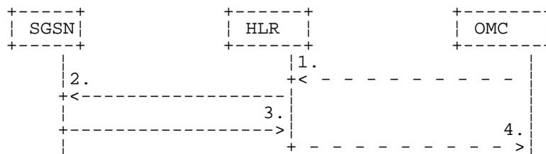
**Figure 20.3/8: Subscriber deletion procedure for GPRS**
