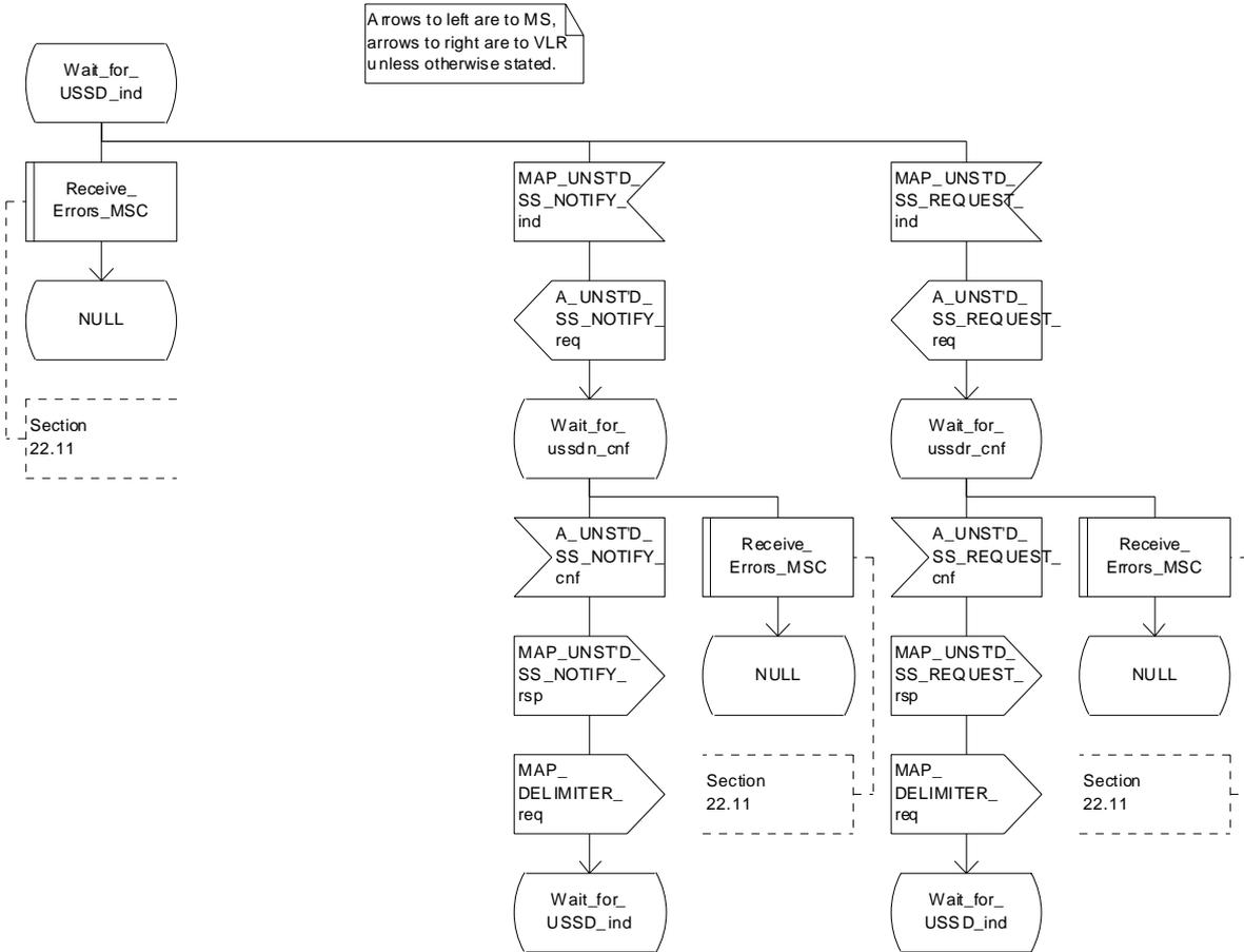
Figure 22.10.2/1 (sheet 2 of 4): Procedure NI\_USSD\_MSC
