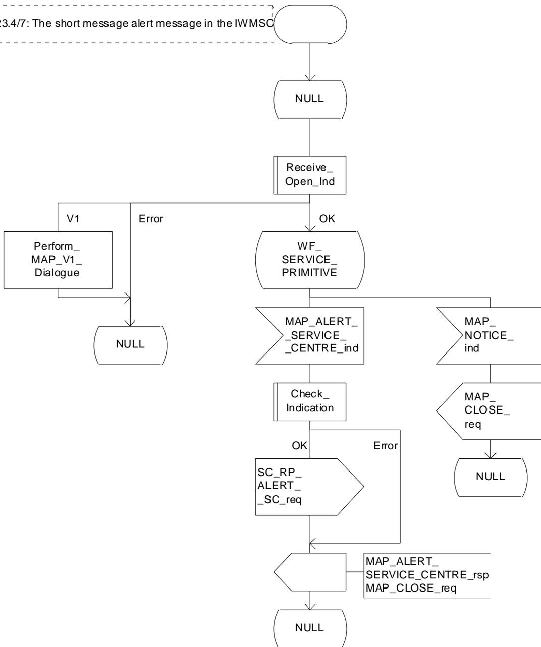
Figure 23.4/7: Process Alert\_SC\_IWMSC
