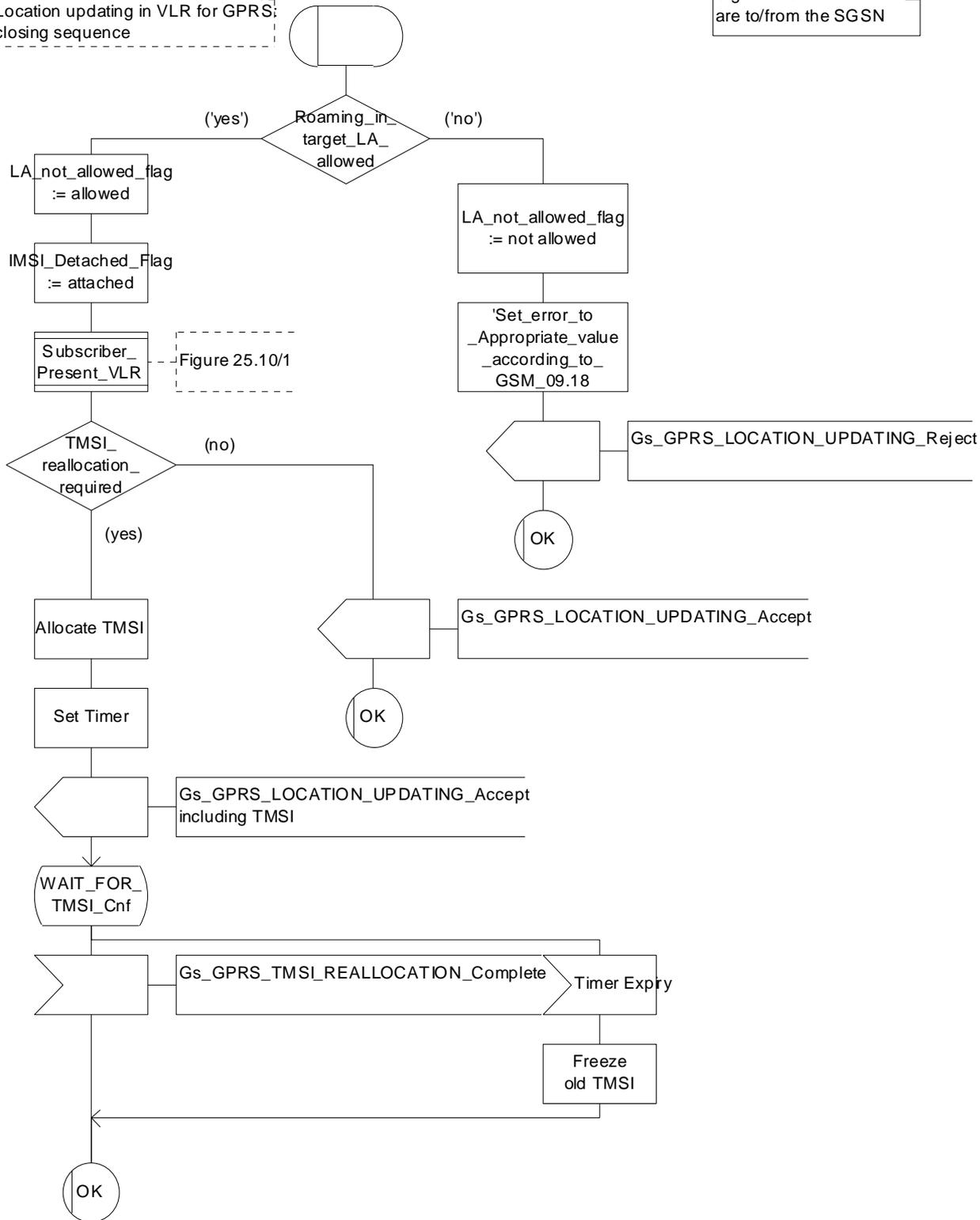
Figure 19.1.1/17: Macro GPRS\_Location\_Update\_Completion\_VLR
