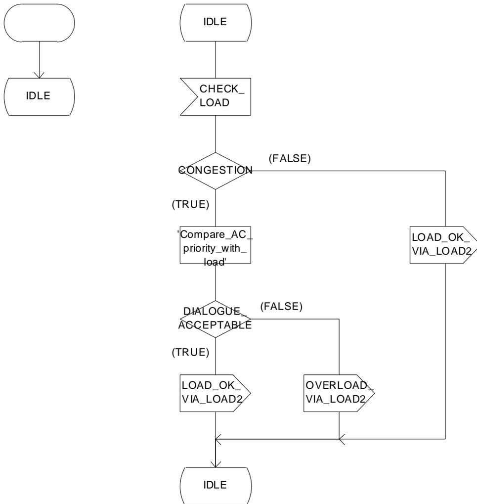
Figure 16.2/5: Process LOAD\_CTRL
