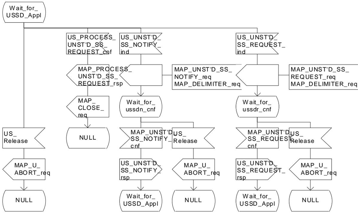
Figure 22.9.4/1 (sheet 2 of 4): Procedure MI\_USSD\_HLR
