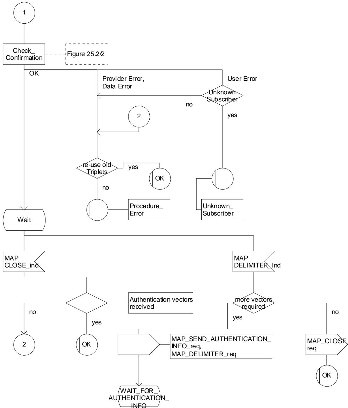
Figure 25.5/4 (sheet 2 of 3): Macro Obtain\_Authent\_Para\_VLR
