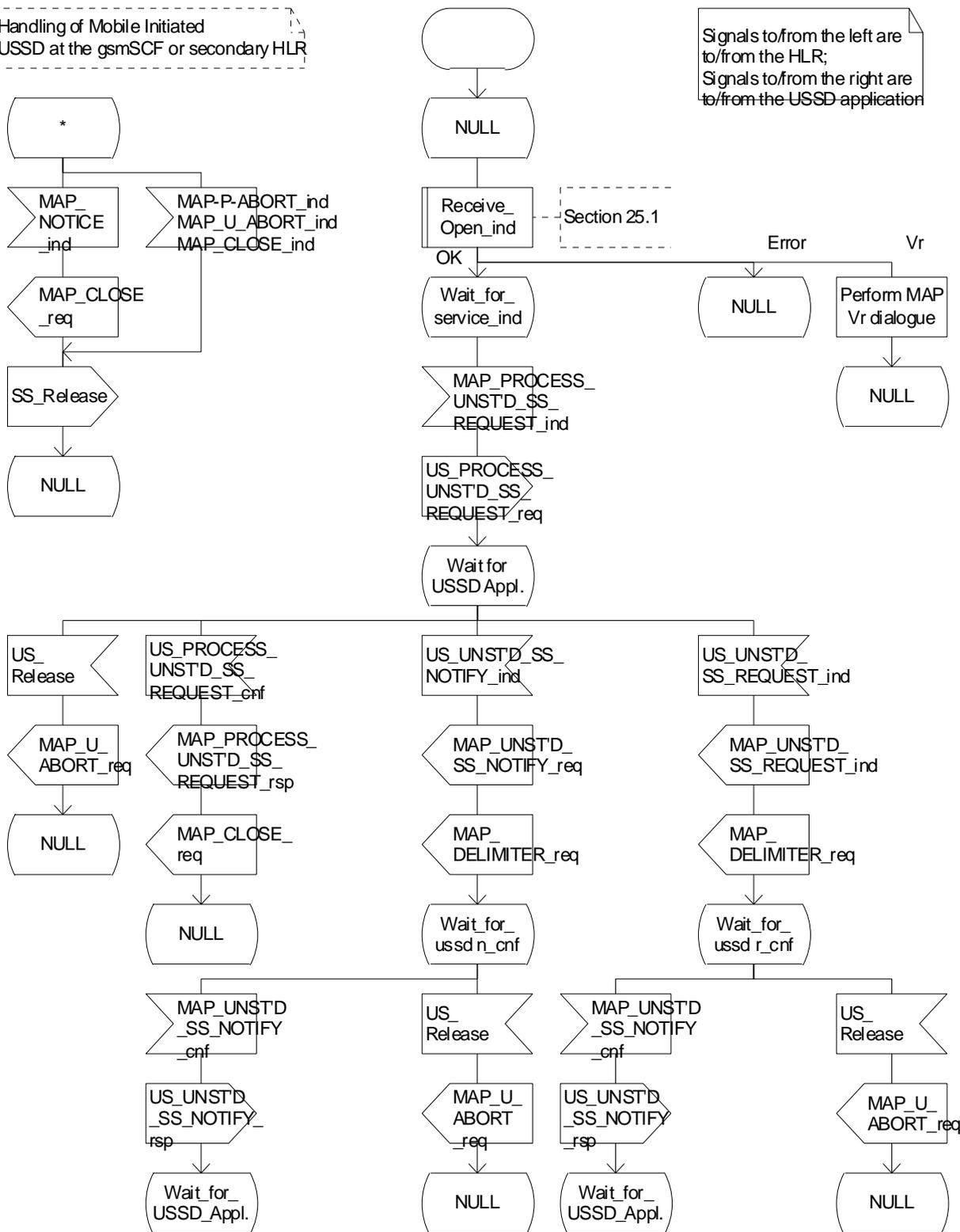
Figure 22.9.5/1 Process MS\_INIT\_USSD\_gsmSCF\_secondary\_HLR
