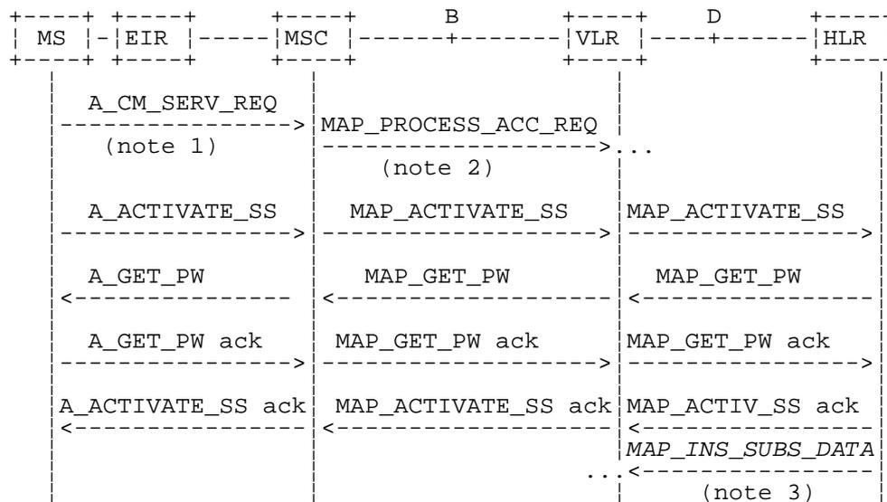
**Figure 22.4.1/1: Interfaces and services for supplementary service activation**
