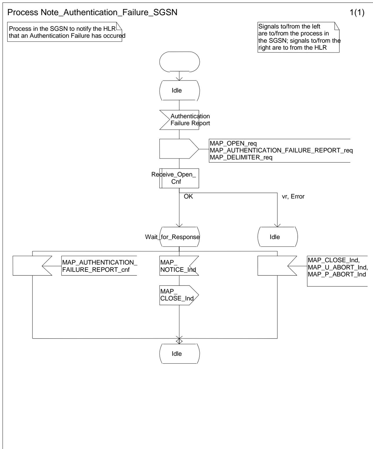
Figure 25.6/9: Process Note\_Authentication\_Failure\_SGSN
