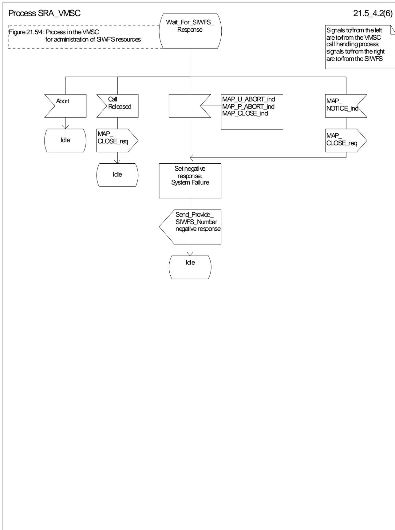
Figure 21.5/4 (sheet 2 of 6): Process SRA\_VMSC
