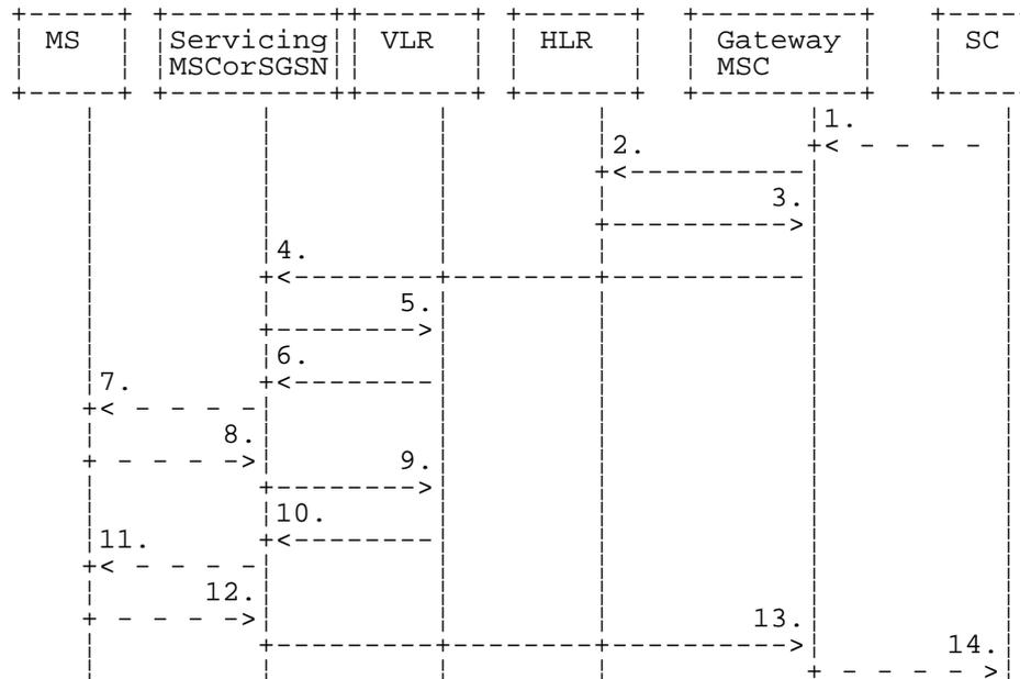
**Figure 23.3/1: Mobile terminated short message service procedures**
