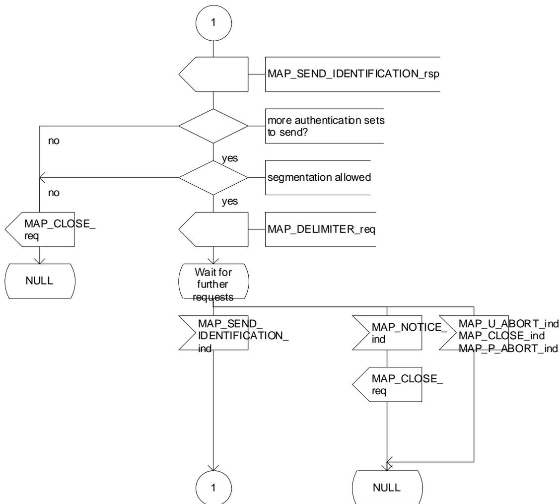
Figure 19.1.1/XX (sheet 2 of 2): Process Send\_Identification\_PVLR
