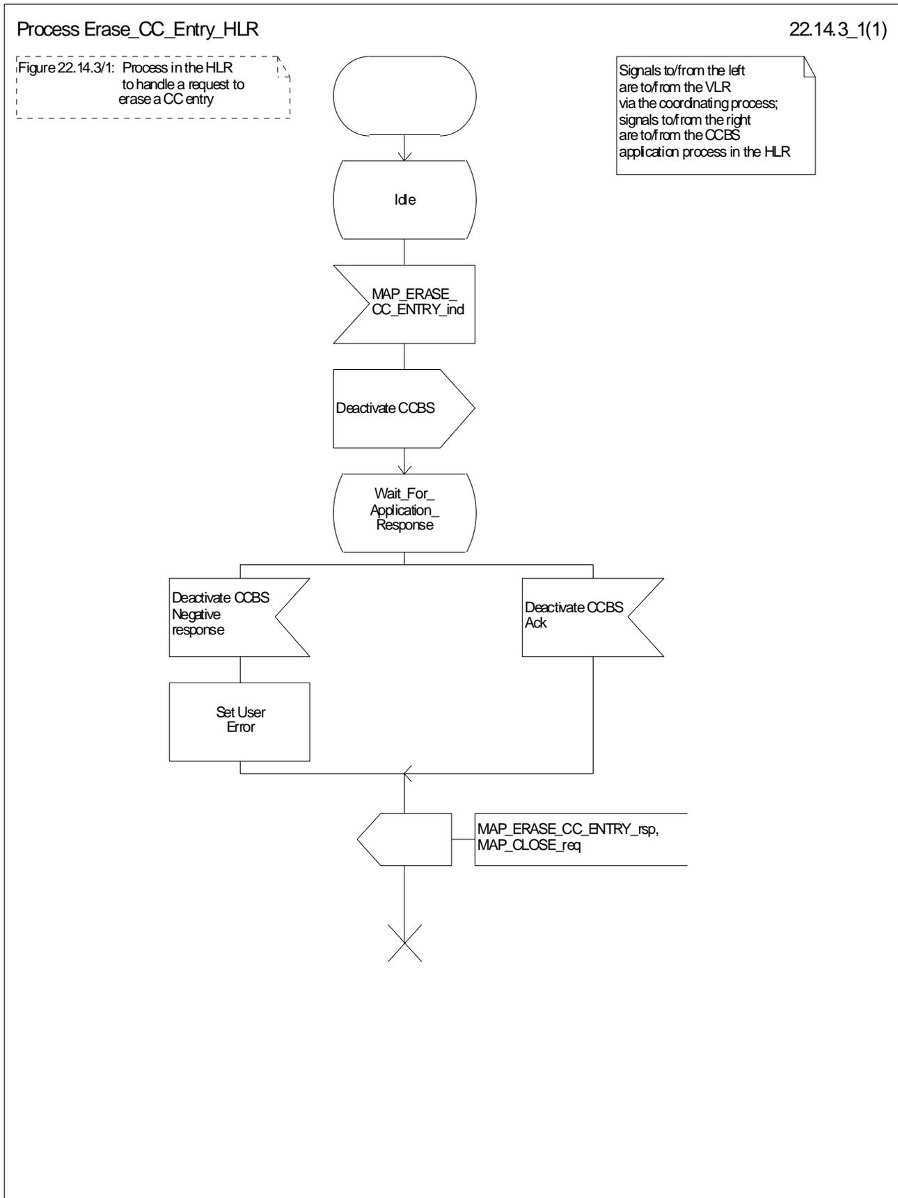
Figure 22.14.3/1: Process Erase\_CC\_Entry\_HLR
