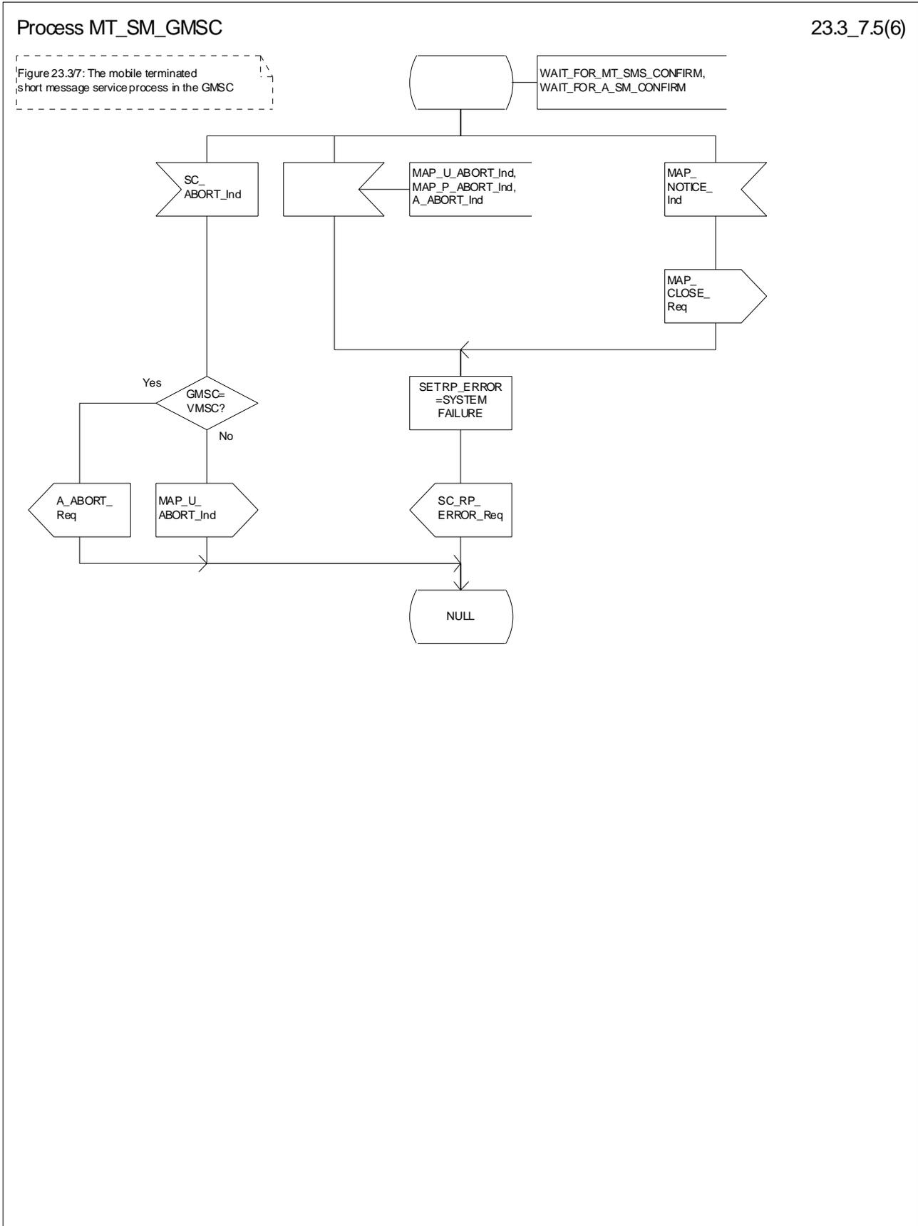
Figure 23.3/7 (sheet 5 to 6): Procedure MT\_SM\_GMSC
