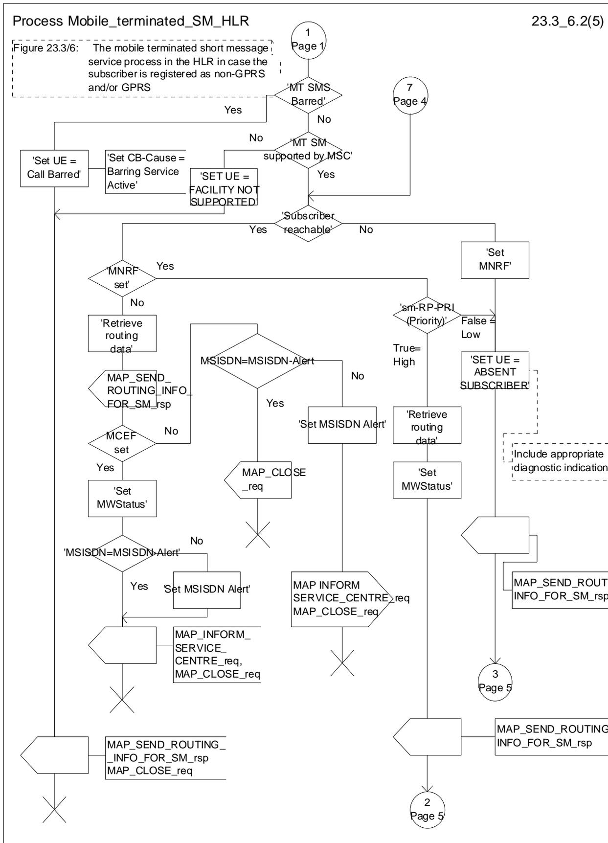
Figure 23.3/6 (sheet 2 of 5): Process Mobile\_terminated\_SM\_HLR
