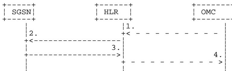
Figure 20.2/13: Subscriber tracing deactivation procedure for GPRS
