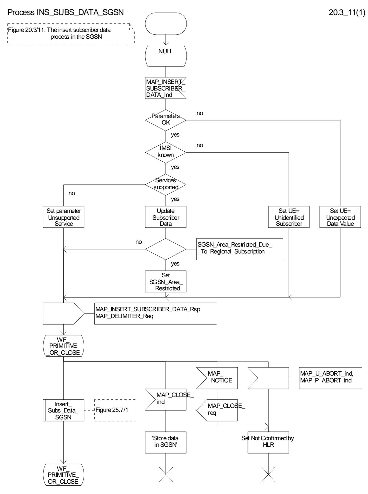
Figure 20.3/11: Process INS\_SUBS\_DATA\_SGSN
