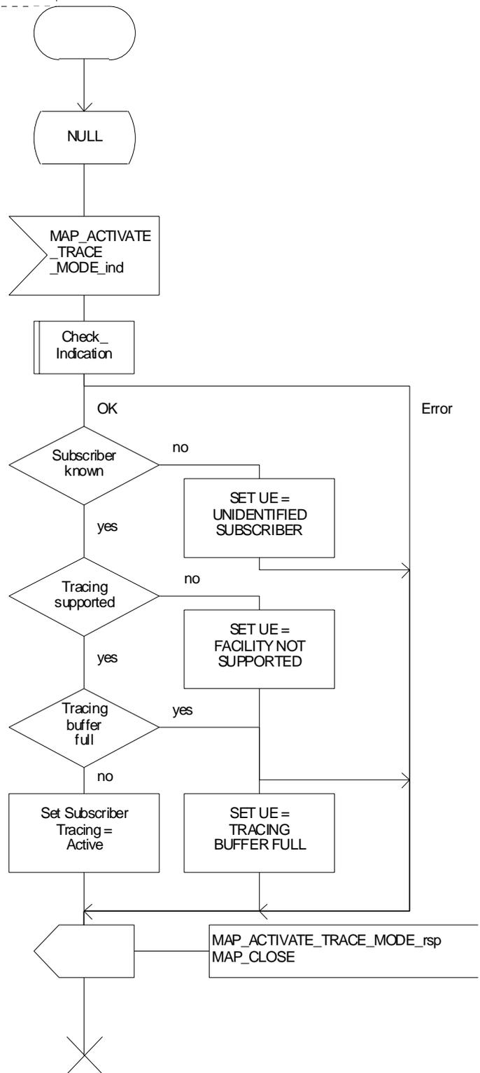
Figure 20.2/16: Process ATM\_SGSN\_Standalone
