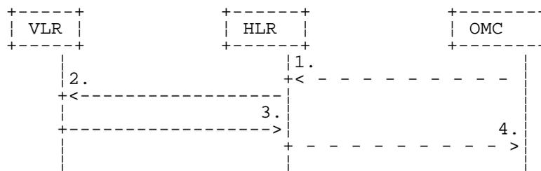
**Figure 20.2/1: Stand alone subscriber tracing activation procedure**
