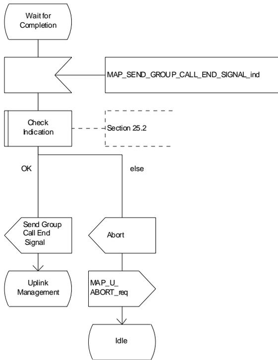
Figure 21.4/2 (sheet 3 of 4): Process ASCI\_Anchor\_MSC
