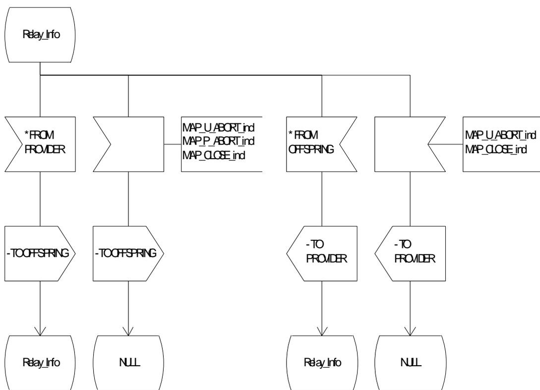
Figure 22.1/3 (sheet 2 of 2): Process SS\_Coordinator\_HLR
