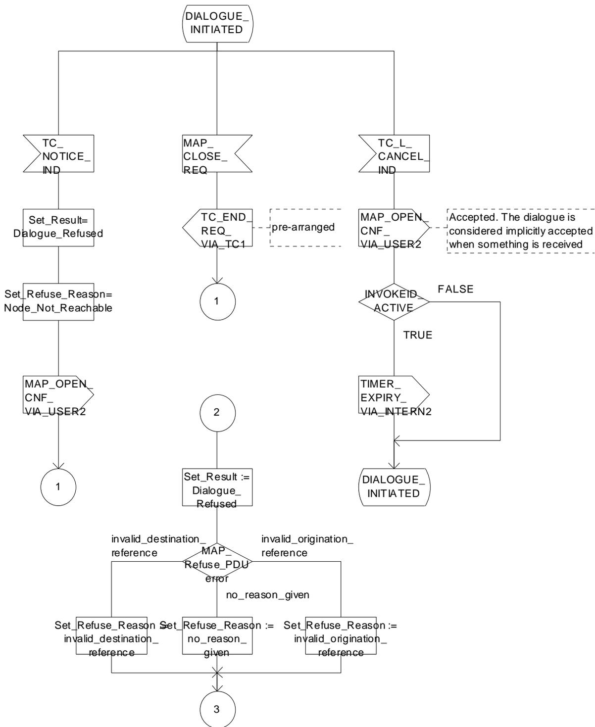
Figure 16.2/3 (sheet 8 of 11): Process MAP\_DSM
