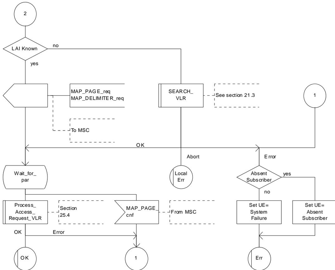
Figure 22.10.3/2 (sheet 2 of 2): Macro Start\_USSD\_VLR
