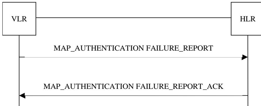
**Figure 25.5/7: Message Flows to Authentication Failure Report**
