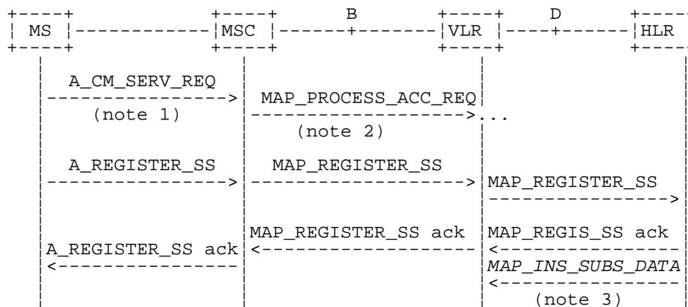
**Figure 22.2.1/1: Interfaces and services for supplementary service registration**
