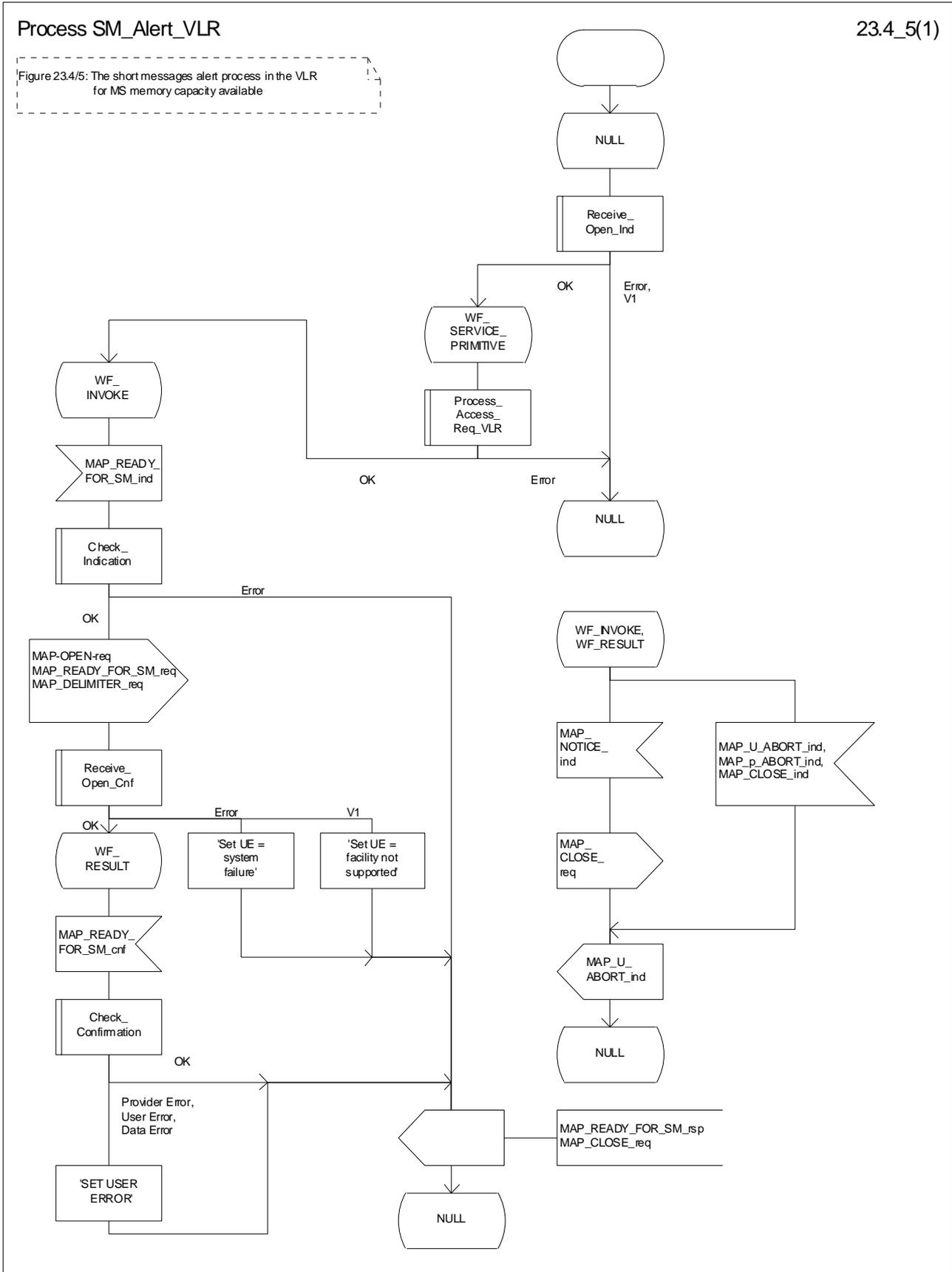
Figure 23.4/5: Procedure SM\_Alert\_VLR
