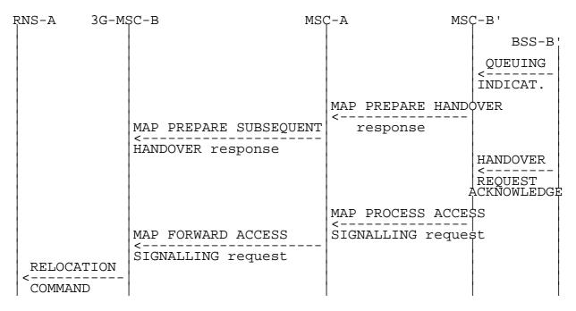
Figure 33: Signalling for Subsequent Inter-MSC Handover to third MSC (MSC-B') execution (Positive outcome)
