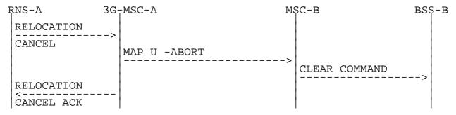
Figure 23: Signalling for Basic Inter-MSC Handover execution (Negative outcomes)
