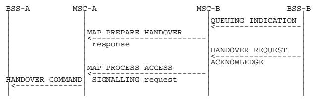
Figure 6: Signalling for Basic Inter-MSC Handover execution (Positive outcomes)
