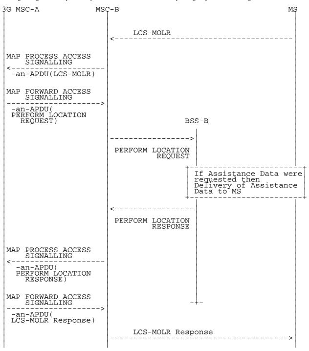
Figure 67c: Signalling for the request of Assistance Data or De-ciphering Keys
