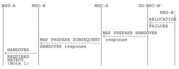
Figure 47: Signalling for Subsequent Inter-MSC Handover to third MSC (3G\_MSC-B') execution (Negative outcome)
