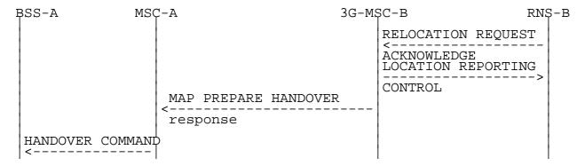
Figure 38: Signalling for Basic Inter-MSC Handover execution (Positive outcome)
