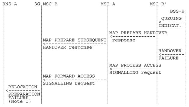
Figure 34: Signalling for Subsequent Inter-MSC Handover to third MSC (MSC-B') execution (Negative outcome)
