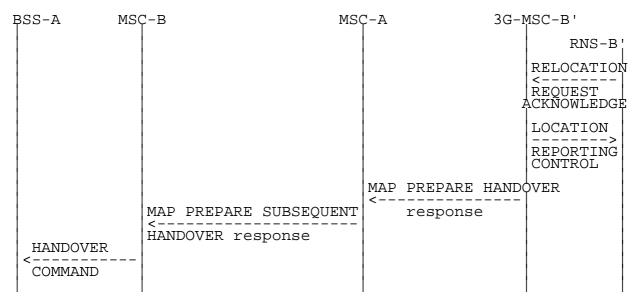
Figure 46: Signalling for Subsequent Inter-MSC Handover to third MSC (3G\_MSC-B') execution (Positive outcome)
