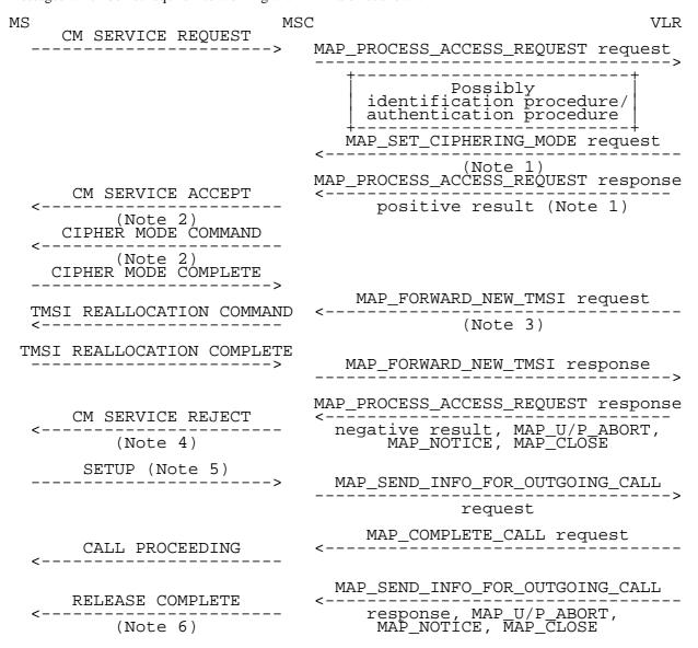
Figure 3: Part of outgoing call set-up sequence
