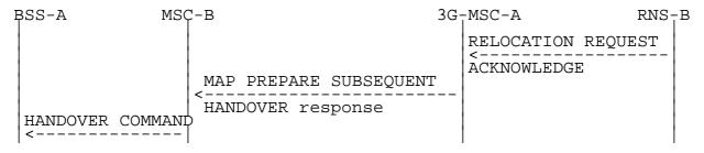
Figure 44: Signalling for Subsequent Inter-MSC Handover back to 3G\_MSC-A execution (Positive outcome)
