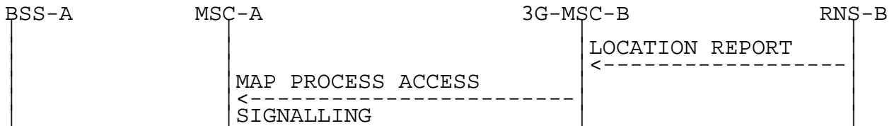
Figure 42a: Signalling for updating of anchor MSC after change of location in RNS
