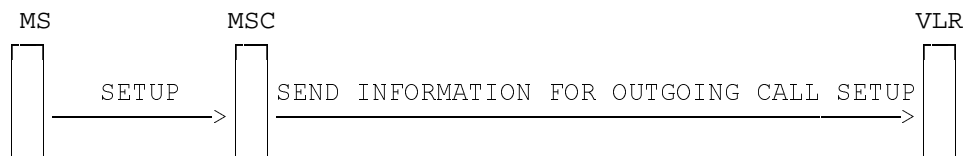
Figure 5.8: Signalling at explicit invocation of a CUG call
