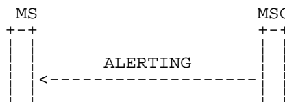
Figure 5.7: Signalling for notification of waiting call to calling subscriber
