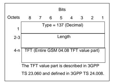
Figure 50: Traffic Flow Template Information Element
