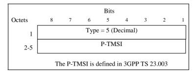
Figure 13: The Packet TMSI Information Element
