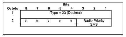
Figure 28: Radio Priority SMS Information Element
