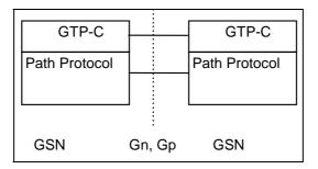
Figure 63: Signalling Plane - Protocol Stack
