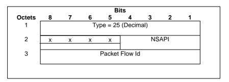
Figure 30: Packet Flow Id Information Element
