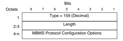
Figure 7.7.58.1: MBMS Protocol Configuration Options Information Element
