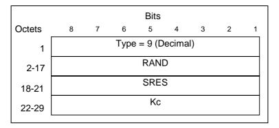
Figure 15: Authentication Triplet Information Element
