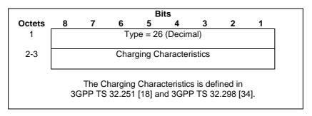
**Figure 31: Charging Characteristics Information Element**
