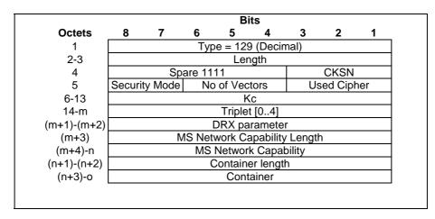
Figure 40: MM Context Information Element with GSM Key and Triplets
