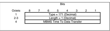
Figure 7.7.70.1: MBMS Time To Data Transfer Information Element
