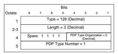
Figure 38: End User Address Information Element for PPP
