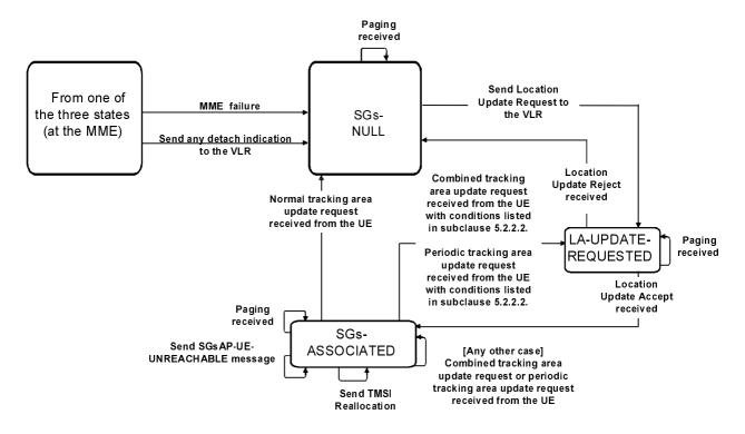
NOTE: A normal attach request or attach request for emergency bearer services causes the same state transition as a normal tracking area update request.
