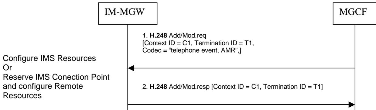
**Figure 49: Activation of processing of DTMF digits received in RTP for sending the digits inband to CS CN (message sequence chart)**
