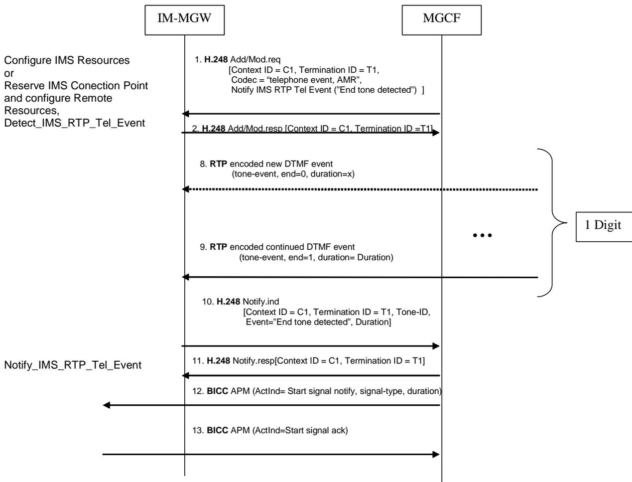
**Figure 48: Activation of notification of DTMF digits received in RTP and examples of sending the digits out-of-band to CS CN, a whole digit received by IM-MGW before sending further (message sequence chart)**
