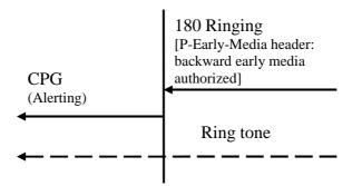
Figure 18a: Sending of CPG(Alerting) (Receipt of 180 Ringing response with authorization of early media)
