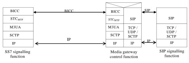
Figure 27: Control Plane interworking between CS networks supporting BICC over STC and M3UA and the IM CN subsystem
