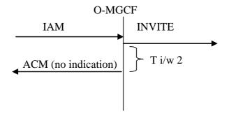
Figure 17: Sending of ACM (Ti/w<sub>2</sub> elapses)
