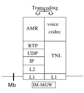
Figure 31/1: IM CN subsystem to bearer independent CS network user plane protocol stack
