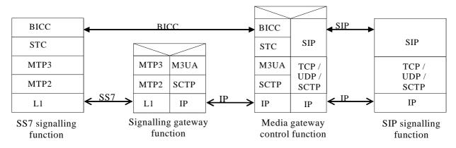
Figure 25: Control Plane interworking between CS networks supporting BICC over MTP3 and the IM CN subsystem
