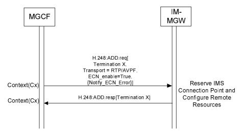
Figure 9.2.11.2.1: Procedure to Request ECN
