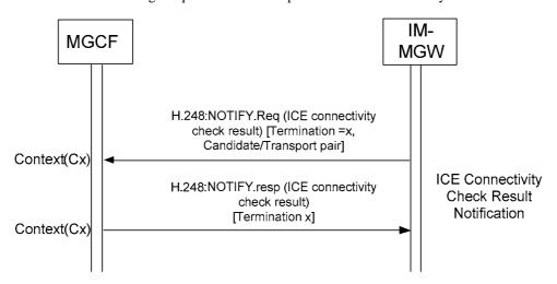
Figure 9.2.12.4.3.1: Procedure to report ICE connectivity check result
