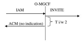
Figure 17: Sending of ACM (Ti/w2 elapses)
