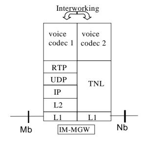
Figure 31/1: IM CN subsystem to bearer independent CS network user plane protocol stack
