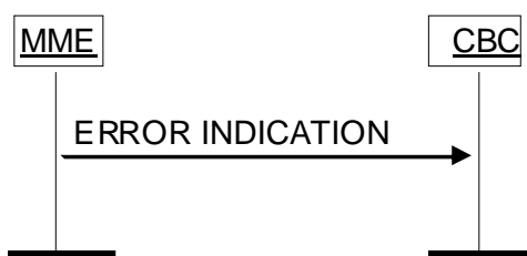
Figure 4.3.3B.2-2: Error Indication procedure, MME originated. Successful operation.
