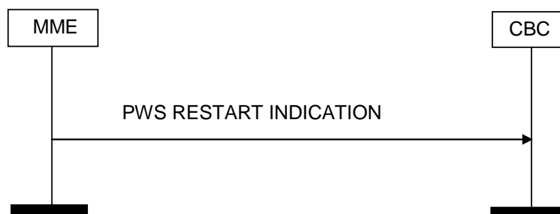
Figure 4.3.3E.2-1: PWS Restart Indication, Successful Operation.
