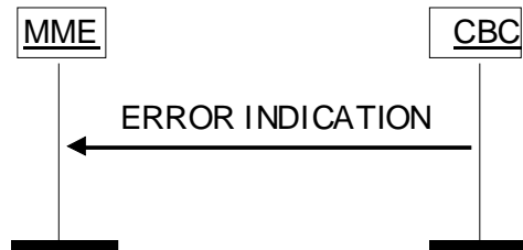
Figure 4.3.3B.2-1: Error Indication procedure, CBC originated. Successful operation.
