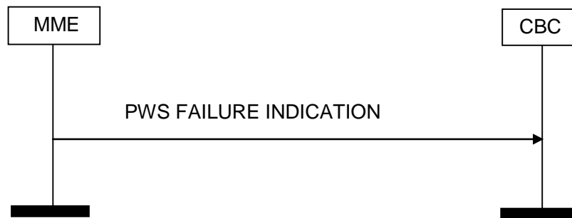
Figure 4.3.3F.2-1: PWS Failure Indication, Successful Operation.
