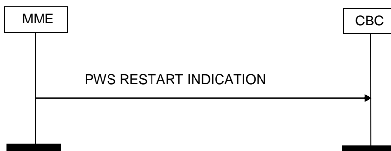
Figure 4.3.3E.2-1: PWS Restart Indication, Successful Operation.
