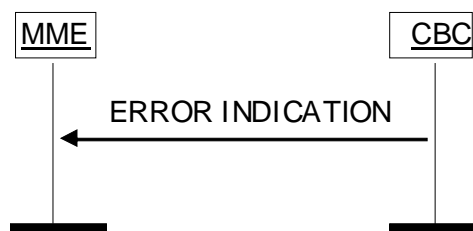
Figure 4.3.3B.2-1: Error Indication procedure, CBC originated. Successful operation.
