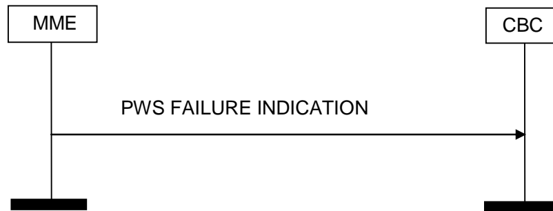
Figure 4.3.3F.2-1: PWS Failure Indication, Successful Operation.
