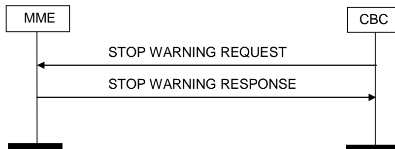
Figure 4.3.3A.3-1: Stop Warning procedure, Unsuccessful operation.
