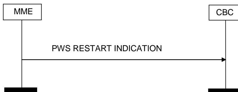
Figure 4.3.3E.2-1: PWS Restart Indication, Successful Operation.
