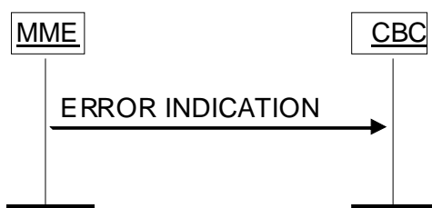
Figure 4.3.3B.2-2: Error Indication procedure, MME originated. Successful operation.
