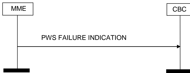
Figure 4.3.3F.2-1: PWS Failure Indication, Successful Operation.
