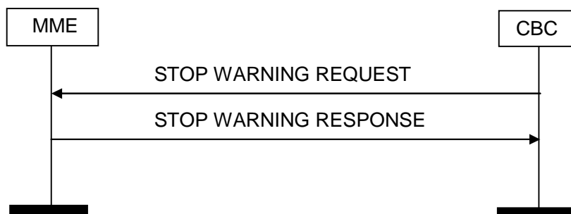
Figure 4.3.3A.3-1: Stop Warning procedure, Unsuccessful operation.
