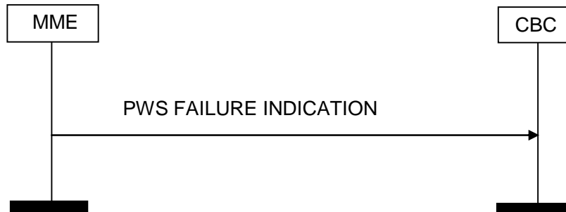
Figure 4.3.3F.2-1: PWS Failure Indication, Successful Operation.
