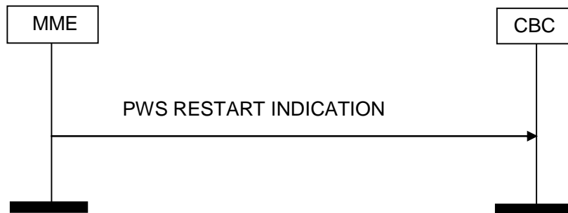
Figure 4.3.3E.2-1: PWS Restart Indication, Successful Operation.
