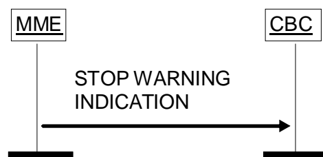
Figure 4.3.3D.2-1: Stop Warning Indication procedure, MME originated. Successful operation.
