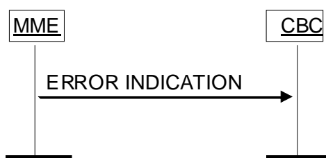
Figure 4.3.3B.2-2: Error Indication procedure, MME originated. Successful operation.
