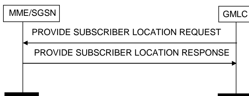
Figure 6.2.2-1: Provide Subscriber Location procedure. Successful operation.
