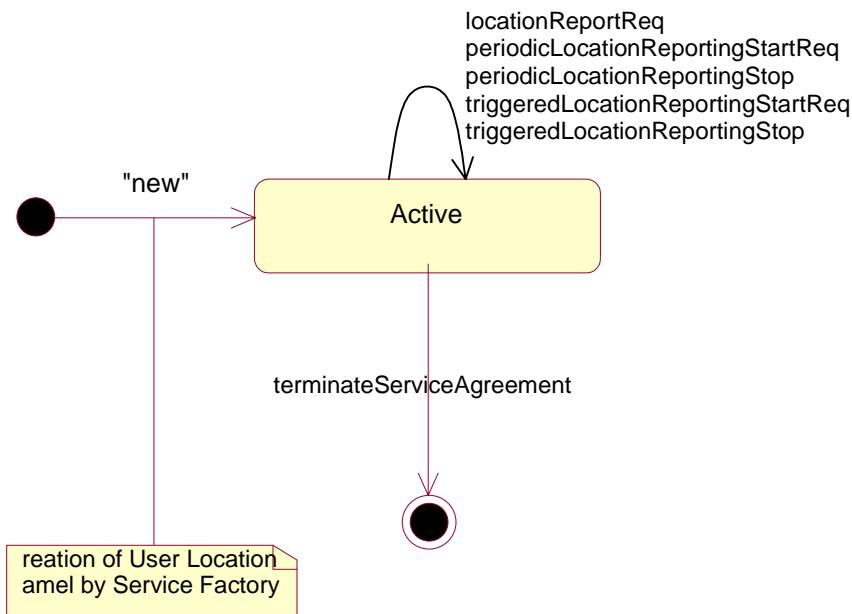
**Figure 7-17: State Transition Diagram for Network User Location**
