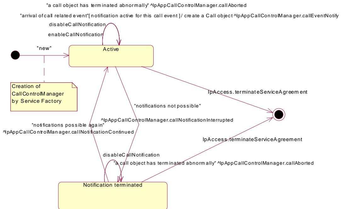
**Figure 7-11: State Transition Diagram for the CallControlManager**
