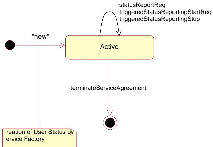
**Figure 7-18: State Transition Diagram for User Status.**
