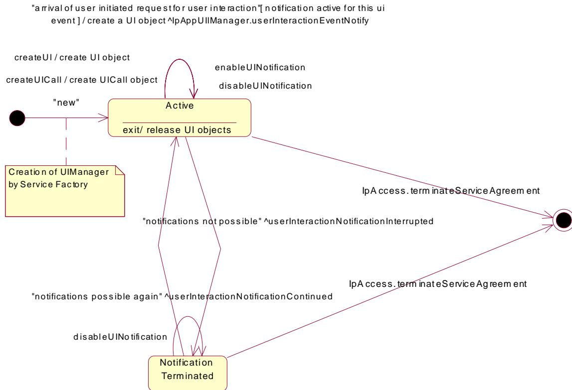
**Figure 7-13: State Transition Diagram for the UIManager**
