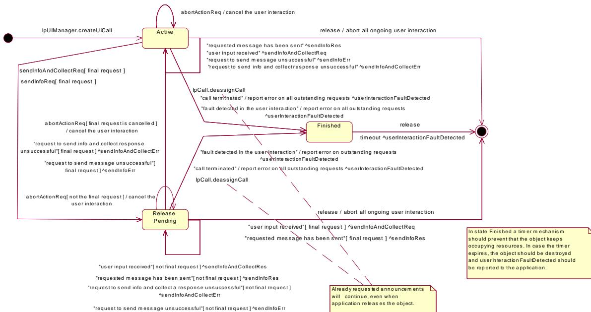
Figure 7-15: State Transition Diagram for UI Call
