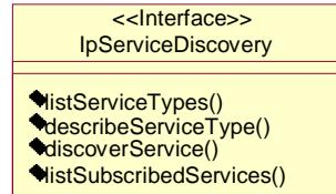
**Figure 6-4: Service Discovery Class Diagrams**
