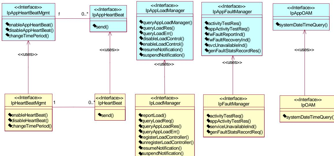
**Figure 6-6: Integrity Management – Application and Framework Class Diagrams**
