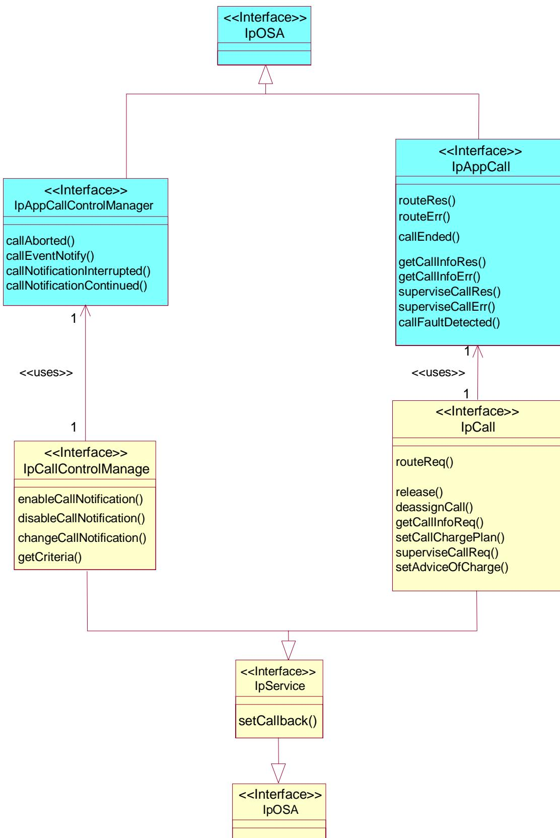
Figure 6-10: Generic Call Control Class diagram Interface Classes
