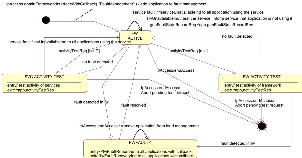
**Figure 7-6: State Transition Diagram for Fault Manager**
