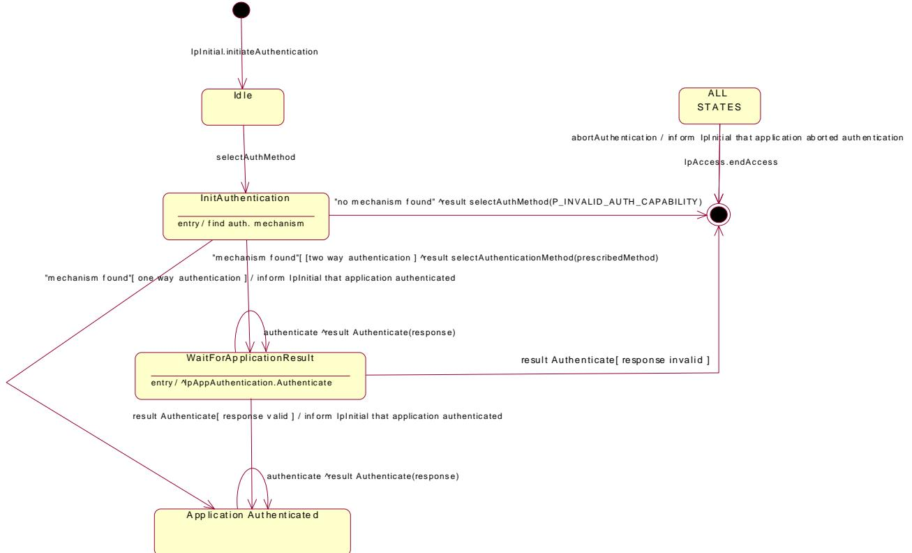
**Figure 7-1: State Transition Diagram for Authentication**
