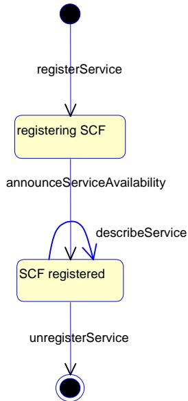
**Figure 7-10: State Transition Diagram for Service Registration**
