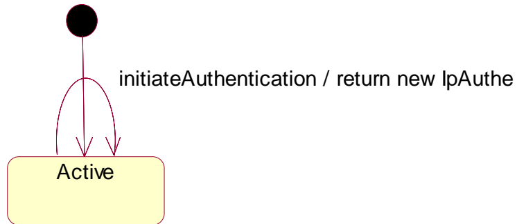
Figure : State Transition Diagram for IpInitial
