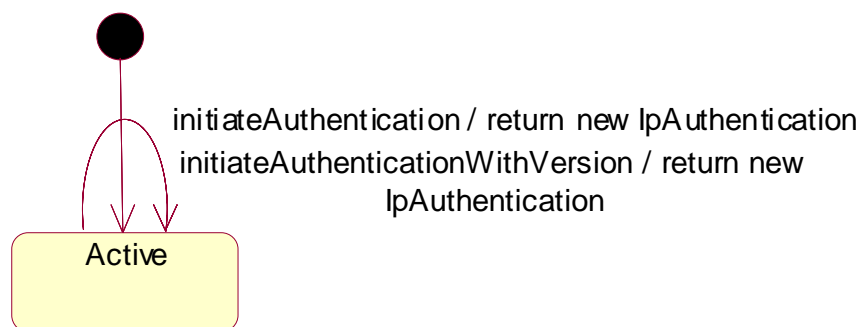
Figure : State Transition Diagram for IpInitial
