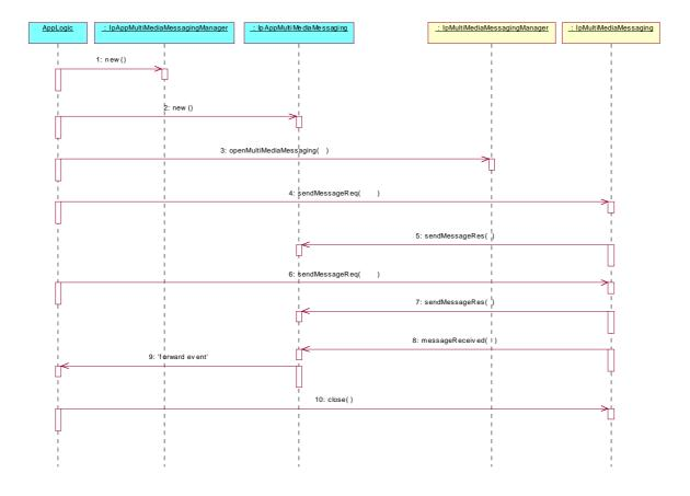
3: Request the opening of a MultiMedia Messaging object. The application intends to use this object to send messages to the same destination, so it has specified the defaultdestinationAddressList. The defaultSourceAddress is also specified.
