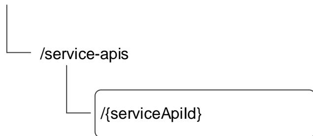
**Figure 8.10.2.1-1: Resource URI structure of the CAPIF\_Routing\_Info\_API**
