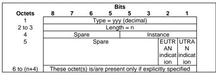
Figure 8.116-1: WLAN Offloadability Indication
