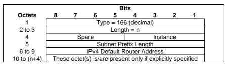
Figure 8. 97-1: IPv4 Configuration Parameters (IP4CP)
